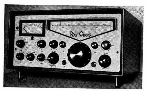
THE RCX505 IS THE FIRST AVAILABLE BRITISH DESIGNED RECEIVER TO EMPLOY A BALANCED MIXER SYSTEM WITH NO RF STAGE, TO GIVE EXCELLENT PROTECTION AGAINST CROSS MODULATION
