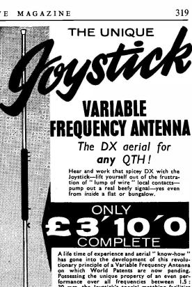
Possessing the unique property of an even performance over all frequencies between 1.5: 30 mcs. the Joystick's special matching facilities and associated A.T.U. ensures efficiency on any frequency. Peak performance for transmission and maximum voltage for reception—the Joystick is a major break-through for ardent SWLs and all licensed stations. Over 1,000 stations all over the world are already equipped with the Joystick—Testimonials pour in, e.g.— SIZE 7'6".
