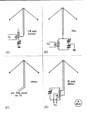
Fig. 2. In (a) it is shown that by strapping the feeders and series-tuning the whole system against ground, operation on both LF bands can be obtained. The other sketches show the Tx-end arrangements for working the HF bands. The only requirement at the station end is a versatile ATU.
