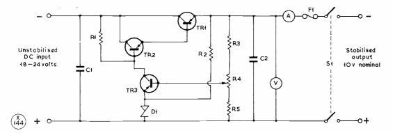
Fig. 9. Simple circuit for a stabilised power supply, using a zener diode at D1. The circuit will hold to a nominal voltage output, set hy R4, over builte a wide range of DC input. Meters as shown should be incorporated in the construction, and the pack should be correctly fused.
