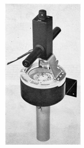
The "Sailor Navigator" can also be mounted on a hand bearing illuminated compass, for direct readings from beacon stations, with correction for variation and local electrical or magnetic deviation. The compass is dead-beat in action and will give readings to within one degree.
