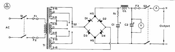
Fig. 6. The circuit for a variable low-voltage general-purpose power supply, for which suitable diodes are suggested in Table II. In construction, heat sinks should be provided at the points HS if heavy currents are to be drawn — see Table II. The smoothing choke Ch. should be chosen to pass the maximum load current without saturating, and should have as low a DC resistance and as high an inductance as possible.
