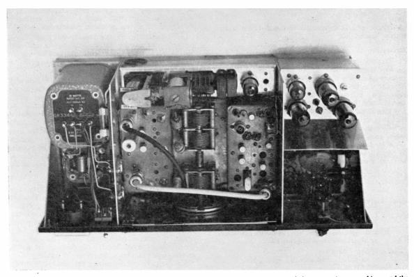
Plan view of the over-chassis layout of the VHF transceiver. The two-metre receiver converter is in a separate screened box, and the whole of the construction is in unit form.
