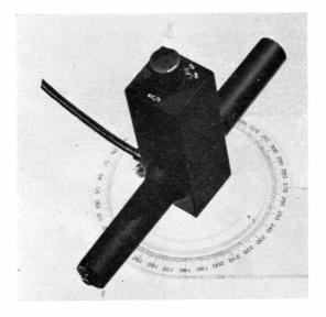
The neat D/F unit to work with the "Sailor 16T" marine receiver. It is a ferrite-rod aerial with a tuned circuit covering the beacon range 275-425 kc (the navigation waveband) and is mounted to rotate on a compass rose having a long ruler arm. This can be set up on the chart, and bearings laid off to get a fix.
