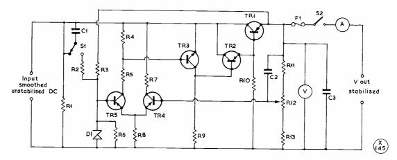
Fig. 10. A stabilised power supply, with overload protection, and designed for either of three possible output voltages — 6v. negative from 14-20v. input; -10v. from 24-30v.; and -20v. from 30-40v. DC input. Table III shows the resistor values to use for either of these three ranges, and the design allows for load currents up to 2 amps. R12 sets the output voltage and, as in Fig. 9, an ammeter and voltmeter should be provided.
