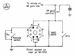
Circuit for the modification to the Hallicrafters SX-100, to enable it to be used for monitoring the radiated signal. The resistor Rx is selected to choice — see text. R60, of 330K, is as in the original, as are the RF gain and S7A, both panel controls. This modification should not be attempted without reference to the SX-100 manual.
