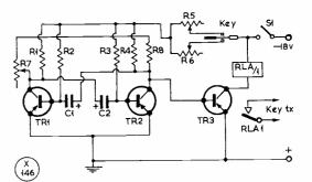
Circuit for the electronic (automatic) key for CW transmission, described by G3LRO. The secret of success with any sort of el-bug is correct adjustment of the dot-dash ratio. A certain amount of practice, with an audio oscillator, is also very advisable before attempting operation on the air, as the action is quite different from that of a straight, or pump-handle, Morse key.
