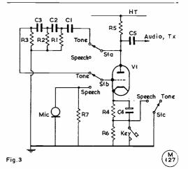
These circuits are self-explanatory when read with the text. Fig. 3 shows the finalised arrangement, where the first-stage valve functions either as tone modulator or speech amplifier values are given in the table opposite.
