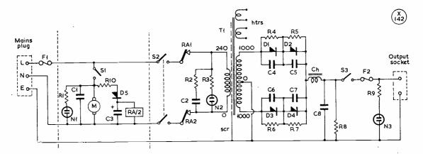
Fig. 7. Circuit design for a transmitter HT power pack, giving 650v. at 500 mA and incorporating suitable suppression where a blower motor is involved for forced-air cooling of the PA; this part of the circuit is between the dotted lines. The design considerations are discussed in the text and all values are given in the table. There are a number of silicon diodes suitable for a power pack of this sort. On no account should R8 be omitted, as it bleeds the pack when the mains are switched off.
