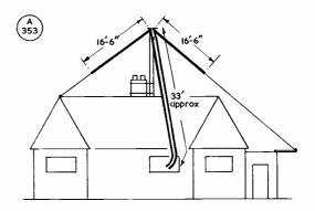
Fig. 1. General layout arrangement of the inverted-V system discussed by G6QB in his article. In sui'able locations, the arm-lengths could be doubled and a higher roof-mast used. The feeder-terminating configurations for six-band working are shown in Fig. 2.
