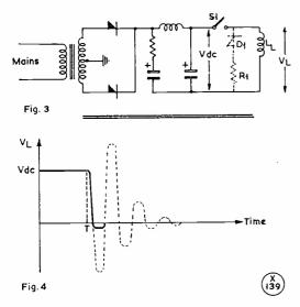
Fig. 3. Protection in the case of inductive loads — see text. Fig. 4. The appearance of an inductive-load transient when S1 is opened at time T; the dotted line shows how the transient behaves without the D1, R1 of Fig. 3.
