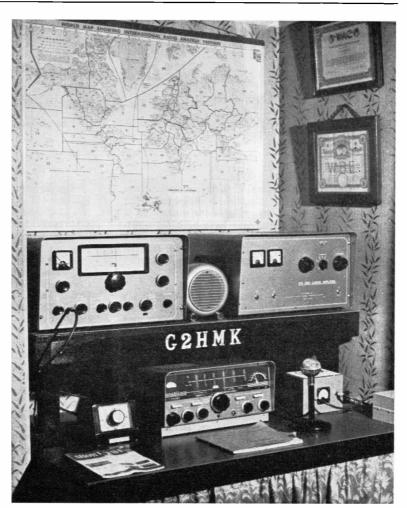
installation, and likewise is for SSB working only. It consists of an AR88D receiver and the transmitter is a home-constructed G5BJ-type crystal filter exciter into a 6AG7 buffer driving a TT21 linear running about 50 watts; this in turn pushes an 813 linear PA to full p.e.p. on 20 and 80 metres. The aerials used, for either station, are an 80-metre dipole and  $a_{1}^{A}$ . Mosley TA-33JR. beam.
