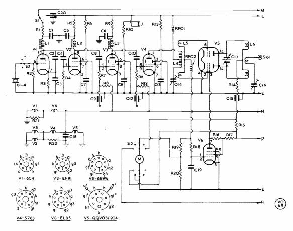
Fig. 6. Circuit of the transmitter section of the G3OCB two-metre transceiver, which is built as a separate and self-contained unit. Conventional circuitry is used and all values are given in the table herewith. Like other parts of this design, the circuit as shown here could be adopted for a low-power fixed-station transmitter, running about 20 watts input, with a conventional modulator.
