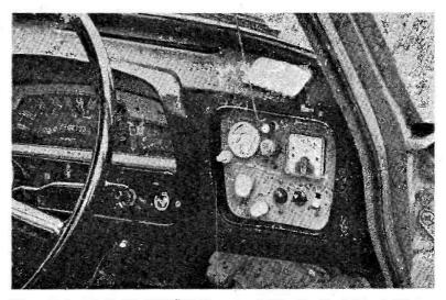
The control panel for the G3MCG/M two-metre mobile rig. The left-hand dial is a repeater for the tuning of the remote Rx in the boot, the motor control being for both speed and direction. The meter (right) functions as an S-meter and an RF output indicator. The panel is about  $4\frac{1}{2}$  ins. square and quite shallow. A 12-core cable connects it to the Tx/Rx and PSU at the rear. A G3GMN primt
