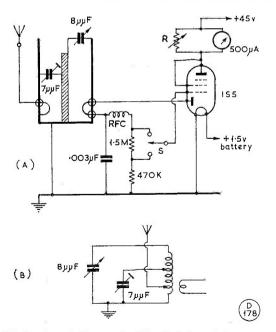
Fig. 1. At (A) is the circuit of the BC-906D, which is in the category of a secondary frequency standard for the range 144-240 mc. Sketch (B) is the equivalent circuit of the resonant cavity.
