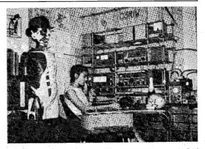
Station G3RIW is owned and operated by Miss Beatrice Whitaker, 51 Chevening Road, London, N.W.6. Her equipment includes a KW-77 Rx and transmitters for all-band coverage. Note how the frame-work for carrying the gear is built up by use of adjustable tubular fittings. It should be explained, that, as well as Amateur Radio, G3RIW is actively interested in human physiology, the keeping of lizzafes, and breeding a particular species of beetle. She refuses to explain the significance of the skull!
