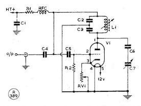
Fig. 2. Q-multiplier arrangement used by GW8PG for his TCS receiver — and see Fig. 1 for inter-connection. C7 is the peaking condenser. The selectivity of the receiver is considerably improved by incorporation of this unit.
