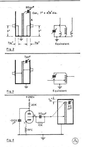
stability. Tapping the grid leak down the inner conductor will also improve the stability. The cathode choke RFC can be the ground lead or else about five turns close wound to  $\frac{1}{2}$  in. diameter.
