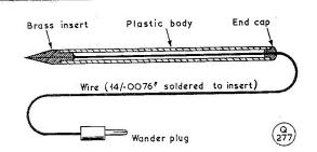
The sketch shows a cross-section of the assembly. A test lead of this nature should fill the needs of those in a similar predicament, and would also serve those who have constructed test meters described in this *Magazine*—all of which articles never mention a test prod !
