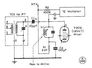
Fig. 1. The IF circuit modifications for the TCS receiver, discussed by GW8PG in the text. Cl is for bandwidth control.
