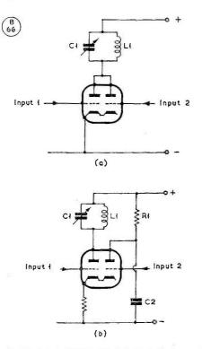
Fig. 3. Double-triode mixers are suitable both for receiver work or for the early stages of transmitters. At (A) the and is are paralleled and the combined frequency selected by the tank circuit L1, C1; at (B) the second anode is held at earth potential (RF) by C2, so that the second half of the triode runs as a cathode follower, with a common cathode load.
