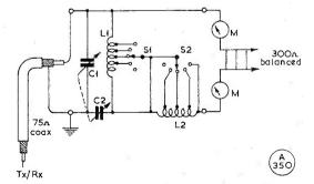
Fig. 2. A multi-band adjustable balun for the HF ranges, which can be used either way round. Values are given in the text, opposite.
