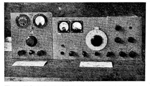
This was one of the home-constructor items in the Cornish Radio & Television Club's exhibition at Penzance on June 15. Built by G3OCB of Truro, it is a 10-160m. SSB exciter giving 40w. p.e.p. with, at left, a two-metre PA operated on the transverter principle, through an oscillator-mixer unit.
