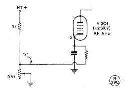
Fig. 3. Separating the RF and IF gain controls on the TCS receiver. In the original, this is common to both, as in many surplus types. The modification is explained in the text, and values here are 220K for R1, and 20K for RV1.
