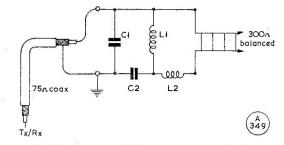
Fig. 1. Circuit for a single-band matching unit for 75 ohms into 300 ohms, transmission or reception. Values for each band are given in the table below.
