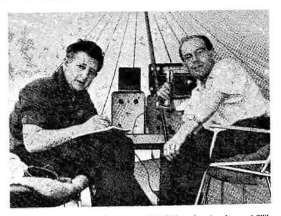
The operating position, PX1OX, Andorra, with DL2AG on the microphone and SWL Brian Balchin logging. The gear, fitted up in their living-tent, consisted of a K.W. Viceroy and a Drake 2B receiver. Except for some trouble due to power supply variation, which caused a 500-cycle drift on the Tx, it all performed faultlessly. The band mainly used was 20 metres, in the SSB mode. In a total operating time of 49 hours, 720 contacts were made in 64 countries and 171 of the QSO's were with U.K. stations.
