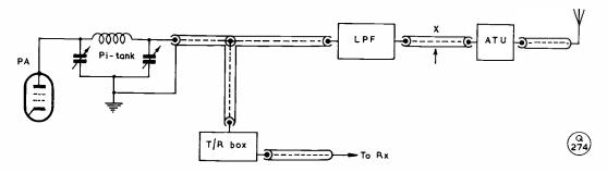
Fig. 4. Connecting in the T/R Box, or send-receive switch, where the transmitter output is at low impedance. The system functions by reason of sufficient voltage being derived from the transmission line to actuate a circuit — as in Figs. 1, 2, 3 and 5 — which blocks off the receiver when the transmitter comes up. The considerations in regard to getting full receiver protection are discussed in the text, and methods of making the Tee-junction required are shown in the drawings in Fig. 6 overleaf.
