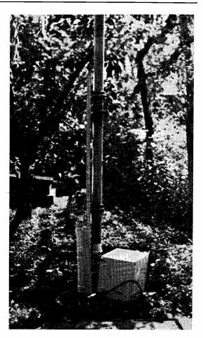
Base arrangement for the G6AS vertical radiator, showing the mounting sketched in Fig. 3. The switched ATU, for pre-set coverage of the three bands 3.8, 7 and 14 mc, is in the earthed bax.
