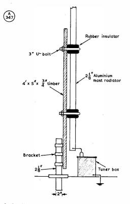
Fig. 3. Details of the base mounting in the G6AS design for a vertical mast radiator. The ATU (see Figs. 1 and 2) is in the (biscuit) box. By using rubber rings and timber as the intermediate support, adequate base insulation is obtained.
