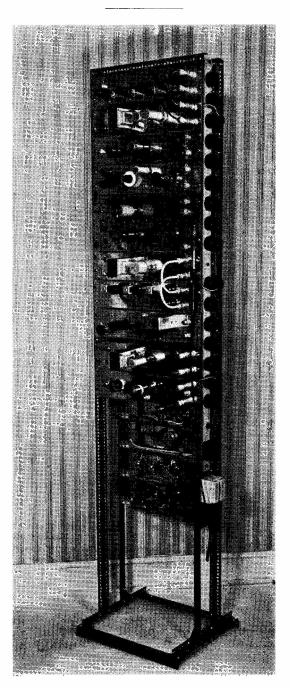
General appearance of the rack-panel layout used by G3KAB for the unit construction of equipment. Dexion angle forms the main frame and in his case the spacing between uprights accommodates a panel 14 in. wide. The height is 5 ft. Dimensions may, of course, be varied to sult individual requirements, remembering always to provide sufficient hase area for stability.
