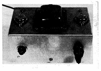
One way of constructing the transistor power supply unit discussed in the article by G3MY. Mounting the OC28's in the manner shown here ensures adequate heat-sinking, some points about which are brought out in the text. The transformer is a standard item as used for a 12v, vibrator HT circuit, and the final output is about 300v. at 100 mA, very suitable for mobile equipment.
