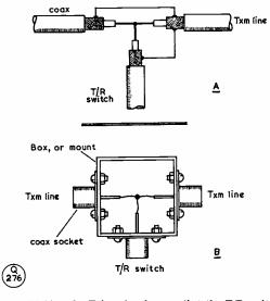
Fig. 6. Making the T-junction for coupling the T/R switch. At (A) is a neat way of doing it, requiring only a sharp knife, a pair of sidecutters and a small soldering iron. Sketch (B) shows how coax sockets can be mounted to make the interconnection pluggable.
