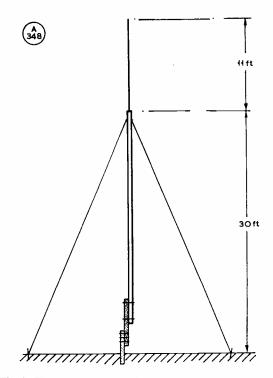
Fig. 4. The general layout, to give 41 ft. of height for the threeband vertical system at G6AS. Three guys are used, of plastic clothes-line, with a 15 ft. spread relative to the mast. A good earth mat is essential to get the best out of the system — see text for discussion.
