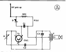
Circuit of the self-powered device for monitoring a CW signal. The RF picked up is rectified and used to power the transistor, connected as an audio oscillator. The resistor R gives some control of pitch.
