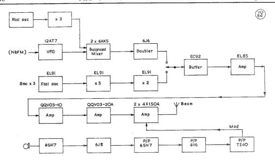
Fig. 1. Block schematic of the full-power AM two-metre layout in use at G3NPF (Southend-on-Sea), using a pair of 4X150A's in the PA, modulated by TZ40's. The frequency generating sections give choice of either crystal or VFO drive, the latter being of the crystal-mixer type, with the variable element on a relatively low frequency. Both frequency generators give output at 144 mc. The EL85 is a low-level amplifier and the QQV03-20A ensures ample drive for the high-power PA.
