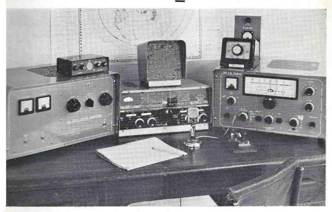
The KW Station comprising (left to right) KW 500 Linear Amplifier, Hammarlund HKIB Electronic Keyer, KW 77 Triple-Conversion Receiver and Speaker, Geloso Table mic., KW Viceroy transmitter, CDR Beam Control Unit, KW Match SWR indicator (Vibroplex bug-key and 'phones in desk drawer).
