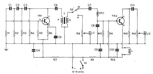
fed into any low-impedance audio amplifier, and J2 coupled into a receiver. The degree of coupling between the pick-up coil L and the GDO is a matter of experiment for the best results ("depth of modulation") and since J2 output is at low impedance, any coupling to this point can be through quite a long lead without appreciable loss. In practice, satisfactory operation with any normal type of amateurband GDO can be expected right up into the VHF region.
