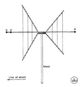
Fig. 2. Sketch to show side-view appearance of the G3NVA beam array consisting of a three-band two-element Quad with parasitic reflectors and directors. The assembly is mechanically in balance and the dimensions of the reflector and director elements are kept down by the use of traps—see Fig. 1, p. 121.
