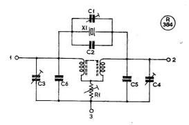
Fig. 2. Circuit of the R.206 filter discussed in the text. The nominal values are: CI, 30  $\mu\nu$ F; C2, 15  $\mu\mu$ F; C3, C4, 100  $\mu\mu$ F; C5, C6, 746  $\mu\mu$ F. R1 is explained in the text, and the crystal is a 465 kc bar.
