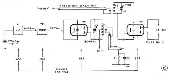
Fig. 2. Circuit arrangement suggested by G3BA for the conversion of an SCR-522 (BC-624 Tx) for Sideband operation on two metres. Apart from the modification, the essential requirement is an existing SSB exciter (such as the K.W. "Viceroy") capable of giving Sideband output on 14 mc, for mixing in the output stage V4. Various points about this arrangement are discussed in the text and only the necessary circuit modifications to the BC-624 are shown here.
