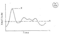
Fig. 1. Speech waveform showing a peak "P," which is what is indicated by the device shown in Fig. 2. At "A" is the average level, as measured by most monitoring devices. It is the peak voltages which cause over-modulation effects and splatter.
