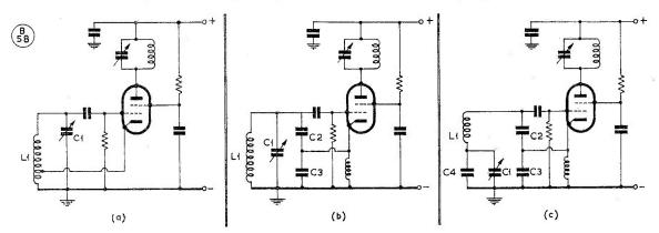
Fig. 1. Three basic circuits for a VFO, either for receiver or transmitter. In practice, most VFO's are elaborations or derivations of one of these. At (a) is the Electron-Coupled Hartley, at (b) the Colpitts, and at (c) the Series Colpitts, or Clapp. In each case, C1, L1, is the actual oscillatory circuit; in (b) and (c) the condensers C2 and C3 are relatively large, and serve as swamp capacities; and in (c) the condenser C4 is large compared with C1, and must be of good quality.
