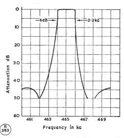
Fig. 1. Resonance curve of a typical R.206 filter unit. This is good enough for use in an SSB generator giving 40 dB unwanted sideband suppression—see Fig. 3.
