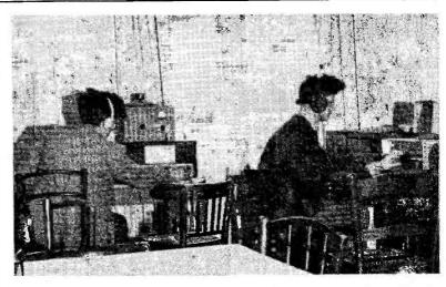
A general view of the HF and Top Band station at Douglas, I.o.M., signing GD6UW, with G3RSE at the 160m. rig on the left, and G3MZM operating on the HF bands, for which the gear consisted of a Hammarlund HX-50 CW/SSB transitter and KW-77 receiver. For 160m., the transmitter was a Labgear Topbander and the Rx an S.640.
