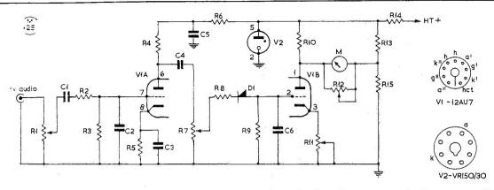
Fig. 2. Circuit of the Peak Audio Level Meter. A speech voltage input of about Iv. is taken off from some point in the speech-amplifier/modulator chain, and the action of the device is such that speech peaks only are indicated on the meter in the anode of VIB. VIA is a low-gain amplifier, DI rectifies the audio for charging C6, and VIB is in bridge with the meter. Circuit function is explained in the article and all values are given in the table.
