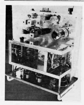
View above-chassis of the transmitter, showing the layout in the PA compartment. Expanded aluminium, covering top and side, is used to complete the screening. The neat arrangement of parts and the careful workmanship can be seen from this photograph.
