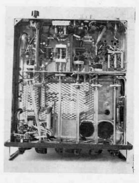
Under-chassis view of the G3NNK two-metre transmitter. The xtal holder is on the extreme right, with Swi immediately above it. The driver anode compartment is at extreme left; the twin-feeder from the coupling coil into the PA grid section runs along the side of the chassis. The gating valve V6 see Fig. 1, p.459— is at bottom left.
