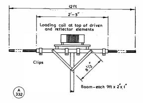
Fig. 2. Plan view of boom-ends and their supports in the G3KBE Mini-Quad design. Sections 1-in. cube are cut out of the top end of the booms so that they are flush with the 27-in. hardwood pieces. The canes are secured under the hardwood.
