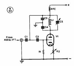
Fig. 1. The Q-Multiplier shown in basic form, for easy understanding of its operation. The oscillatory circuit (L1, C3, C4) is tuned by C5 to peak up the wanted signal. Feedback is controlled by the cathode potentiometer R2.
