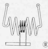
Fig. 3. Detail of the PA anode coil assembly; the coupling coil is made adjustable with respect to the tank, and is controlled from the rear of the PA compartment.
