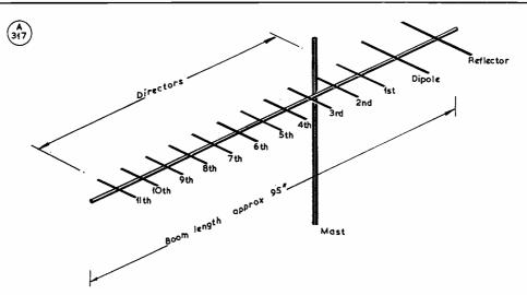
Fig. 1. To show the general appearance of a Long Yagi, with approximate layout dimensions, as described in the text. The exact positions of the directors are given in the tabulated data, and these must be adhered to for correct operation with maximum gain. Constructional methods and the feeding and tuning of the array are explained in the article.
