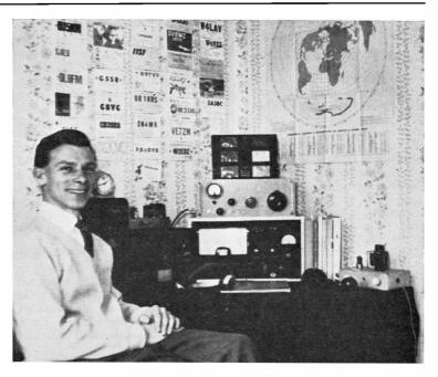
G3NRI is one of the Yorkshire stations, and runs a home-built Tx using a Geloso VFO driving a 6146 PA to about 45 watts, the receiver being an HRO. For the occasional phone QSO, cathode modulation is used, and the station equipment includes a dummyload and SWR indicator incorporated in the ATU, also a 100 kc CC oscillator for calibration. Activity is mainly CW on the 15-20-40 metre bands.
