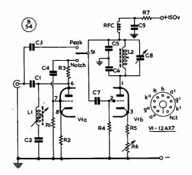
Fig. 2. The full circuit arrangement, for giving both "peak" and "notch"—see text. A double-triode is used, VIB for peaking and VIA for notching. Under certain conditions, the outer of the input coax socket should be earthed to the chassis of the unit; or it may be found preferable to leave the earthing to the Rx end.
