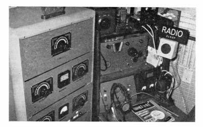
Neat station operated by Derek Morris, ZL4OP, 134 Stobo Street, Invercagill, New Zealand. His Tx is all-band with an 813 PA, modulated by a pair of 807's, and aerials are a ground-plane and an 80-metre Zepp. The main Rx is a BC-342, and the stand-by Tx an ARC-5. ZL4OP was licensed in 1957, comes from Lancing in Sussex, is active mainly on 20m. CW, 0300-1000 GMT, and has 62 countries confirmed. He has been out in N.2. since 1952.
