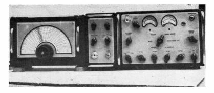
The complete two-metre layout as designed by G3NNK and described in the article. The units, left to right, are: VFO, with its scale drawn to give 10 kc reading-off points through the whole band; the Modulator, for either series-gate operation through the V6 stage in Fig. 1, or NBFM on the VFO; and the transmitter itself, which runs 90 watts on full CW input. All the constructional work was done with normal amateur-station facilities only.
