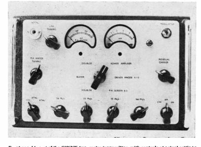
Front panel layout of the G3NNK two-metre transmitter, with controls at actual settings for operation. The right-hand meter is suitably switched for current readings at all necessary points, the other meter heing in the plate of the QQV06-40 PA stage. Main layout details are discussed in the text.
