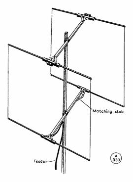
Fig. 3. Showing the general constructional layout for the Mini-Quad as described by G3KBE. The loading coils — see text and Fig. 2 — are carried on the upper length of each section. Dimensions, tuning and results are discussed in the article.
