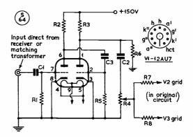
Fig. 1. The limiter stage, showing alterations to the first half of the circuit, and changes on the grid side of the tone amplifiers, V2, V3. The text and the circuitry here should be read with the original articles, by G3BST.
