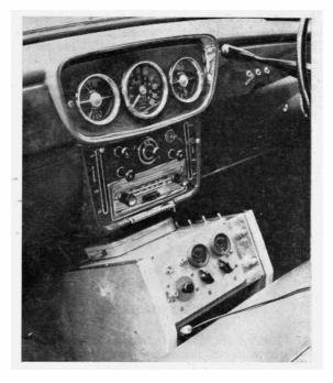
The G3OUQ/M installation, the transmitter and control panel being mounted in the console; the transistor Top Band converter -- to the circuit on p.188 of our June 1962 issue -- is in the slim box below the car radio. The complete wiring plan for the inter-connection of the various units of the equipment is given in the accompanying circuit diagram, on p.461. The car is a Singer "Gazelle," 5404-AC.
