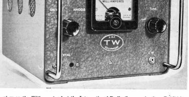
On view on the Withers stand at the International Radio Communications Exhibition — the TW VHF transmitter, a very neat little 10-watt CW/phone job which, in spite of its small size, is highly efficient. The PA is a QQV03-10 modulated by a pair of EL84's. The transmitter is available for either 2, 4 or 6 me tree (overseas).
