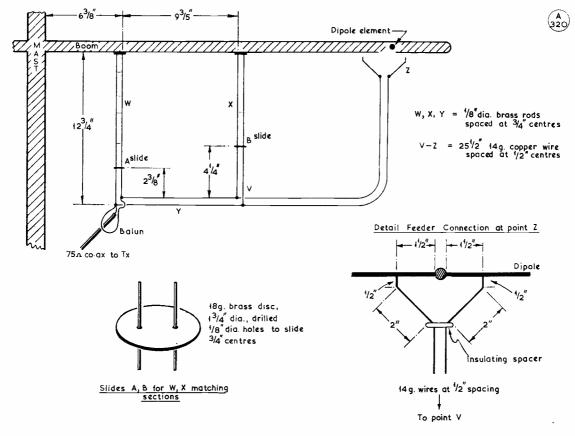
Fig. 3. Sketch to show the layout and dimensions of the matching arrangements for the Long Yagi designed by G3KPT. To feed from the transmitter by coax at 75 ohms, a 75-300 ohm balun is required, which is matched into the driven (dipole) element as shown here. The positions of slides A and B, which tune the stubs, may vary from those indicated, these being as obtaining at G3KPT.
