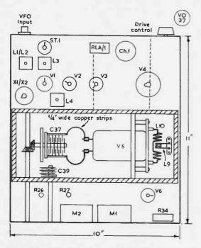
Fig. 2. The above-chassis layout of the G3NNK transmitter. The xtal mount is a ceramic octal v/holder using alternate sockets. The PA anode coil L11 and L12 — see Fig. 1 — have been omitted for clarity.
