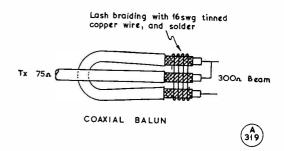
Fig. 2. Construction of the 75-300 ohm matching balun, feeding from the transmitter at 75 ohms — and see Fig. 3.
