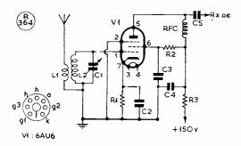
Circuit of the 20-metre preselector, which amounts to no more than a tuned RF stage, suitable for use with any receiver capable of giving the necessary HT/LT supplies. It is not recommended for a receiver that is already lively around 14 mc, as an RF amplifier of this sort will bring in a good deal of noise; on the other hand, it will improve the performance of a receiver which is sluggish at these frequencies. upon, the mobiles would find many more stations to work . . . and so it would go on.
