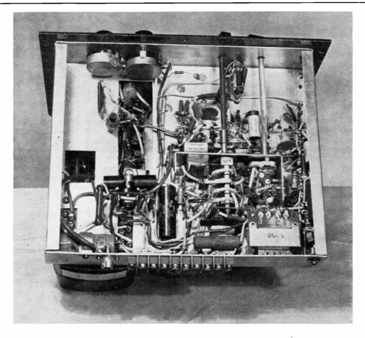
Underside view of the amateur-band receiver, showing the screened compartment for the product detector and BFO circuitry, using a 7360 in this position. Extension rods connect the function switch (SW3 in the main circuit) and the BFO control with their knobs on the front panel. The output transformer T2 can be seen in the lower right-hand corner of the chassis, and the pea-bulb serves as an HT fuse.
