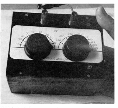
This device will give direct measurement of unknown capacities over the ranges shown, when used with any usual GDO — see circuit and discussion in text. It is easily calibrated from a few condensers of known value, and the readings obtained are entirely suitable for practical work.
