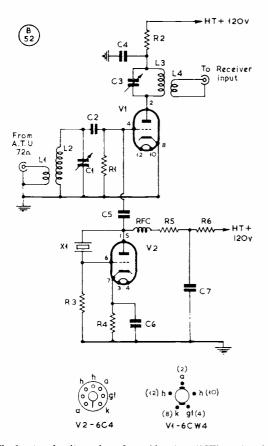
The front-end unit consists of a troide mixer (6CW4 nuvistor) with a triode crystal oscillator loosely coupled to its grid circuit. Cl/L2 is tuned to signal frequency, and C3/L3 to a frequency in the 1.5-2.0 mc area. The value of R5 is chosen to allow V2 to operate at the lowest voltage at which it will con-tinue to oscillate.
