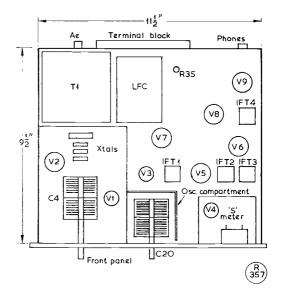
Fig. 3. Layout above chassis and arrangement of the main items in the G3BDQ receiver — compare with one of the photographs. This drawing is not to scale and is intended for suggestion only.
