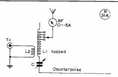
Showing the circuit arrangement discussed in the text. By using a counterpoise, radiating efficiency on 160 metres can often be considerably improved compared with a direct earth. In amateur practice, the counterpoise need not be directly underneath the aerial, nor must it be of the same electrical length. The coll size suggested, with the taps taken, will accommodate wide variations in aerial and counterpoise dimensions.
