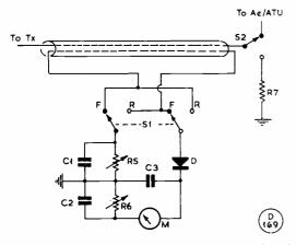
Fig. 3. The SWR device is the standard circuit adapted for the panel instrument in the Type 3 Visual Indicator. C1, C2, C3 are .001  $\mu$ F; R5 is a 200-ohm potentiometer for adjustment control; R6 is a 5K potentiometer for setting up (see text); and R7 is the non-inductive load resistor, which must be rated to the Tx input as it absorbs all the RF output in the test position for S2. Rectification for the meter is by the crystal diode D. See text for the text for further details.
