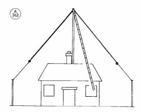
Fig. 2: A Vee-shaped aerial can be erected above the house or bungalow, using one roof mast. Lengths are discussed in the text, and two wires of 33 feet each will make a very useful threeband arrangement for 7, 14 and 21 mc.
