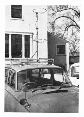
Nice gainy two-metre mobile array carried by G3BAK/M (Stockport), consisting of two halo's, stacked. As well as gain, such an arrangement would give a marked increase in directivity-which might be thought a disadvantage under mobile conditions.
