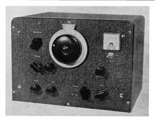
General appearance and front panel layout of the G3BDQ amateur-band receiver, which is a constructional design embodying modern circuitry and techniques. The block diagram at Fig. 1 shows the circuit sequence and by adopting unit construction a neat and space-saving layout is achieved.
