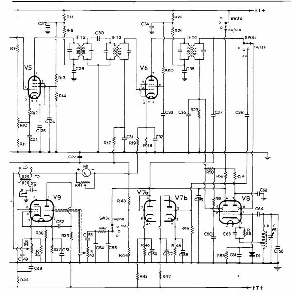
AR88 is prone to this fault. In most cases of cross-modulation the RF stage or stages are to blame. The hotter the RF stage the more likely it is that you will hear your local BC station beneath old local G9ZZ's emanations. The well known Racal receiver does not use an RF amplifier, and most amateurs would give a good deal to lay hands upon one of these fine pieces of commercial gear.
