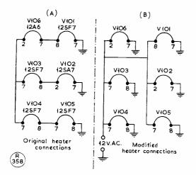
The heater modification to the ARB receiver, enabling it to be run from a 12v. AC supply. The ARB is a surplus-type 6-valve receiver having a good performance on the lower frequency amateur bands-1.8, 3.5 and 7 mc are covered.
