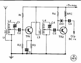
Circuit of the transistorised LF band converter, designed for covering the 160m, amateur band by tuning 200-230 metres on almost any BC receiver. This arrangement could be used with a standard car radio Rx, for mobile working on Top Band; with the oscillator on the high side of the signal, there is the slight disadvantage that the main receiver tunes "in reverse." All necessary details are given in the text. To avoid damage to the transistors, switch off on "transmit" and short the input.
