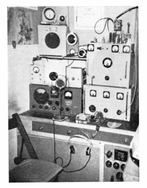
GaVZ is operated on two metres by J. Redrup, Lyndale, Longwick Road, Princes Risborough, Bucks. Very successful results have been obtained over a long period, using a 12-ele bi-directional stack and only 12w. input. This photograph shows, on the right, the transmitter, power supplies and modulator and, on the left, the 144 mc frequency meter and monitor, with 100/1000 kc crystal marker, and the SX-24 main receiver; the two-metre converter is an ECC84 cascode arrangement.
