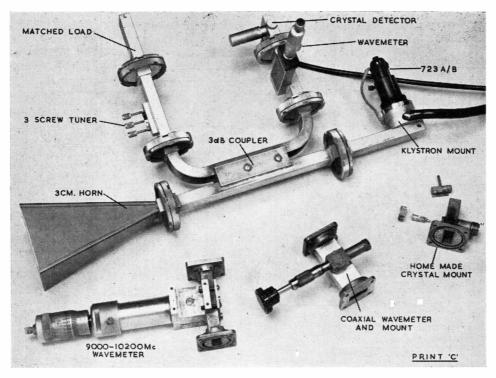
This photograph shows a number of the items used by G3BAK in connection with amateur microwave working; some can be home-constructed, and others are commercially available. As explained in the article, the secret of success is the 3 dB coupler or hybrid junction. Tuning can be done with ordinary BA-size screws fitted to the waveguide. Sizes for waveguides to operate on a wide range of amateur SHF bands are shown in Table I, on p.657 of the February issue.
