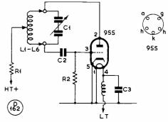
Circuit arrangement for the G73 modification suggested in the article. C1 is 5  $\mu\mu F$  per section; C2 is 50  $\mu\mu F$ ; C3 is .001  $\mu F$ ; R1 is 1000 ohms; and R2 is 10,000 ohms. The values for L1-L6 are given in the table alongside.
