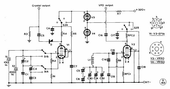
Fig. 1. Circuit of the instrument described in the article. The circuitry associated with V2 forms the stabilised variable frequency oscillator, the coverage of which can be calibrated to a high degree of accuracy — see text. V1 is a CCO with switched 100/1000 crystals for marking and checking the variable oscillator; it can also be used as a separate 100/1000 kc marker, giving band-edge and calibration beats into the receiver.
