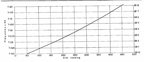
Fig. 3. The final calibration curve of the crystal-checked heterodyne frequency meter, as described in the article and shown in the photographs. From this basic curve, obtained from a specimen instrument constructed on the principles given in the text, graphs can be produced covering the higher frequency bands. Accuracy is limited only by the extent to which the crystal checker can itself be adjusted to zero-beat with some external frequency standard, such as WWV or MSF.
