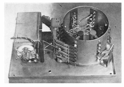
Illustrating the modification to the G73 Wavemeter, suggested by G3MFW and discussed in the text. It enables the G73 range to be extended to about 200 mc (1½ metres) and the instrument as modified can be used as a frequency meter or a VHF signal generator.
