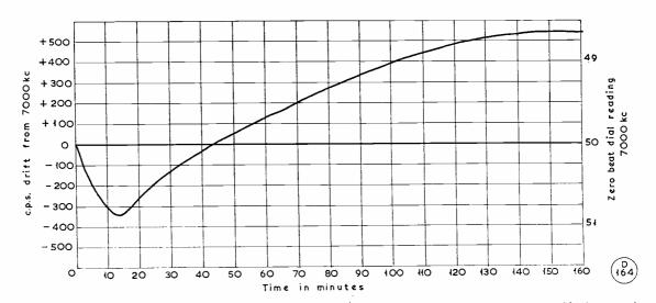
Fig. 2. The drift characteristic curve of the crystal-checked heterodyne frequency meter, in conditions as described in the text. As explained in the article, the shape of this curve can be varied according to the adjustment of the negative coefficient condenser. Where a long warm-up run is possible, it is sufficient to check the scale against the crystal standard as readings are taken.
