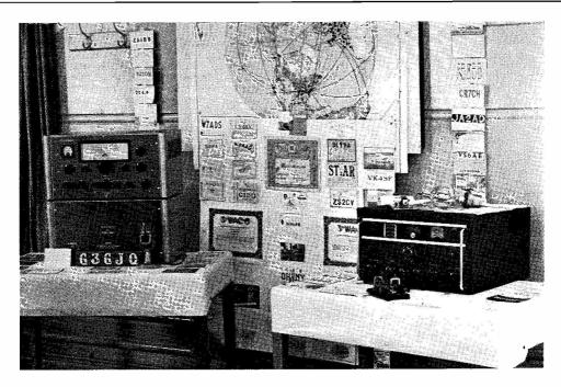
Gear arrangement by G3GJQ (ex-AP2R, YI2AM) at an exhibition at R.A.F. Swanton Morley, Norfolk, for a visit to the Unit by H.R.H. the Duke of Gloucester. The K.W. Viceroy (left), with its associated PSU and control unit, is operated on 15-20 metres, CW and SSB, into a Minibeam aerial, with an AR88 receiver. The fat bottle resting on the Rx is a 20-year-old 250TH, which comes in nicely for a 20-metre linear amplifier used with the Viceroy.
