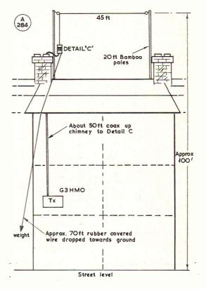
Fig. 1. General arrangement of the 160-metre transmitting aerial at G3HMO, London, S.W.1, of which full details are given in the text. The main feature of the design is that the RF appears at the highest point in the system.
