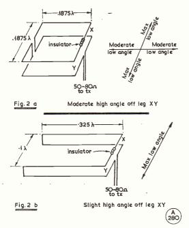
Fig. 2 (A) and (B) are further variations on the author's theme, which is to find a good indoor transmitting array for the 20-metre band. Fig. 2 (B) is tending to be large, requiring about 25 ft. on the maximum dimension, but would still be manageable, if the directions for which it can be placed in the roof-space are favourable.
