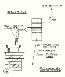
Fig. 2. Dimensions of loading and link-coupling coils, the feed to the system being by coax (down the chimney). It should be noted that the loading coil value is critical, to a turn or two, so that a tappable coil should be made up before finalising the coil assembly. There will be wide variations due to local site conditions.
