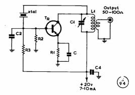
Fig. 1. A transistor crystal oscillator for about 27 mc, which will go off with an OC170 and an FT-241A type surplus crystal.
