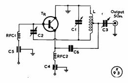
Fig. 2. Typical circuit for a 70 mc transistor oscillator, values for which are given in the text above.
