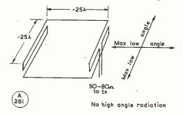
Fig. 3. Another variation, still taking low-impedance feed, in which a continuous length of wire is folded from the feed-point.
