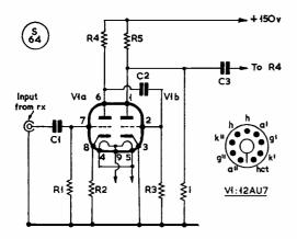
The circuit devised by G3NPF (2 Edith Road, Prittlewell, Southend-on-Sea, Essex) to replace the first stage in the G3BST circuit shown on p.12 in our March, 1960 issue. It ensures hum-free operation since the iron-cored component in the original is eliminated. Note: The resistor marked "1" is R6.
