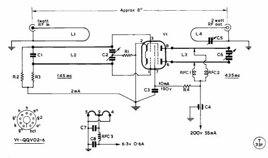
Layout for a 145-435 mc tripler circuit, using the QQVO2-6. For quite a low DC input, a useful level of RF output can be obtained if attention is paid to the various points about this circuit discussed in the text. It should be noted that the HT feed chokes RCF1 and RFC2 are tapped in at a voltage node on L3. Having obtained resonance, the final adjustments are for bias, and the positioning of L1 with respect to L2, and L3/4.
