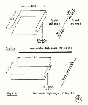
In Fig. 1 (A) and (B) are two practical indoor arrangements for 20 metres, requiring a maximum horizontal space of about 11ft. for Fig. 1 (A) the Reinartz Loop, and of 15 ft. or so in the case of Fig. 1 (B). These measurements allow the aerials roughly 3 ft. of clearance.
