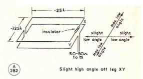
Fig. 4. The final version evolved by G3DIJ, with the results described in the text. It requires a maximum indoor dimension of about 20 feet, allowing for clearance.
