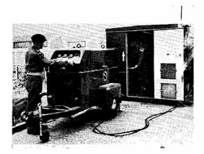
The power unit for the Racal transportable station, designed for field work with NATO Forces, is self-contained on its own towing trailer.
