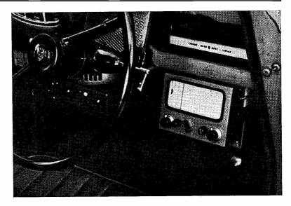
In the G3GMN/M installation, the receiver is carried in a shaped tray fitted as shown here. The control unit and 6-band transmitter (already described in previous issues) are visible at lower left of the wheel.
