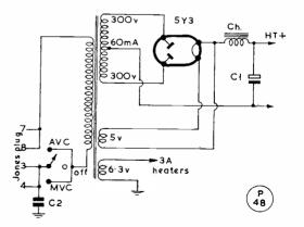
Circuit of a suitable AC power supply unit for the BC-348; it can be fitted on the dynamotor mounting, after removal of the machine. Values are: Cl, 16  $\mu$ F, 350v. working; C2, .01  $\mu$ F; Ch. 12-Hy, 100 mA; and T a 300v. transformer with suitable LT windings.
