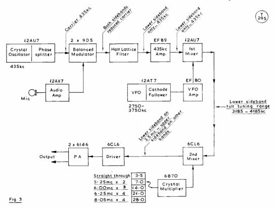
Fig. 3. Simplified block diagram of a filter-type SSB transmitter, based on the K.W. Viceroy. Other circuitry is included in the finished transmitter, but this diagram shows the essentials, together with the type of signal appearing at the output of each stage.
