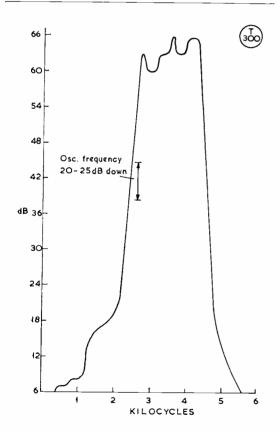
Fig. 5. The filter response curve, obtained by using a BC-221 as an RF generator and a carefully adjusted S-meter on the station Rx at G3BDQ. The filter band-width is adequate for amateur phone working and it has a good cut-off characteristic. For USB generation, the carrier oscillator should be positioned as shown, about 20 dB down the LF slope. Exact carrier placing is achieved by pulling the oscillator frequency slightly with a small air-trimmer C62—see Fig. 2.
