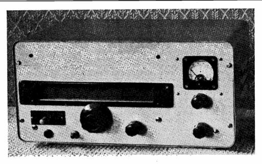
General view of the 20-metre SSB Transceiver, which is housed in a wrap-round style cabinet. The controls, from left to right, are: Send-receive keyswitch and phone jack, calibrator push-button, main tuning, RF gain and PA tuning controls, the upper of these two being the PA tank condenser C73 and the lower the grid condenser C72 (see Fig. 2). The dial mechanism is the Eddystone type 898, with a home-made escutcheon.
