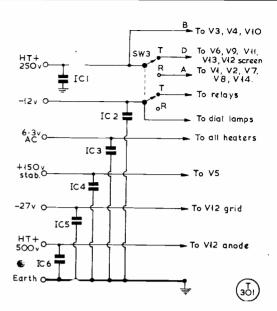
Fig. 6. A GPO type key-switch is used for SW3, the transmit-receive selector switch on the front panel — see photograph. SW3 switches HT to the appropriate sections of the equipment and also operates the IF and aerial relays. IC1-IC5 are .01  $\mu\mathrm{F}$  disc ceramics at the input sockets; IC6 is a .0018  $\mu\mathrm{F}$  disc ceramic rated at 1,200v. The negative 27v. blas for the PA is obtained from three 9v. dry batteries.
