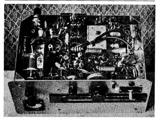
Underside view of the SSB Transceiver designed and built by G3BDQ.
