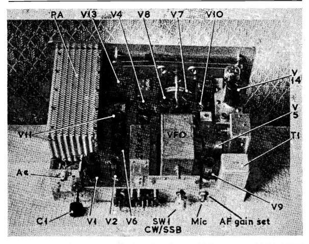
Rear view of the 20-metre SSB Transceiver out of its cabinet, with main items identified. The aerial relay is between the PA box and C1, and to the left of the VFO box are the IF stages and IF relay. The balanced modulator box and the crystal calibrator unit are behind the transformer T1; the 100 kc (calibrator) crystal is hidden by V14.
