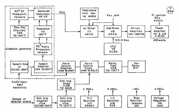
Fig. 4. General arrangement of the Hallicrafters HT-37 all-band SSB transmitter, and including all relevant circuitry. It will be noticed that in this design, carrier generation is at 9 mc with the VFO swinging across 5.0 to 5.5 mc. As in the K.W. Viceroy, the PA takes a pair of 6146's, and in both the output circuit is designed for a low-impedance load.
