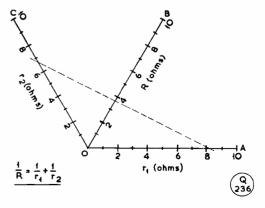
An abac for resistor calculations, where resistances are to be put in parallel to produce a required value. This diagram is drawn in such a way that it can be used as given here, with reasonable accuracy for practical purposes.
