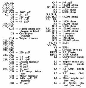
Note: With the exception of C3, C37, C43, C44, R19, L6 and L7, the original component reference numbers have been used. Where the components in the actual Unit are marked, the reference numbers will be prefixed with figure 3, e.g., C22 will be marked 3C22. C2, C45 may be omitted in some Units and C32, C42 may be of values different from those shown above.
