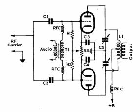
Fig. 1. A push-pull balanced modulator circuit. RF is introduced to both grids in parallel, audio in push-pull. The push-pull output circuit suppresses the carrier, leaving the two groups of sideband frequencies. C5 is tuned to the RF input, and R3 adjusted to give minimum carrier at the output terminals.
