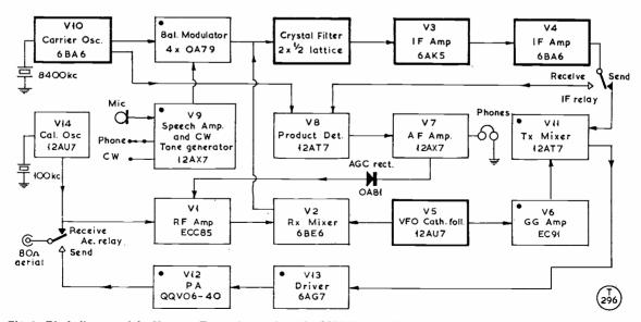
Fig. 1. Block diagram of the 20-metre Transceiver designed by G3BDO, and fully described in the article. The units in heavy line are common to both "transmit" and "receive" positions, and those with a dot in the top left-hand corner operate when transmitting. V1, V2, V7, V8 and V14 are only in use when receiving. The send-receive switch, SW3 in Fig. 6, is not shown on this diagram.
