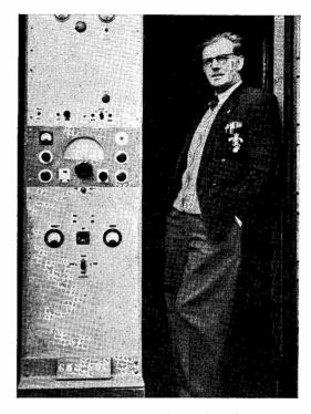
GM3GOC, Whithorn, Wigtownshire, author of the accompanying article—and also of that on the receiving SSB Adaptor in our November issue—has the tuner described here mounted in the upper chassis of the rack, which comprises a complete Tx/Rx assembly for SSB operation on 80 metres. The SSB Adaptor is fitted just above the receiver, occupying the central panel.
