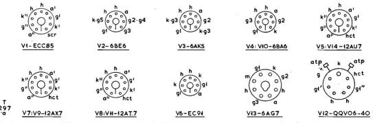
Fig. 2A. Base connections for all the valves used in the G3BDQ 20-metre SSB Transceiver. (Note: In the V12 diagram, the grid connection at upper left should be marked G2, for screen).
