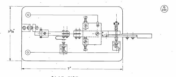
Fig. 2. Plan view of the semi-automatic key, showing arrangement of the parts. The dot-sender is carried on the vibrating arm, the period of vibration and hence the speed of the dots being controlled by adjustment of the sliding weight and the position of the end stop. The dash contacts are at the paddle end.
