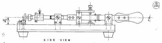
Fig. 1. Side view showing general construction of the semi-automatic (dash-dot sender) key described by G3BIK. The photograph on p.411 depicts the finished appearance, and all parts required (most of which can be made if they cannot be found in the junk box) are listed separately opposite.
