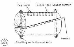
Fig. 1. Construction of a wooden mandrel, as described in the text, for winding transmitting coils. This is a re-usable former, and coils of different turns value can be wound up on it as and when required, the size being limited only by the length of the former.
