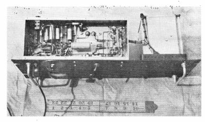
As constructed by G3MVY, the 25-watt modulator unit is mounted on a standard 19 ins. by 7 ins. rack; this view is with the bottom cover removed. Other forms of construction are possible, such as the open chassis with or without a screening cover, and this is always a matter of individual preference.
