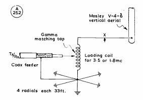
Loading up the Mosley V-4-6 for operation on the LF bands. With the appropriate coil in position—see text for 3.5 and 1.8 mc values—tuning is effected either by adjusting the number of turns or by inserting a variable condenser at point X. The loading coils for these bands can be built into weatherproof boxes with plug-in connectors.
