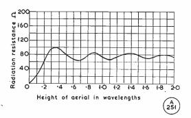
The well-known diagram showing the effect of aerial height on radiation resistance. A half-wave aerial is assumed.
