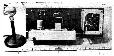
Impression of the general layout above chassis of the speech-amplifier/modulator described by G3MVY in the accompanying article. Provided the input side is properly screened, and layout of the parts approximates to the circuit diagram, any convenient form of construction may be adopted for apparatus of this sort.
