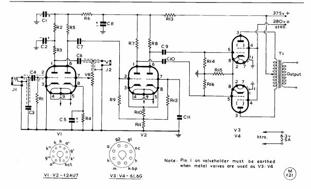
In this circuit, the speech amplifier values are chosen to restrict audio response to the speech-frequency range, though "quality" output (for a tape-recorder or pick-up) can be obtained by using the jack position J2. As a modulator with a crystal microphone at J1, any RF amplifier running up to about 50 watts input can be fully controlled with good communications-quality speech.
