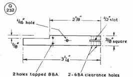
Fig. 3. The main moving arm, Item 17, for the G3BIK key should be constructed as shown in this sketch.
