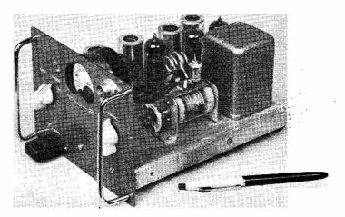
The TW-2 portable/mobile phone transmitter for two metres is a particularly neat job; it runs about 10w. input in the QQVO3-10 PA, with push-pull EL84's in the modulator. The speech amplifier gives ample gain from any standard crystal microphone. There is only one tuning control, for PA tank, as the oscillator-multiplier chain has pre-set adjustments for the crystal frequency used; the holder takes the FT-243 type of crystal.
