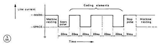
Fig. 1. The character of the  $7\frac{1}{2}$ -unit teleprinter code, explained in the text. The pulse lengths given, in milliseconds, are those of the American configuration of the code.
