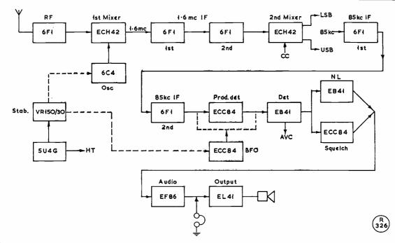
Block diagram of the home-built double-conversion superheterodyne receiver for the amateur bands designed and constructed by G2HFG; this receiver is illustrated in one of the accompanying photographs.
