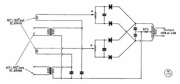
Fig. 2. Arrangement of the simplified balanced modulator, as discussed in the text. Potentiometers A and P are the carrier balance controls, the adjustment of which is explained in the article.
