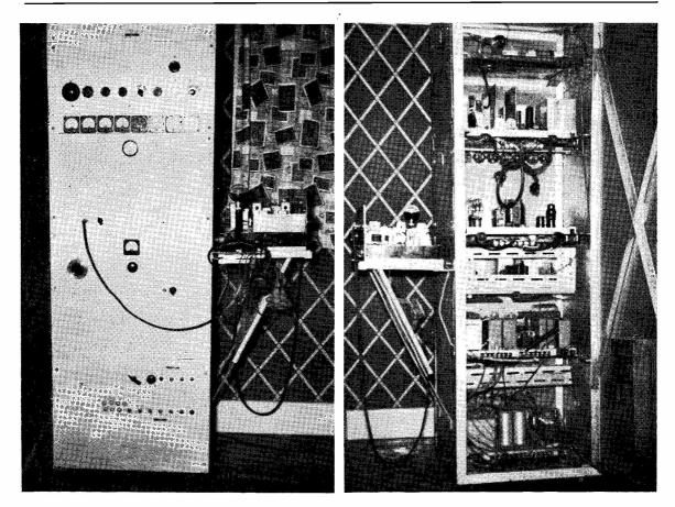
The station of G2HFG, 21 Alderton Road, Horfield, Bristol 7, is entirely home-built. The left-hand view is of the transmitter assembly from the front, the receiver being carried on a shelf at the side. The right-hand photograph is from the back of the transmitter cabinet, with the door open. The power packs are built on the lower-deck chassis, and at the top level is the aerial tuning unit.
