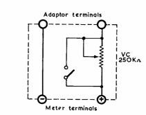
Fig. 9. An adaptor for safeguarding the meter while measuring the leakage current of electrolytic condensers.
