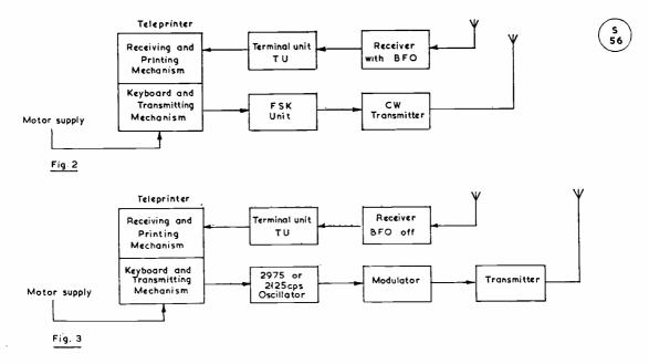
Fig. 2. Block schematic diagram of the layout of an FSK RTTY station. Fig. 3 shows the arrangement of an AFSK radio teleprinter station, transmit/receive.
