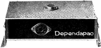
It employs a system (patent applied for) of switching by relay the Transformer taps and bias enabling you to use it on your receiver at 90% efficiency and when the Transmit relay is actuated the efficiency is 85% at 150 watts. A typical supply for a 6146 in the final modulated by a pair of metal 6L6's, 807's or TT21's, 530 volts at 228 m/a and 265 volts at 110 m/a is easily
