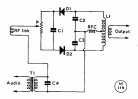
Fig. 1. With this circuit, the carrier can be balanced out by means of the potentiometer P; the output is then double-sideband.
