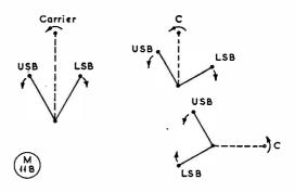
Fig. 3. Showing how, from the circuit of Fig. 2, the lower sideband is cancelled out.
