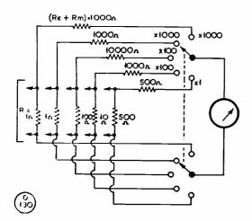
Fig. 7. The universal shunt employed for stage metering in apparatus, where the meter is switched into the required circuit.
