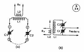
Fig. 2 (A) Basic arrangement for a simple universal ATU, for series or parallel tuning of a feeder line — see text. At (B) is another arrangement explained in the article, where one plate of C2 is bent to make a short-circuit in the maximum position,
