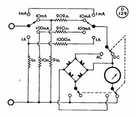
Fig. 6. Based on the Fig. 5 arrangement, a multi-range milliammeter utilising the universal shunt.
