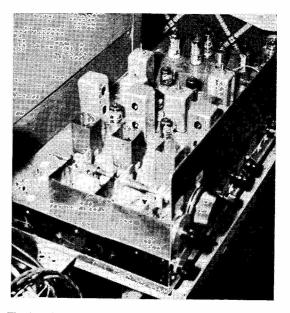
The 17-valve receiver built by G2HFG is a double-conversion arrangement, with 1.6 mc first IF and 85 kc second IF. The second oscillator is crystal-controlled — see block diagram.
