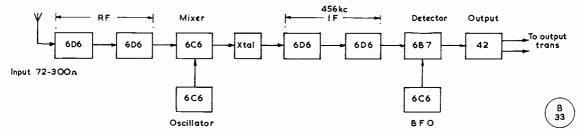
Fig. 1. Block diagram of the HRO Receiver, applicable to the pre-war models HRO, HRO-M and also the types suffixed MX, M/RR, M/TM, SR and JR. Certain later models use octal valves (6K7, 6J7, 6Q7 and 6V6), but the general schematic layout is unchanged.
