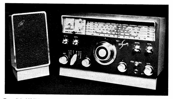
The new National NC-270 incorporates their famous "velvet vernier" dial assembly for easy SSB tuning, and a high degree of selectivity is given by a ferrite filter combined with a bi-filar T-notch. The frequency coverage is amateur band only, 80m. to 6m., and a 100 kc crystal calibrator is built in. A forward prop tilts the receiver slightly for more convenient operation.
