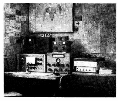
G3LSC is at Poole, Dorset, and started with the Top Band Talking Box — see "Short Wave Magazine," October 1956 — and a CR-100 receiver. Though he still has the Talking Box, the main transmitter is now a K.W. Vanguard, with a Cubical Quad for the 21 mc band. For 160 metres, he has a 250ft. wire, so arranged that the middle 30ft. section is in the vertical — another approach to the problem of getting the current antinode, where the radiation occurs, into the right place.
