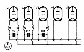
Fig. 5. Heater by-passing for the circuit shown in Fig. 4. C1, C2 are each .003  $\mu F$  and C3 is 270  $\mu \mu F$ . Values for the heater chokes are given with the coil table.
