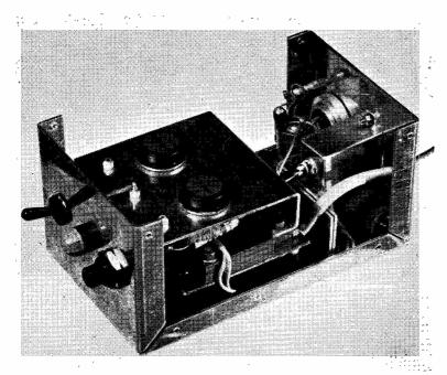
Upper chassis view of the transistor power unit designed and built by G3KUM, showing mounting of the power transistors and the general component layout. The final size is only 3 ins. by 3 ins. by 4½ ins. overall.
