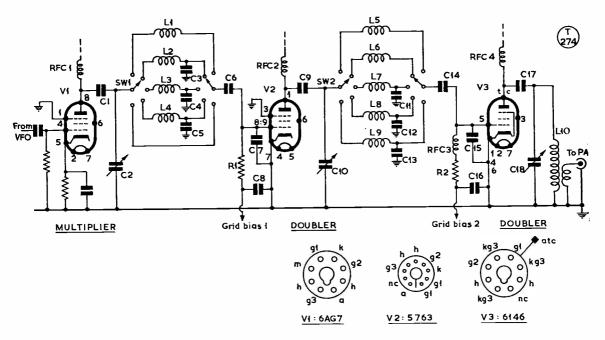
Fig. 2. The circuit arrangement as used by GM3IAA. V1 is a buffer or frequency multiplier, and V2/V3 are doublers. In the fifth position of the switch SwI, V2 operates as a buffer with C2 at minimum; this would permit operation on 3.5 mc, as ample drive is available. The anode of V3 is conventional, drive to the PA grids being by coax cable and link coupling. In this circuit, screen connections and all wiring not relevant to the method of inter-stage coupling have been omitted.
