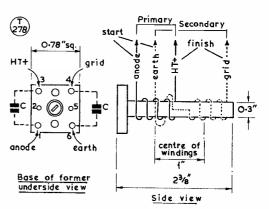
Fig. 2. Dimensions of former and winding details for the wide a band couplers described in the article.
