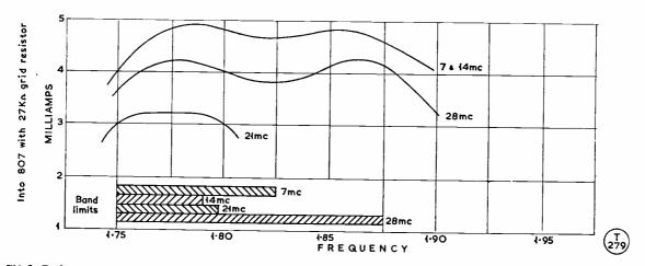
Fig. 3. Performance curves of the wide-band couplers described and illustrated in the article. These couplers are easy to make and full details are given in the text.
