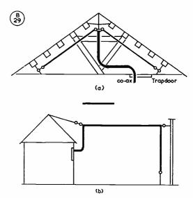
Fig. 1 (a). Layout for an indoor aerial, which can give very good results if installed as suggested in the text. The roof-space is always a suitable location for HF aerials if no outside arrangement is convenient or possible.
