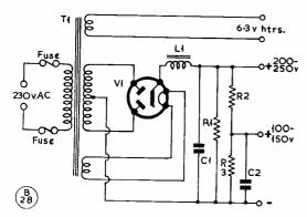
Fig. 2. Circuit of a simple general-purpose power pack, suitable for most receiver applications and for general work round the station. It can be built in a metal box, or on an open metal chassis with adequate protection, and in either case must be properly earthed.
