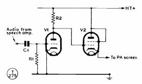
Fig. 1. Essential circuitry for the series-gate modulation system as specified for the DX-40U — see text. G3MMW has obtained better results on phone by modifying his DX-40U for screen control, as Fig. 2.
