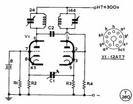
Fig. 1. About the simplest possible circuit for a two-metre crystal oscillator. The RF output at 144 mc will not be much, but it will be in the band. An 8 mc crystal is multiplied up in the sequence shown, and values are given in the table. The valve is a 12AT7
