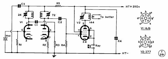
Fig. 2. Using a 6J6 and Z77 to get output at 144 mc from an 8 mc crystal. The multiplication sequence is 8-24-72-144 mc and there would be enough RF drive for a small buffer stage.
