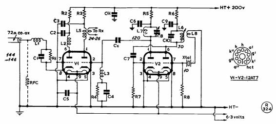
Fig. 3. A double twin-triode crystal-controlled converter circuit, using a pair of 12AT7's, and designed for a receiver tuning 24-26 mc to cover the two-metre band. Injection is at 120 mc, and the mixer output is peaked at 25 mc. A circuit of this kind, built as a small unit to fit inside the main receiver, could take power from it and would extend the range of almost any communications-type receiver into the two-metre hand.
