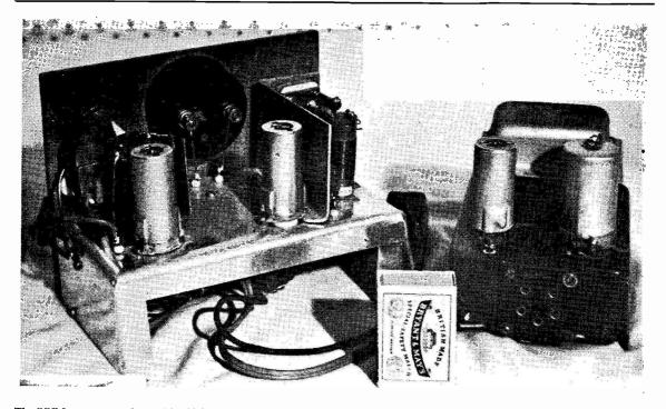
The QRP 2-watt transmitter with which G3NMX started up on 80 metres, with the results described in the article. A simple VFO-PA circuit, consisting of a 6C4 into an EL91 as PA, produced contacts with eleven European countries in a few days.
