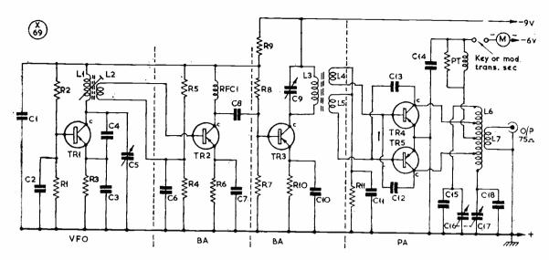
Fig. 1. Circuit of the 4-stage Transistor Transmitter for Top Band, designed and described by G3JRH. Running about half a watt in the push-pull transistor PA, G3JRH has worked 24 counties, and OK for the Continent. The circuit of the modulator is shown in Fig. 2 on p. 405.
