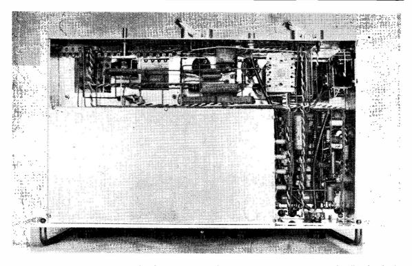
Neat wiring on the underside of the RF section of the G3CCA Transmitter. The screened compartment contains all the RF circuits, and connections into it are via feed-through condensers. On the extreme right of the chassis is the microphone pre-amplifier, with the audio filter circuits. The control relay is in the top right-hand corner.
