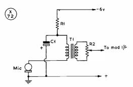
Fig. 4. The simplest arrangement is possible when using a carbon microphone for the Transistor Modulator.
