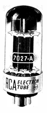
This is just about the actual size of the new RCA 7027-A, a beam power audio type. Two in Class-AB1 can deliver a maximum of 76 watts of audio with only 540 volts on the plate. The safe plate dissipation is 35 watts.
