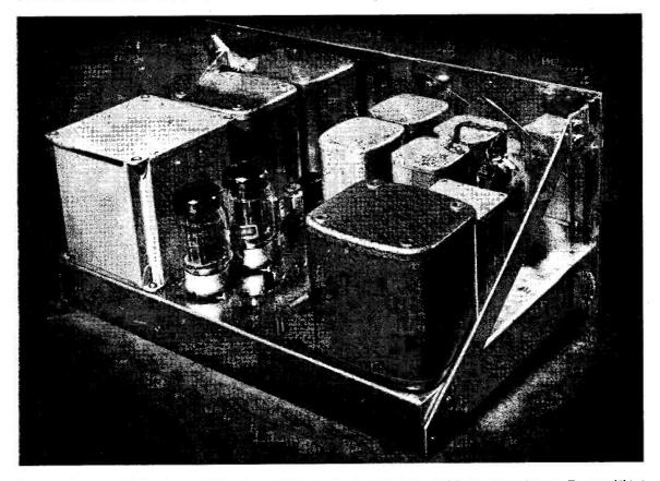
Chassis of the completed Modulator PA HT unit. At left nearest the front panel is the Modulator HT transformer. To near right at the rear of the chassis is the PA HT transformer. The CULA balancing potentiometer VR2 (see Fig. 8, and text) can be seen next to the KT88's, and on the extreme left is the modulation transformer.
