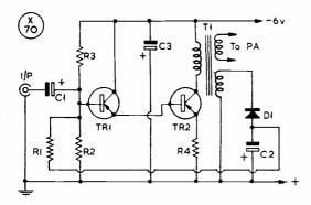
Fig. 2. Circuit of the modulator section for the Transistor Transmitter described by G3JRH. Various speech amplifier arrangements are suggested in Figs. 3-5 below.
