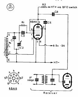
Fig. 1. Circuit of the BFO unit, considered as an addition to an ordinary general-coverage BC receiver. Values are: Cl, 200  $\mu\mu$ F; C2, 25  $\mu\mu$ F; C3, C5, 100  $\mu\mu$ F; C4, 2  $\mu\mu$ F, or "very small capacity"; R1, R2, 47,000 ohms; L, see text.
