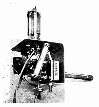
A beat-frequency oscillator unit (BFO) can be made up to work with almost any domestic broadcast receiver, some of which are capable of a good short-wave performance. As in this case, such a unit can be powered from the main receiver. The control rod is for the small variable condenser to swing the beat frequency across the main receiver IF.
