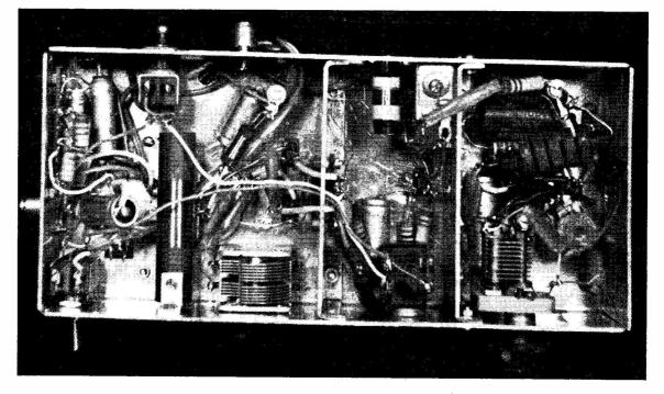
Layout under-chassis of the Transistor Transmitter, with the VFO compartment on the right. The audio section is to the extreme left, with the PA tank coil and tuning condenser towards the centre. The circuit in detail is shown in Fig. 1.
