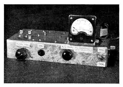
General view of the G3JRH half-watt Transistor Transmitter for Top Band CW/Phone operation. The home-constructed modulation transformer is at right behind the meter, with the RF section of the transmitter to the left. A unit of this type, run from a couple of dry cells, would make an excellent mobile-portable rig. The design discussed here is capable of surprising results — as G3JRH is able to show.
