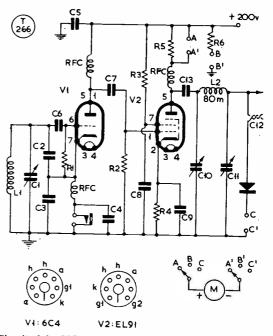
Circuit of the G3GKU 80-metre transmitter used by G3NMX, consisting of a VFO, V1, into a PA, V2 input 2 watts, coverage 11 countries.
