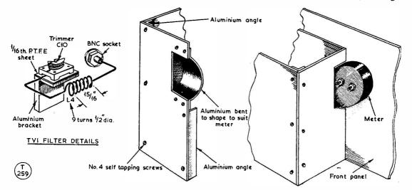
Fig. 6. Mechanical layout of the TVI filter (C10, L4 in the circuit on p.294 of the October issue) with screening box and meter mounting detail. For full TVI-proofing, it is essential to screen meters properly.
