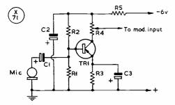
Fig. 3. Transistor speech amplifier circuit for use with a moving coil microphone.
