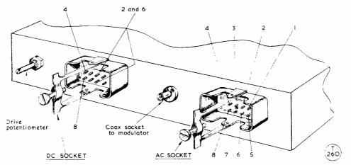
Fig. 7. RF unit plug mounting and wiring connections. Taking the DC socket, at left : 2,6 to X2-X6 in PA control circuit; 4, earth; 8, to X8 in modulator. Connections to AC socket, right: 1, to No. 11 in control circuit; 2, to No. 13 in control circuit; 3, live side mains; 4, front panel light; 5, to No. 22 in control circuit; 6, earth; 7, mains neutral lead; 8, front panel light. For cross-reference to the main relay control unit, see p. 347 November issue.
