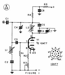
Fig. 1. The basic circuit of a Q-Multiplier. With full switching, this device can appear very complex on paper, but this simplified diagram shows a Q-Multiplier suitable for peaking signals only, without also giving the "match" facility, which requires another valve.
