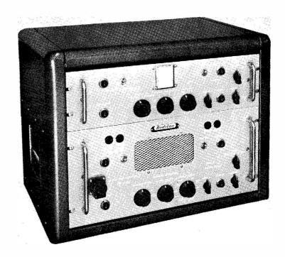
The Redifon Type GR.286 VHF/FM radio-telephone equipment has become an outstanding success in the marine communication field, and is now a standard fit in ships of the Castle and Clan Lines, and in tankers of the major oil companies. The transmitter frequency-coverage is 156.05-157.40 mc, on 18 channels, crystal controlled. The corresponding receiver section is a crystal-controlled double superhet with a first IF of 10.6 mc and second of 450 kc.
