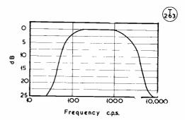
Fig. 3. The audio frequency response curve of the speech amplifier designed by G3CCA for his all-band transmitter.
