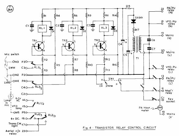
Fig. 4. The relay control circuit, using transistors, devised by G3CCA for the all-band transmitter described in the article. One switch on the microphone controls the whole relay unit, which performs all transmitter functions, with appropriate panel indication.
