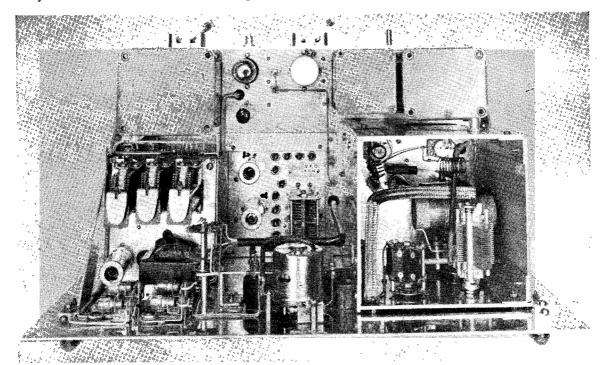
Top-side view of the RF chassis, with the control circuit, incorporated in the relay unit of Fig. 4, on the left, the PA "transmission time meter" in the centre, and the 6146 PA stage, clamper valve and pi-network in the screened compartment on the right. The Geloso type 104/4 VFO unit is at the centre of the chassis. The VFO/exciter power unit, to the circuit of Fig. 5, is at the rear, and the speech amplifier is underneath the relay control unit.
