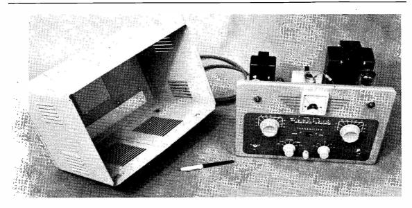
General appearance of the Heathkit DX-40U five-band transmitter before installation in its matching cabinet, with a size comparison. It runs 75 watts input on CW, and the controlled-carrier system of modulation drives the PA to 60 watts on phone. The kit of parts supplied is complete to produce the transmitter as illustrated.
