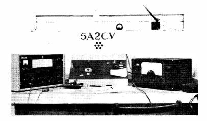
5A2CV, Tobruk, is an RAF-ARS club station, where they run a Panda Explorer as transmitter, with a Radiovision Commander receiver. Bands worked are 40-10 metres, CW and phone, and the 5A2CV boys are always glad of a call from U.K. stations. This winter, they hope to be  $\alpha$ 1,825 kc with a half-wave aerial positioned for Top Band working in this direction. For those fortunate enough tc QSO, it will be a new country and another continent.
