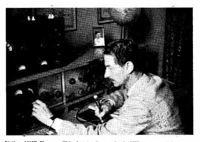
Station of IIIT, Florence. This photograph was taken by SWL Paterson, G-L018, on a recent visit. He reports that IIIT runs 150 watts in the transmitter and has a 12-valve communications receiver, all home-constructed. Aerials are a 20-metre Zepp, a dipole for 15 metres, and two-element rotary beams for 10 and 20 metres.
