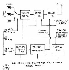
Fig. 1. Block schematic of the DX-40U CW/Phone Transmitter described and illustrated in the accompanying article.
