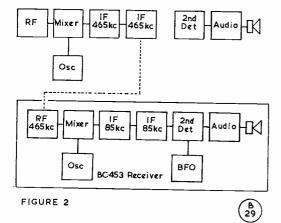
Fig. 2. Block diagram of a "Q5'er," using a BC-453 receiver, the tuning of which is set to 465 kc. In the arrangement shown here, the rear section of the original receiver is not used.
