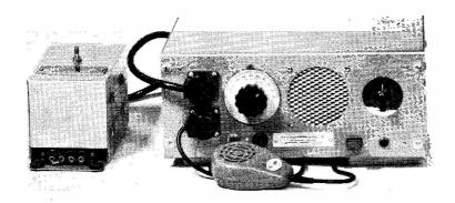
The new R.E.E. Communicator Mk.II is a VHF transceiver specially designed for mobile operation on two metres. The receiver section is a double-superhet, tuning 143-147 mc, with noise limiting. The RF power amplifier in the transmitter is a QQVO3-10A, screen modulated by a 6BW6. Size overall is  $5\frac{1}{2}$  ins. high x 13 ins. wide x 8 ins., deep.
