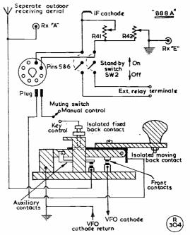
The circuitry and key connections involved in the modification suggested by G2NS. The effect is to give true BK operation with complete receiver protection.
