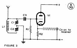
Fig. 3. A device known years ago as the "R9'er," which provides efficient aerial matching into the receiver — this alone will often lift signals two or three S-points. This version operates as a cathode follower.
