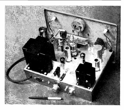
Inside the DX-40U Transmitter, showing general layout above chassis, which is punched ready for the acceptance of all parts. The power supply section is on the left, with the smoothing choke at lower right. The PA is a 6146 (Mullard QVO6-20) and its tank assembly can be seen immediately beneath the meter, between the tuning condensers. The switch on the rear chassis drop (foreground) is for VFO-crystal selection, with the aerial socket to the right and the accessory connector at left.
