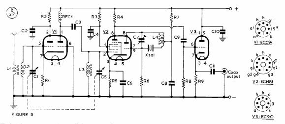
Fig. 3. A three-stage crystal-controlled converter for the HF bands, using a cathode-coupled double-triode RF stage, a triode-heptode crystal oscillator, and cathode-follower output to give a good impedance match into any usual type of main receiver, used as the tuned second IF section. There is a good deal in the design, construction, lining-up and satisfactory operation of HF-band converters, much of which is discussed in the text.
