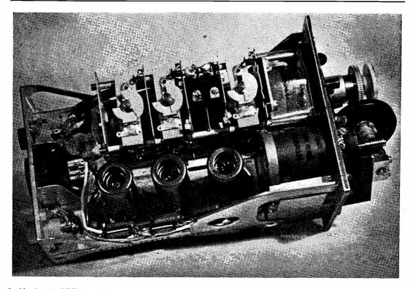
Looking into the RF Unit No. 1, showing the heater RF chokes and decoupling condensers in the lower foreground, with the new power plug and two coax connectors at the left-hand end of the chassis. To the right are the additional (edgewise) tuning knob and band indicator. Above are the trimmers and micro-switches, with the re-routed coax cable at the rear.
