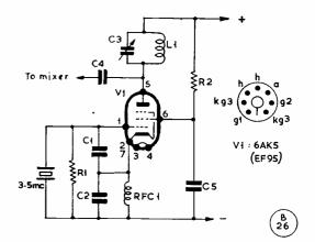
Fig. 2. Basic crystal oscillator circuit for harmonic operation. C1-C2 form a capacity divider on the grid-cathode side; L1-C3 in the anode circuit are proportioned to pick out the desired harmonic and should tune to 17.5 and 24.5 mc.
