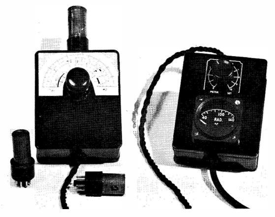
The grid-dip oscillator (GDO) as described in the article. For convenience, it is built into two boxes. The indicating meter is an aircraft-instrument type which has a very sensitive movement and, in fact, care must be taken not to "blow" the meter when the shunts are removed; the meter-setting is by a potentiometer. Plug-in coils are used to give a wide frequency coverage.
