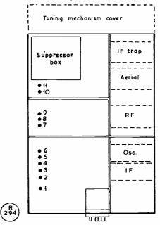
Fig. 1. Sketch showing locations of the feed-through insulators on the underside of the chassis in the Unit. Some of these have to be picked up for the conversion.
