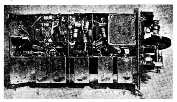
General view of the Unit below chassis, showing the termination of the aerial input coax cable at the IF trap, at lower centre of the compartment at upper right. The box in this compartment contains the suppressor components, not required for the application discussed in the article.
