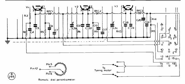
Fig. 2. That part of the circuit of the RF Unit No. 1 which is affected by the modifications discussed in the text — see Fig. 3 for full circuit and values. This diagram is to show the original power socket connections, including those to the tuning motor and remote control system, which are stripped out for the modification proposed by G3APA. Other items removed are the resistors R14 (22 ohms) and R15 (15 ohms).
