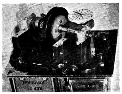
Front end of the Unit, showing the method of manual tuning. The added edgewise knob is fixed to the face of the large fibre pinion by adhesive only. With the front cover back on the assembly, only the edgewise tuning knob protrudes, control being smooth and positive by thumb-control — see another photograph.
