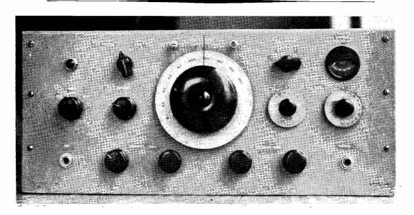
Front panel layout of the G3CCN SSB Transceiver, running 60 watts on 14, 21 and 28 mc, combined with a receiver having a crystalcontrolled oscillator, tunable IF and crystal lattice filter. The panel size is 18 ins. by 7 ins, and operation on either CW or phone is entirely automatic, in that change-over is by VOX control in either mode -- see text.
