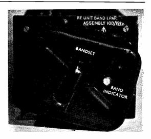
Panel plate of the RF Unit No. 1 as modified by G3APA. The thumb-disc tuning gives smooth and easy control through the 21-28 mc bands; this could, however, be improved upon by a dial assembly, with the conventional calibration markings. It should be noted that the legend "RF Unit Band 1" refers to a Service Band 1 of 19-35 mc, which bears no relation to the Band I of 19-35 mc, TV) of the present time.
