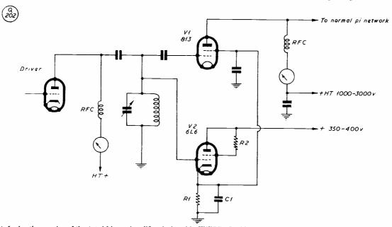
Fig. 5. Another version of the gated Linear Amplifier designed by W6EDD. In this case a grounded-cathode circuit is used and the amplifier screen voltage is controlled by the gate-control valve. Application of SSB drive increases the amplifier screen voltage. In this circuit, C1 is 2  $\mu$ F, oil-filled, 600v. working; R1 is 20,000 ohms, 10-watt, wirewound; and R2 is 100-200 ohms, 1-watt.
