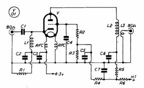
Fig. 1. Circuit of the RF pre-amplifier for two metres, described by G6TA, using a GEC A2521 UHF triode. This valve is capable of high gain with excellent stability. A suggested form of construction for the amplifier is shown in
