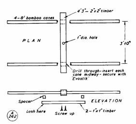
Fig. 2. Construction of the frame for the 10-metre "ZL Special." The cane lengths on which the dipole elements (made up of 300-ohm ribbon) are supported are themselves secured by a 4 ft. length of 1-in. by 1-in, wood strip, as shown in the elevation.
