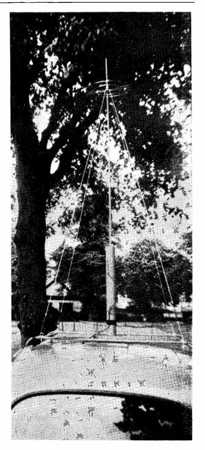
Seen at the Cheltenham Mobile Rally — the 160-metre "pyramid," complete with loading coil and capacity hat, on the roof of G3GTN's car.
