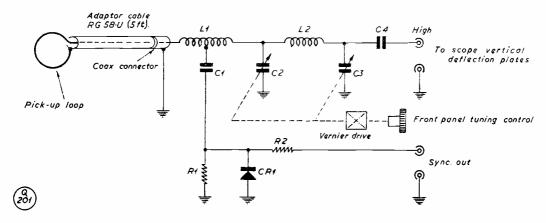
Fig. 4. The Vantron ''O-Probe'' is an instrument designed to provide the necessary coupling and voltage step-up when measuring sideband equipment with an oscilloscope. A pick-up loop samples the RF energy and feeds the multi-band tuned circuit through a five-foot length of coaxial cable. The tuned circuit covers from 3 to 30 mc continuously. A detector is included which will provide the 'scope with a sync, signal obtained from the sideband wave form.
