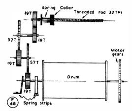
Fig. 8. The gear-train layout for the drum and the transverse drive for the stylus.
