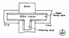
Fig. 3. The beam elements consist of lengths of 300-ohm ribbon, to the dimensions of Fig. 4, taped to the bamboo spreaders.
