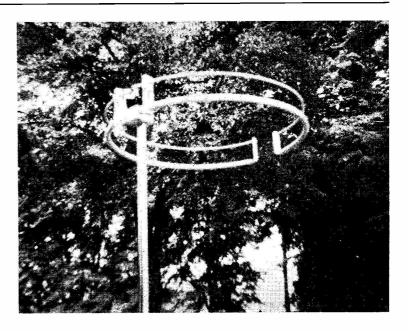
The two-metre halo now being used by G6VX/M, Cheltenham. This is an interesting design and is most effective, London stations having been worked from the hills above Cheltenham. The feed impedance is 75 ohms and some further details are given in the text.
