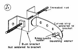
Fig. 7. The manner in which the stylus can be mounted; a gramophone needle is used, which has to be changed fairly often.
