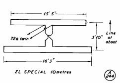
Fig. 4. Element layout for the 10-metre ZL Special, using 300-ohm ribbon feeder throughout. The transposition, or cross-over for the phasing line, is obtained merely by twisting the 46-in. length of ribbon connecting the centres of the sections.
