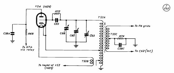
Fig. 1. Part of the VFO section of the Command transmitter type CCT-52232 (similar to the BC-457/459 series) covering 2.1-3.0 mc. This version has an electron-coupled oscillator of the grounded-anode type as VFO; nothing need be altered in this part of the circuit for the Top Band modification, except only that the padder C60 is increased in capacity — see text.
