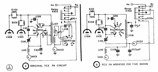
Fig. 1. The RF power amplifier section of the TCS (A) before, and (B) after modification for operation on the 14 and 21 mc bands. The essential change is the use of the roller inductance L108 as the PA tank coil for all bands 160-80-40-20-15 metres. This involves a fairly radical rearrangement of the PA section of the Collins TCS transmitter which, in the original, covers only the three LF amateur bands. Circuit element numbering is as used in the transmitter section of the TCS manual.
