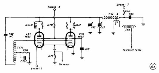
Fig. 2. The PA side of the CCT-52232 Command transmitter, running a pair of 1625's (12v. 807's). For the Top Band modification, the only alterations needed are the removal of one 1625 and the shorting of its heater connections; the removal of L52; and an increase in capacity on C67. The work involved in getting the CCT-52232 Command Tx on to 160 metres can actually be done in about an hour.
