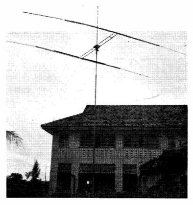
A full-size 20-metre beam is quite a large structure — when G3CCN was VS1HS in Singapore, he had this two-element array for the 14 mc band.
