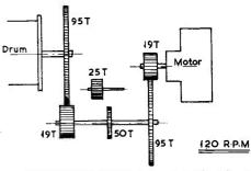
Fig. 6. Sketch showing gear layout and tooth ratios to get correct turning speeds — see text.
