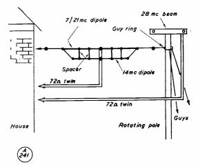
Fig. 1. General layout, showing the 7/21 mc dipole (half-wave on 7 mc, into three half-wave on 21 mc), with the 14 mc dipole physically "in parallel." The 10-metre ZL Special is on the rotatable pole, the dipole array acting as a horizontal guy. A sleeve or ring at the top of the mast is the termination for all three guys; the pole rotates in this ring and in a drain-pipe support at the foot. The 10-metre beam is fixed to the top of the pole at the point of balance.
