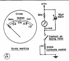
Fig. 3. Circuit arrangement for calibrating a meter to give proper visual control of dot-dash ratios when running an El-Bug, or electronic key.
