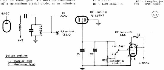
Fig. 4. The RF indicator device in the 20A Exciter. A magic-eye valve is used instead of a voltmeter. The triode rectifier may be replaced by a crystal diode. The switch can be set for maximum sensitivity, to permit carrier suppression adjustment, or for variable sensitivity using the magic-eye sensitivity control. The maximum undistorted peak output may also be observed following adjustments in the exciter.
