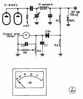
Fig. 3. A rather more sophisticated RF output indicating circuit, as used in the Hallicrafters HT-32; the sensitivity control R3 is adjusted for zero-dB on the meter (full-scale deflection), as a reference point, and carrier level can be read off directly when tone is removed. The sketch of the meterface shows the calibration (in the HT-32) in terms of actual carrier suppression.
