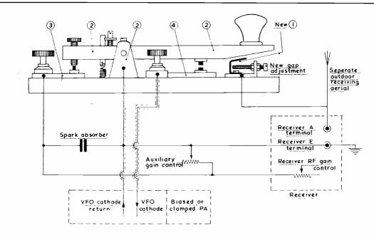
Fig. 1. Circuit arrangement for CW break-in working, as suggested by G2NS. (1) New auxiliary contact; (2) Common earth and all moving contacts; (3) Back contact; (4) Front contact. The key should be modified accordingly.
