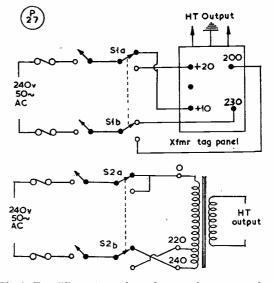
Fig. 1. Two different types of transformer primary connection are shown. The DPCO switch must be of the kind suitable for switching at mains voltage, and it is most important that the contacts "break before make," i.e., that they do not bridge.
