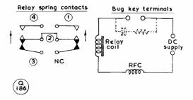
Fig. 4. Using the Type 600 GPO relay, with two sets of changeover contacts. Connections are as given in the sketch at Fig. 1
