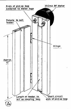
Sketch of the Kipper, which is self-explanatory. Indication is on an 0-350 mA RF meter, though the meter range depends to some extent on the power normally used. The pick-up loop is the length of 300-ohm ribbon (right-hand section), where a 300-ohm feeder line is in use. The general idea could be applied to any form of open-wire balanced feeder.
