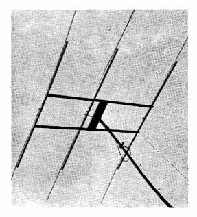
The three-element, 10-metre beam used by VQ1PBD on his Zanzibar expedition was constructed of ordinary H-section curtain rail, on a wooden mounting using curtain-rail supports. The whole thing can be broken down into a number of sections not more than 9 feet long, for easy transport.
