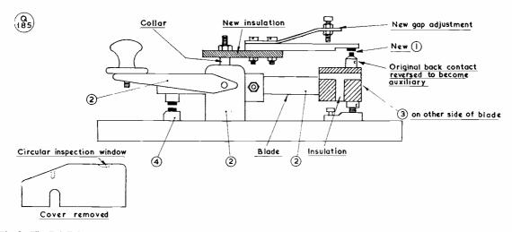
Fig. 3. The R.A.F. key Type 1969 — the pattern with a cover and an inspection window — can be modified in accordance with this sketch to give receiver muting and aerial shorting to earth. The principle is the same as in Figs. 1 and 2.
