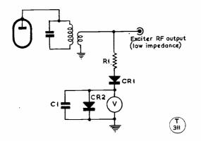
Fig. 2. A carrier null-RF output indicator. This circuit provides for continuous monitoring of the carrier suppression, without over-driving the meter on voice peaks. The selenium rectifier CR2 ' shorts " the meter at high values.
