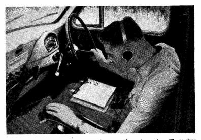
Interior installation for G3KEQ/P, CW or phone operation on two metres. The receiver is a 6BQ7A cascode and the transmitter runs a QQVO3-10 at 15 watts, the beam being a portable 4/4, slot fed, which can be pushed up to 27 feet.
