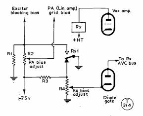
Fig. 5. A circuit, devised by YU1AD, for a voice-controlled operating system. It requires only a single-pole doublethrow set of contacts on the relay; the latter should be the sensitive type, with a DC coil resistance of 5-15,000 ohms, operating at 1-2 mA only. The adjustable voltage-divider, R1-R2, sets the PA bias, and R4 the cut-off bias for the receiver. The diode may be any vacuum type. At YU1AD, this control circuit is used with parallel-6146's as the linear amplifier.
