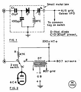
The circuit arrangement discussed in the article by G3KQH. Change over from AM to NBFM is by the switch. The lead from the pre-set 20  $\mu\mu$  frondenser C should be made as short as possible, as it is "hot" to RF. As explained in the text, the deviation must be kept low, not only to minimise adjacentchannel QRM but also to make the signal resolvable on an AM receiver.
