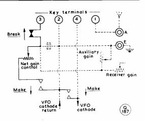
Fig. 5. Circuit for net, gain control and key short (for phone), using a manually-operated key switch having two sets of "make" and one pair of "break" contacts.
