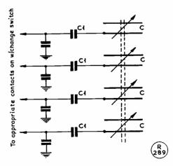
Fig. 2. Method of obtaining improved band-spread when using the R.107 RF/IF packs as part of a double superhet. Capacities marked C are the existing 300  $\mu\mu\mathrm{F}$  sections of the 4-gang tuning condenser, and those marked C1 are all 75  $\mu\mu\mathrm{F}$  1% silver mica condensers.
