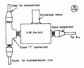
Fig. 6. Suggested constructional layout for the T-R switch shown in Fig. 5. The unit is fully screened and all RF lines are run in coaxial cable. The transmitter output is in effect connected through the T-R switch by means of the T-connector, making for short and direct RF leads.
