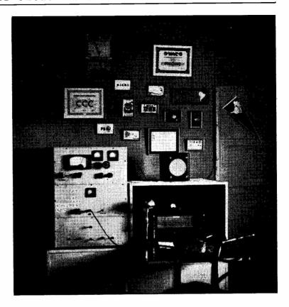
The equipment at LU1HB, Rio Ceballos, includes an Eddystone 888A receiver and a home-built transmitter running a pair of 807's in the PA. His aerial for 21 mc is a 3-element beam.
