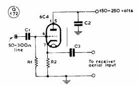
Fig. 2. A cathode-follower T-R switch. Resistors are 1-watt non-inductive, and the input and output circuits should be screened to prevent feed-inrough coupling. Values are: C1, 50  $\mu\mu$ F, 500v.; C2, .005-.01  $\mu$ F; C3, .01  $\mu$ F; R1, 1 megohm; and R2, 500 ohms.
