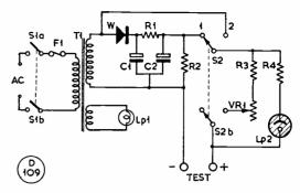
the test terminals, and switch to Posn. 2. When testing electrolytics, observe the *polarity* of the test terminals, and remember, only the leaks can be checked here.
