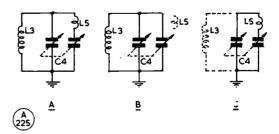
Fig. 1. Basic circuitry of the RF tank section of the Z-Match Unit. (A) is the AFU circuit, with link couplings omitted; (B) is the ATU equivalent circuit for the range 3.5 to 7.0 mc; and (C) is the configuration for 14-30 mc.
