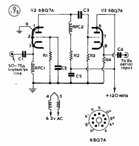
Fig. 3. A much more refined type of T-R switch, using a twin-triode. Values are: C1, 500  $\mu$ F; C2, C4, .01  $\mu$ F; C3, C5, .001  $\mu$ F; R1, 1 megohm; R2, 1000 ohms; R3, 50,000 ohms; R4, 100 ohms; RFC1, 2.5 mH; RFC2, 21  $\mu$ H (10-metre) RF choke; Htr.4/5, bi-filar wound. All resistors are  $\frac{1}{2}$ -watt non-inductive. RFC2 is a single-layer VHF-type RF choke, and is not critical; the special bi-filar choke, in the heater leads, is explained in the text.
