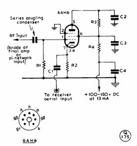
Fig. 5. A transmitter tank T-R switch. Such a unit should be mounted in a screened box, with the valve also screened; all leads to the receiver and external power source must be fully screened, too. Values are: C1, C2, C4, 01  $\mu$ F; C3, 001  $\mu$ F; R1, 1.2 megohms; R2, 220 ohms; R3, 1000 ohms; and R4, 270 ohms. Resistors can be all  $\frac{1}{2}$ -watt non-inductive, and the condensers the disc ceramic type.
