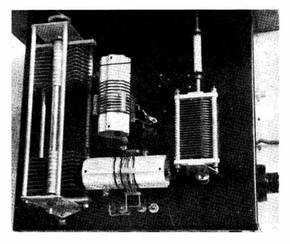
Chassis layout of the Z-Match Unit designed by GW3LJS. The large two-section condenser on the left can be fabricated from a readily available "surplus" type, as described in the text. The L1, L2 assembly and the 80-ohm dummy load resistor R3—see circuit Fig. 2—are mounted sub-chassis. The unit is intended for high-voltage operation at full power; for inputs of 75-80 watts with up to 800v. plate HT, condenser spacings could be scaled down.
