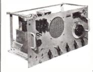
Complete with 6 valves, 2-6K8G, 2-EF39, 6Q7G and 6V6G. Internal mains and 6v. vibrator pack, Built-in 64\* P.M. speaker. Muirhead slow motion drive. B.F.O. head slow motion drive. B.F.O. and R.F. stage. Provision for 'Phones and Muting and 600 ohms line combined input, 100/250v. A.C. or 6v. D.C. All sets in new condition and air tested.
