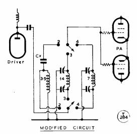
Fig. 2. The recommended modifications for the PA grid stage of the TA-12, to ensure TVI-proofing. If this is not a problem, the grid side can remain as in the original (at left above) except that certain coil changes are desirable, as explained in the text. The value of the condenser Cx in the right-hand circuit is 25  $\mu\mu$ F, and for 7 mc the pi-tank capacities are 80  $\mu\mu$ F each; for 14 mc they are 40  $\mu\mu$ F.
