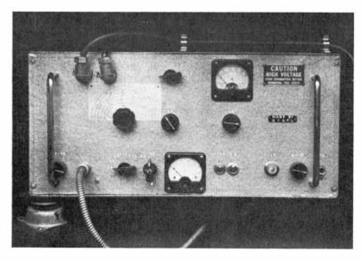
This is the mobile transmitter designed and built by G3ATL and discussed in the article With an adjustable aerial system (see Fig. 2), all bands from 10 to 160 metres can be used. DX phone has been worked successfully on the HF bands, the best contact so far being with a VS1 in Singapore, while actually motoring.
