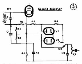
Fig. 1. The noise limiter circuit suggested by G3JBU for incorporation in a BC-342 (or BC-312, which is the same thing except for the power supply). Good results are claimed for this limiter under practical operating conditions.
