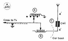
Fig. 2. The aerial layout evolved by G3ATL for six-band (10 to 160 metre) mobile working. Details for the coil arrangement are given in the table; it will be noted that combinations are changed for the different bands.
