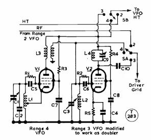
Fig. 1. This diagram shows the circuit of the VFO/doubler combination used on Ranges 3 and 4, in G3BST's TA-12 modification. Considerable simplification is achieved by converting the Range 3 VFO to work as a doubler, as explained in the text.
