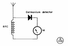
Circuit of the aperiodic radiation meter which, by its very simplicity, can become one of those indispensable items of test gear. The germanium detector and the RF choke are standard items, and can be wired in behind the meter itself (like a shunt).
