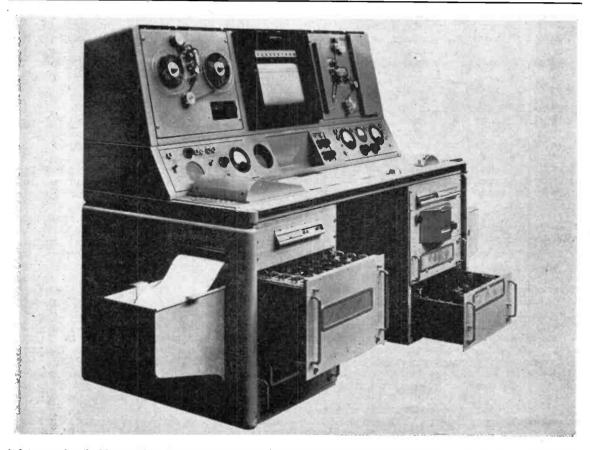
A data recorder, the Mervyn Midas, in which the usual mirror galvanometer with photo-sensitive recording paper are replaced by a tape medium. In this case, "Scotch Boy," made by Minnesota Mining & Manufacturing Co., is used. Tape recording ensures a wider frequency response, a higher system accuracy and produces a record more suitable for analysis.
