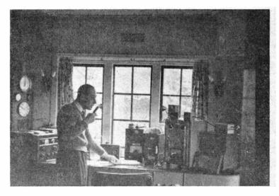
Having moved, G3HCU is now set up at his new QTH at Peaslake, Surrey. Visible are the beam direction indicator and 24-hour clock, and the AR88, at left, next the Top Band and two-metre gear, then the LG.300 transmitter and BC-221 frequency metre. The aerial system includes beams for 10, 15 and 20 metres (under construction) a G8KW multi-band, and a 256 ft. wire for 160 metres. All the equipment is relaycontrolled by switches on the desk panels.
