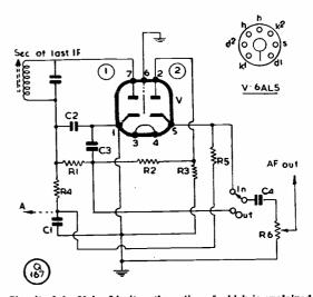
Circuit of the Noise Limiter, the action of which is explained in the text. It is of the type which gives a marked cut-off, but with most receivers any serious loss of audio can be made up by advancing the volume control. The circuit is particularly effective against any sort of peaky noise.
