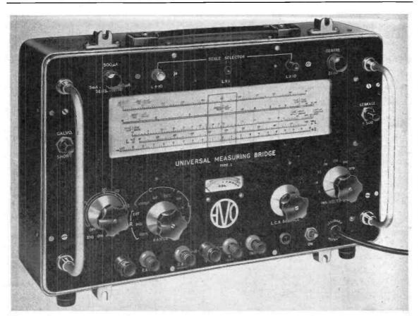
The new AVO Universal Measuring Bridge, Type 1. It measures inductance and capacity at 1,000 c/s, and resistance using DC. This instrument sets a new standard by virtue of its clear and simple presentation of measurements.
