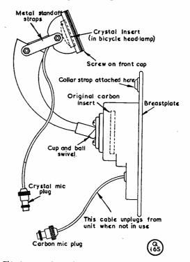
Fig. 1. Adapting a breast-microphone assembly — of the type frequently advertised as "surplus"— to make a mounting for a crystal microphone insert. This arrangement, which retains the original carbon microphone for use if required, makes a convenient and flexible microphone set for general use, either for mobile operation or about the station.
