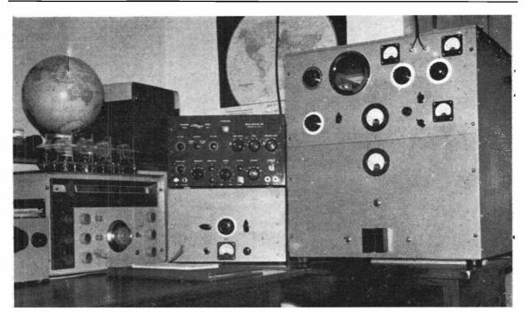
This is another view of the station of ZE5JJ, Salisbury, Southern Rhodesia, featured in the heading to "DX Commentary" in the April issue. Operating on SSB, the transmitter side consists of a home-built VFO into a commercial SSB exciter unit, driving an 805 as PA in the Class-B zero-bias linear arrangement. The receiver is a National NC300, and the station is fully voice-controlled. The aerials at ZE5JJ include a 3-element beam for 20 metres, with dipoles for the 15- and 10-metre bands.
