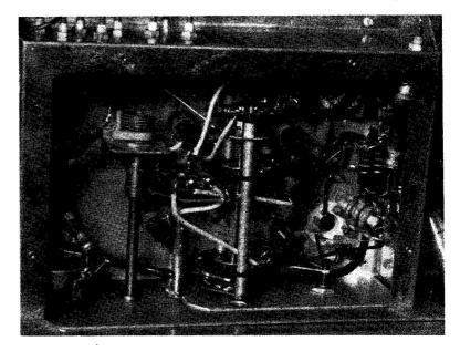
The under-chassis modification for Top Band, applied to the Geloso Type 4/102 VFO Unit, and equally applicable to either mark of Geloso "Signal Shifter." The additional switch unit SAI/SA2 (see Fig. 1a/Fig. 1b) is fitted alongside the existing main bandchange switch, with coils LA1 and LA2 adjacent; the actual positioning will immediately be clear on examination of the Geloso VFO with this photograph.
