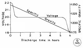
Fig. 2. Typical curves showing how voltage and specific gravity of an accumulator vary during discharge. The article discusses correct charging procedures and general maintenance.
