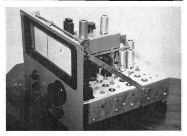
The RF Front End unit designed by G3KGN, to go with his IF/AF Amplifier described in September 1957. The panel controls are RF gain, oscillator set frequency, switch S2, band-change switch S1, the main tuning capacity and aerial trimming condenser C5. Stages V7, V8 are on the sub-chassis above the tuning gang. The dia lhad not been calibrated when this photograph was taken.
