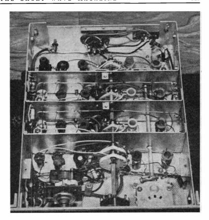
Underneath the G3KGN RF unit, showing general layout and construction. The central switch-line is the band-change, and the oscillator section is in the first compartment from the front.
