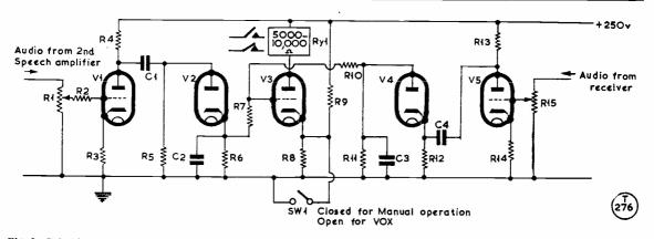
Fig. 3. Suitable VOX circuit for the G2NH SSB Exciter, with loud speaker anti-trip facilities (essential if a speaker is used). The circuit is derived from that of the Collins KWS-1 transmitter, and works well with the Exciter described in the December 1957 issue. The relay Ry1 should be of the fast-acting type for fully effective voice break-in working.
