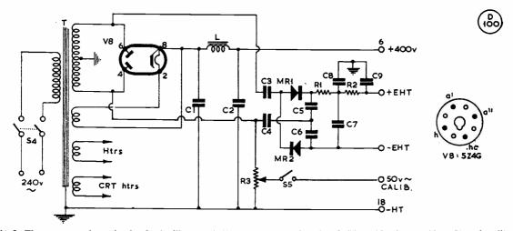
Fig. 5. The power supply section for the Oscilloscope, built as a separate unit. The R3, S5 combination provides a 50-cycle calibration voltage, and the tube EHT is derived from metal rectifiers, R1, R2, being the smoothing resistors. All values are given in the table opposite.
