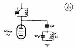
Fig. 1. The 25 mc trap circuit mentioned in the text; it functions as a "sucker" to eliminate the 25 mc output from the 10/15 metre mixer. Coil L1 can be 20 turns of 30g. on a  $\frac{1}{2}$ -in. slug-tuned former of the Aladdin type, spaced to fill the length.
