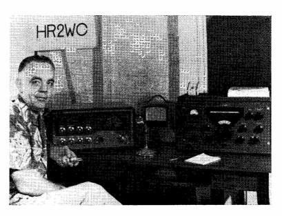
HR2WC, Cortes, Honduras, is ex-YN1WC and was licensed as W6EWC in 1931. HR2WC started on 80-metre SSB in 1953 and now runs a kilowatt, with a Collins 75A-2 receiver and a Hallicrafters HT-32 Exciter. The aerials are a 7/21 mc doublet, and a dipole for 14 mc.
