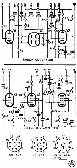
Fig. 6. These important units are constructed on small subchassis, and can be fitted after testing through. The top diagram shows the sweep generator, and below is the deflection amplifier. The inter-connecting wiring and control switching are given in Fig. 7.
