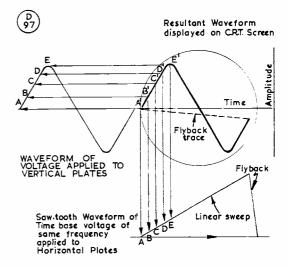
Fig. 2. Showing how a sine wave is traced out on the screen of a cathode-ray tube, when connected into the appropriate circuit. The picture can be made to "stand still" by proper adjustment of the controls.
