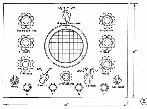
Fig. 4. Front panel layout adopted by the author for the instrument described in the article. On a panel 10 ins. wide by 8 ins. deep, the knobs can be arranged symmetrically round the tube face, and placed for convenient operation. The experienced constructor need not be bound by this layout, which can be varied to suit individual convenience, or the panel and chassis that may be available
