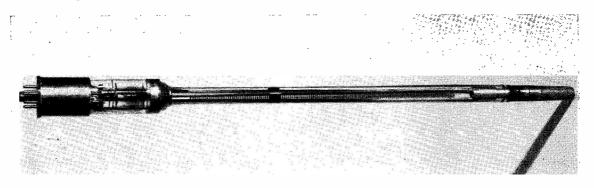
A new type of valve, of which we shall hear much more in the future — the G.E.C. (M.O. Valve Co.) Type TWS-1 travelling-wave tube, which gives an output of 38 watts, with a power gain of 26 dB, in the 1500-3000 mc frequency range. The TWS-1 is convection-cooled, and is suitable for broad-band amplifiers.
