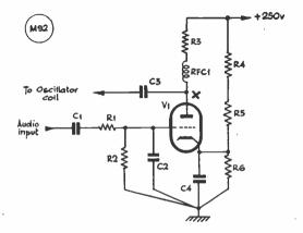
Fig. 6. Circuit for a reactance modulator providing the effect of variable capacity. V1 can be any triode with low internal capacities.
