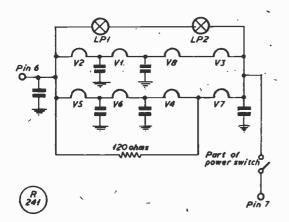
Fig. 3. This is the dial-lamp and beater circuit modification suggested by G8PG to enable the receiver to be run from a normal LT supply; it is designed for 24v. operation.
