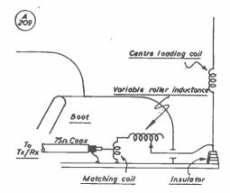
Fig. 3. Electrical layout of the G3CIM/M aerial system, showing arrangement of the loading and matching coils. The variable inductance is roller-tuned by remote control from the operating position.
