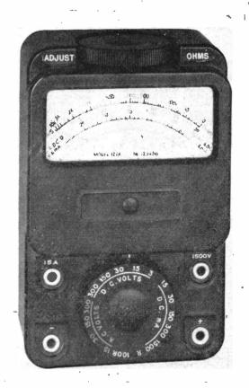
The Taylor Model 122A is a pocket-size multi-range Universal Meter, rated at 5,000 ohms-per-volt, giving 21 AC/DC ranges up to 1500v. AC and 15 amps DC. The Taylor range of test and measuring instruments includes insulation testers, capacity and inductance bridges, valve testers and oscilloscopes.
