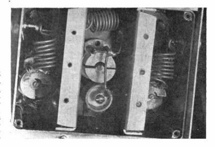
The low-pass filter as designed and constructed by G2HKU, and described in his article. An Eddystone die-cast box, partitioned as shown, is used and the degree of attenuation to be expected with the device is indicated in Fig. 3. Once adjusted, the variable capacities are sealed with the unit inserted in the transmitter output in the manner shown in Fig. 4.
