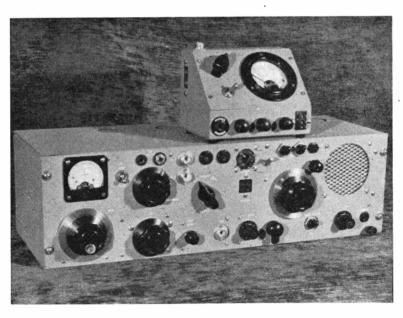
The complete mobile transmitter-receiver-monitor unit installation designed for G3CIM/M, in a Ford Prefect. The monitor box is an important and very useful auxiliary item, the circuit of which is given in Fig. 2. Another photograph shows how the assembly fits into the parcel shelf on the car.
