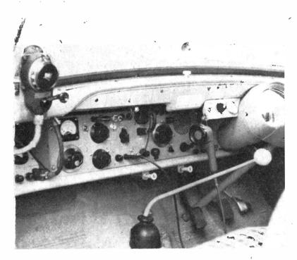
The fitting of the G3CIM/M installation into the parcel shelf of Ford Prefect 633-GEX. The aerial control winch is at upper left; this adjusts the variable section of the aerial coil assembly in the boot—see text and Fig. 3. The monitor unit shown in another photograph is at the left.
