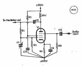
Fig. 7. The difference between this circuit and Fig. 6 is that here the reactance modulator simulates a variable inductance. Values are given in the table, and the valve can be a 6AM6.
