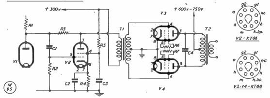
Circuit for the KT88 Class-B modulator, with a KT66 driver stage. With this arrangement, a full 150 watts of audio can be obtained under the conditions stated in the article. The KT66 needs but 15v. grid drive, and in this circuit will produce the necessary 360v. across the grids of the KT88's to drive them to full output. In this application, the G.E.C. KT88 is much superior to the conventional 307, so often featured in Class-B zero-bias modulators.
