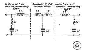
Fig. 1. For this circuit, values would be : C1, 40  $\mu\mu$ F; C2, 130  $\mu\mu$ F; L1, 0.36  $\mu$ H; L2, 0.21  $\mu$ H; and L3, 0.345  $\mu$ H. Fig. 2 shows the practical expression of this arrangement.
