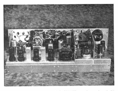
General construction behind the panel of the G3CIM/M transmitter-receiver; the PA section is second from the right. The receiver runs 12v. valves (see Fig. 1), incorporates a noise limiter, and itself involves seven of the 14 valves used in the complete installation.
