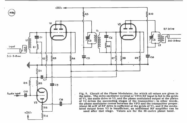
sideband levels is the same as that outlined earlier for the reactance circuits. The provision of a potentiometer with some sort of calibration on it for the audio input is necessary to enable the settings to be reproduced at will after the initial adjustments are completed.
