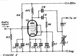
Fig. 1 shows the crystal frequency shift circuit suggested by G3FMO; it will give a good move when the frequency is multiplied up, with perfect stability if the process is not taken too far. At Fig. 2 is the application of this circuit to FM phone working; the tank circuit values are as normally obtain.
