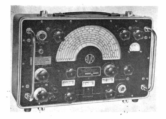
The AVO Signal Generator Type 378 is a CW/AM RF instrument covering the wide range of 2-225 mc; it employs modulation on the post-oscillator stage and provides an amplitude modulated RF signal with negligible FM effect. The Type 378 is ideal for use with AM receivers.
