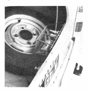
Installation of the G3CIM/M aerial system, showing the variable inductance coil section in the boot, controlled from the operating position. The electrical layout is shown in Fig. 3, and the winch for resonating the variable inductance in one of the photographs.
