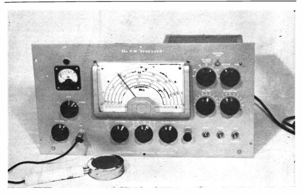
Front view of the K.W. Vanguard Transmitter, as made up from the kit of parts (which includes an enclosing cabinet, not taken with this photograph), showing the general panel arrangement. Behind the central dial is the Geloso Signal Shifter Type 4/102, which is the drive unit for the Transmitter, running a 6146 (QV06-20) PA at up to 45 watts input, phone and CW. The switching gives full control and the Geloso VFO ample drive for the PA, on all bands.
