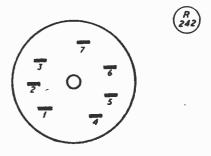
Fig. 4. Sketch to locate the pin connections on the multi-way socket, when viewed from the front.
