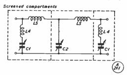
Fig. 2. A practical low-pass filter, as designed by G2HKU. For C1, use a 50  $\mu\mu$ F air-spaced variable, pre-set, to get 40  $\mu\mu$ F; for C2, a 100  $\mu\mu$ F air-spaced pre-set variable, with a 50  $\mu\mu$ F ceramic fixed condenser in parallel, to get 130  $\mu\mu$ F; L4 is 0.31  $\mu$ H, which can be 7 turns of 16g. ½-in. diameter by 1-1/16 in. long; and L5 is 0.50  $\mu$ H, 9 turns as L4.
