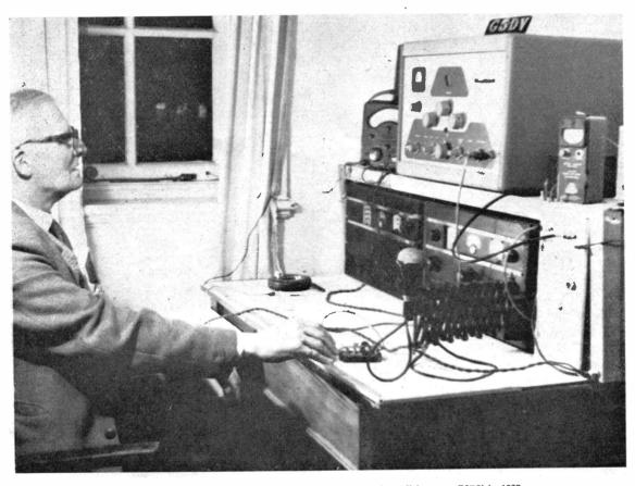
Originally licensed as G5AS more than 25 years ago, the call became G5DV in 1937, and the location is now R.A.F. Upavon, Wilts. The transmitter is a Heathkit DX-100, below which are the two AR88 receivers.
