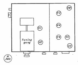
Fig. 2. This sketch is to locate the valve positions and types on the chassis of the CR-300; details of the valves used are given in the article.
