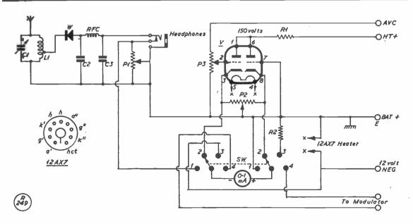
Fig. 2. The monitor unit designed by G3CIM for his mobile installation, the functions of which are discussed in the text. Values are as follows: C1,  $100~\mu F$ ; C2, C3, .001  $\mu F$ ; R1, to reduce HT to 150v; R2, to suit meter resistance, about 20,000 ohms; P1, F/S meter sensitivity, 500 ohms; P2, S-meter zero-adjust, 500 ohms; P3, S-meter sensitivity control, 2 megohms; RFC, 1 mH; W, crystal diode; Sw, 2-pole 4-way break-before-make; L, to tune band required with C1; V, 12AX7.
