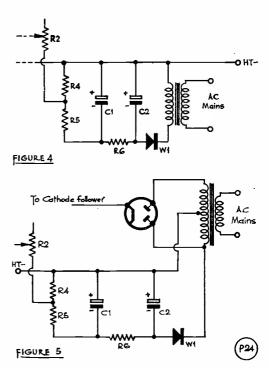
Figs. 4 and 5. Power supply and control circuits for the Variable Voltage unit.
