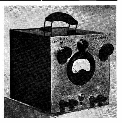
General appearance of the Variable Voltage Power Unit as described in the article. Size can be judged from the fact that the meter is a  $2\frac{1}{2}$ -inch dial instrument. Output is continuously variable over a wide range by the circuit arrangement shown in Fig. 6.
