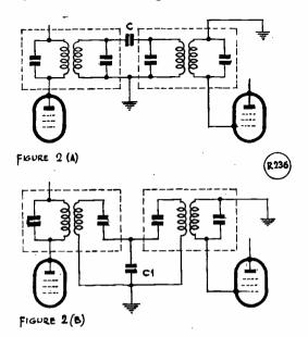
Fig. 2A. High impedance or "top coupling" between two IF transformers. Fig. 2B. Low impedance or "bottom" coupling between IF transformers.
