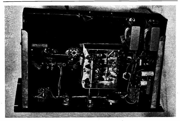
Under-chassis view of the R.A.F. Amateur Radio Society kit transmitter, as wired out ready to go on the air. The smoothing chokes are upper right, and the function switch S3 at lower right. The central assembly is the underside of the Geloso VFO Unit, with the QVO6-20 valveholder to its upper left. The switch below left is the meter change, S2.
