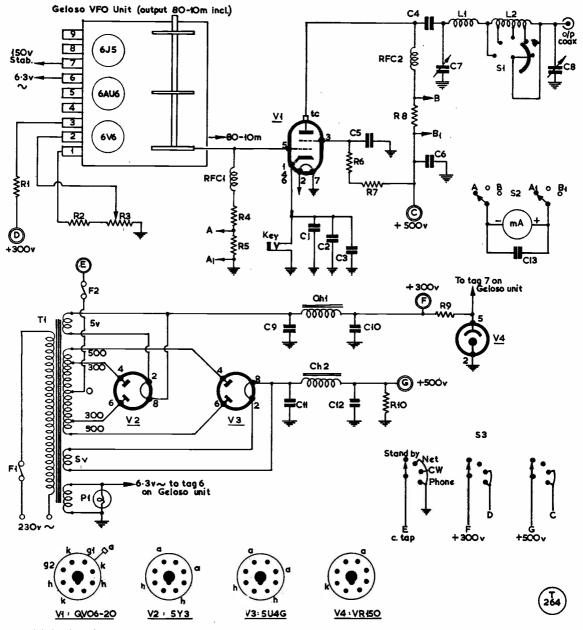
Essential circuitry of the HF-band kit-type transmitter, on which notes are given in the article. A standard Geloso VFO Unit drives a band-switched PA, and the power supply capacity and control switching provides for either CW or phone working — though, as sent out to R.A.F. Amateur Radio Society club stations, a modulator is not included in the kit. A number of these transmitters are already on the air at the stations of overseas member-groups of the R.A.F.-A.R.S.
