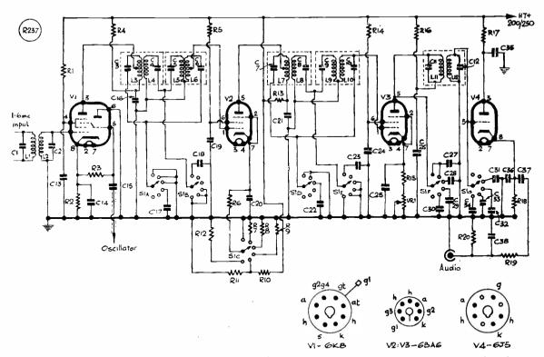
Fig. 3. Finalised circuit proposed for a high-selectivity IF amplifier, for operating at 1.6 mc. Variations on this basic design are possible, as explained in the text; six different bandwidths are given by the circuit shown here, for which all values are in the table.
