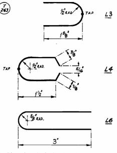
Fig. 2. Dimensions details for the hair-pin inductances in the G3AST 430 mc tripler-PA unit. The wire specified is 17g. Lewmex-M enamelled, which could be substituted by 16g. enamelled copper.
