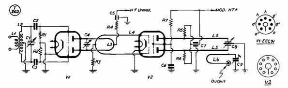
Fig. 1. Circuit of the 70-centimetre tripler-PA unit designed and described by G3AST. The RF output valve is a Mullard QQV02-6, and the general layout arrangement is shown in the under-view photograph. Dimensions for the loop inductances are given in Fig. 2, and all values in the table herewith.
