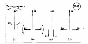
Fig. 1. Showing relative positions of sideband and carrier phases during one cycle of audio frequency with amplitude modulation. Ic is the carrier amplitude, and Im the sideband
