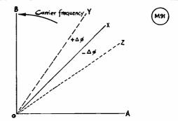
Fig. 5. Showing the variation of phase with the application of phase modulation.
