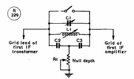
Fig. 3. As suggested in the article, a T-notch rejection filter can be used instead of the "Q-Multiplier." In this circuit, values are: C1, 100  $\mu\mu$ ; C2, C3, 003  $\mu$ ; R1, 15,000 ohms; L1, 4-5 mH.
