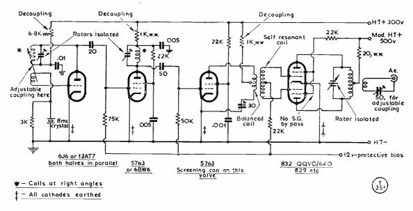
Fig. 11. The points to watch in the layout and construction of a two-metre transmitter, if stable operation is to be obtained under full modulation. The circuit values as shown are correct for the 144-146 mc band, and coils are as normally used; some data are given in the text. It will be noted that for de-coupling, low-value wire-wound resistors are used; the advantage of this is explained in the article. The circuit as shown here represents good modern practice in VHF design and technique.
