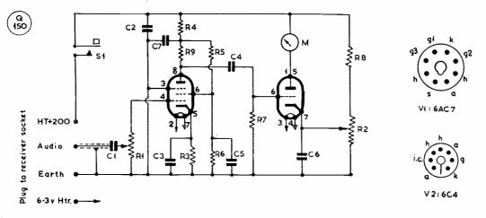
Circuit of the Modulation Meter, designed as an auxiliary unit for any usual type of communications receiver, from which it could take its power. The effectiveness of the arrangement depends upon the accuracy of the initial setting-up procedure, since it is a reference system, as explained in the text. Even if not accurately calibrated, however, it will always compare, reliably, the depth of modulation between different stations on the same band.
