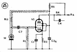
Fig. 2. When using a condenser microphone, the input circuit can be arranged as shown here. C7 is .01  $\mu$ F, 350v. working, and R11 anything from 20 to 40 megohms. Shielded and earthed leads should be used as indicated.
