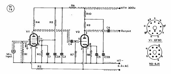
Fig. 1. Circuit of the head amplifier as discussed by G5GQ in the article. An EF50 gives ample voltage gain for the 6J5 in the second stage. To reduce the possibility of hum and because the current drain is very small, the EF50 is run at reduced heater voltage; in this particular application, it does the valve no harm. A condenser microphone is mentioned but a crystal type could be used equally well. The input and output leads should be run in shielded cable.
