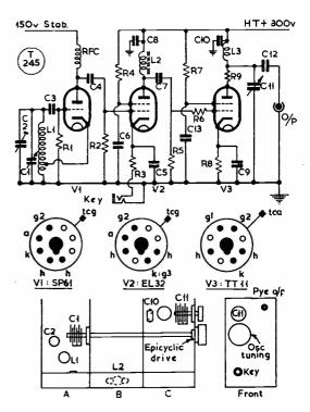
Circuit and layout used by G3IWL for his conversion of the RF-24 as a driver for 10 metres. It is always worth having separate gear for Ten, as not many transmitters can be considered fully efficient over the whole range 3500-28000 kc.
