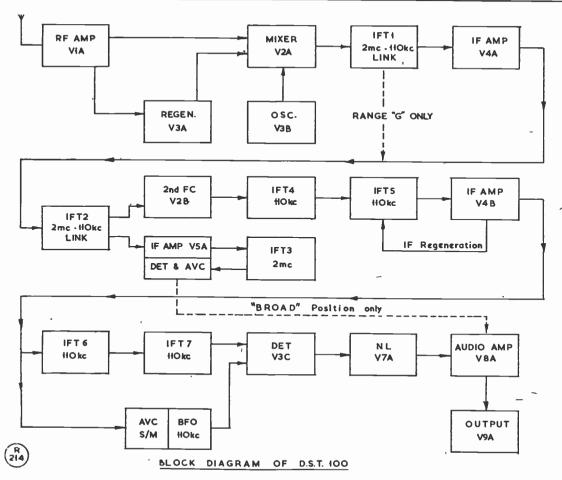
Block schematic of the ex-Army DST-100 receiver, which is a double-superhet (2mc/110 kc IF's) with a very wide tuning range — 50 kc to 30 mc, in seven switched bands. Thus, all six amateur bands in the HF range 1.3 to 28 mc are covered. A good specimen of the DST-100 is capable of a very adequate performance up to about 20 mc. The receiver is not self-powered.
