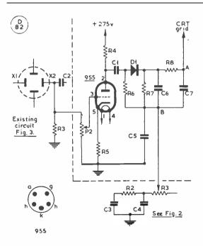
Fig. 7. The talk-brightening circuit devised by 4S7MG. When correctly set up, the trace disappears between words and on carrier only, thus guarding against burning of the tube by the stationary spot — see text for discussion. The only additional values involved are given in the table.
