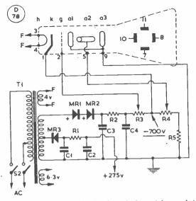
Fig. 2. Power circuit wiring for the cathode ray tube — using either a VCR-139A or a Cossor 23D — in the modulation monitor unit.
