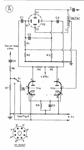
Fig. 3. Applying the audio to the X-plates; there is another way of doing this, as shown in Fig. 7.
