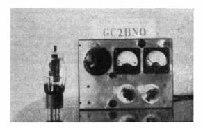
G2HNO's miniature portable Top Band CW/Phone transmitter — with an 807 alongside for size comparison. Acutal dimensions overall are 8ins. by 6ins. by 4ins. and the circuit arrangement is VFO 6AM6, VR159.30 stabiliser, and PA 5763, with a 12AX7-6V6 Clamp modulator. The meters are for plate current and RF loading. Some 190 contacts were made with this transmitter when signing GCEHNO from the Island of Alderney recently.
