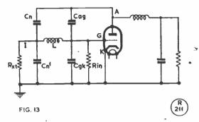
Fig. 13. Circuit arrangement for the bridge-neutralised IF stage in G3HBW's 23-centimetre converter.
