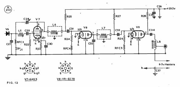
Fig. 12. The IF head-amplifier developed by G3HBW for his 23-centimetre converter; C36 and C37 are feed-through type condensers Circuit values and coil data are given in the tables.
