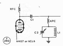
Fig. 3. An effective parasitic-suppression circuit, with the suppressor inductance on the tank instead of at the anode of the valve. APC is 5 turns of 14g.,  $\frac{1}{2}$ -in. diam. by 1-in. long; C1 is .001  $\mu F$ ; C2, L1 is the normal tuned circuit; and RFC a 2.5 mH RF choke.
