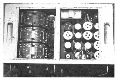
General appearance inside the DST-100, with the massive seven-band coil turret on the left. The compartment on the right is the IF chassis, the receiver being a double superhet with a total of no less than seven IF circuits. In this particular receiver, our contributor has fitted a "magic eye" tuning indicator (shown at centre of the right-hand compartment) in place of the panel light.
