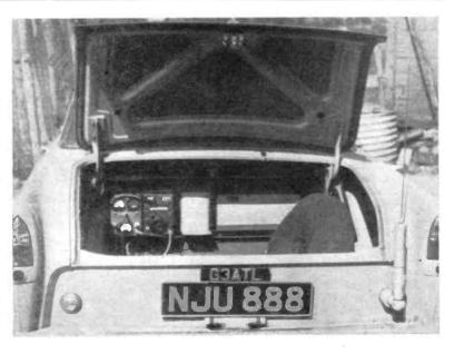
Equipment assembly for mobile working, fitted in the boot of G3ATL's car. Many hundreds of /M contacts have been made on Top Band and Eighty.
