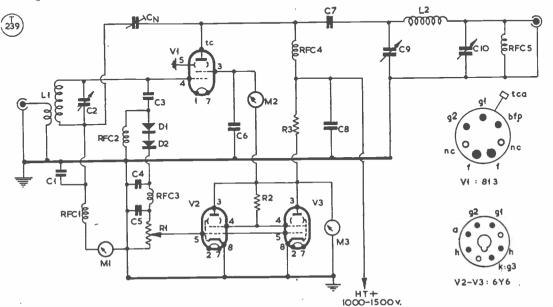
Fig. 2. The linear RF amplifier arrangement suggested by G2MA, and discussed this month. It is found to give very good results, with high efficiency. The action of the circuit is explained in the text, and values are shown in the table.
