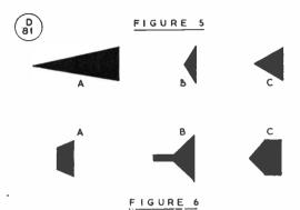
Fig. 5. Adjusting the horizontal deflection, R8 in Fig. 4, for correct patterning — 5C is the desired shape for a transmitter modulating 100%. Fig. 6. Showing the sort of patterns that may be obtained when the transmitter is not modulating correctly.
