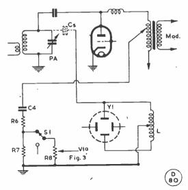
Fig. 4. Basic connections for the modulation monitor circuit — see text, and refer Fig. 7. Values here are as given for Fig. 3.
