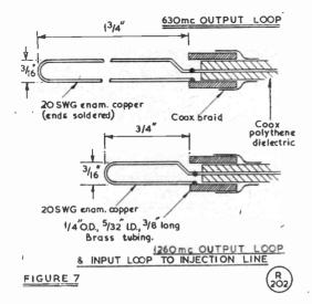
Fig. 7. The oscillator coupling loops, showing all constructional details.
