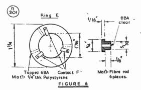
Fig. 6. Cathode contact ring and insulating bushes for the 446A—and see text.
