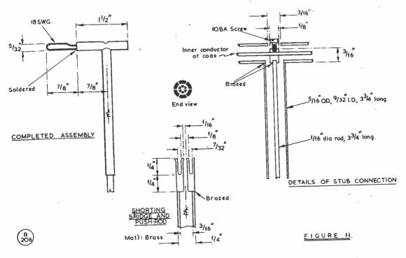
Fig. 11. Detail of the aerial matching stub and variable coupling loop.
