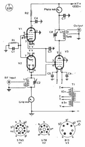
Fig. 2. Grid controlled Linear RF Amplifier in operation at GW2DUR, the action of which is explained in the text. In this case, the PA stage runs an 813. Values are given in the table.
