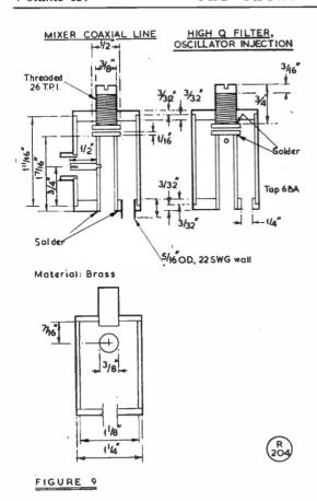
Fig. 9. Detail of the circuit arrangement shown in Fig. 8.
