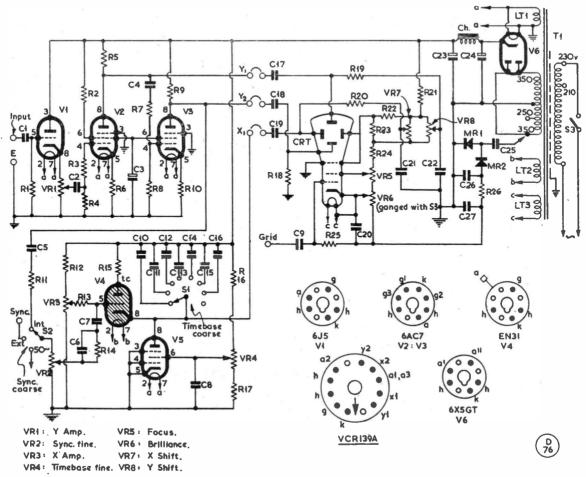
Circuit of the Oscilloscope complete, all values being given in the table. The design incorporates such refinements as are necessary for practical work on the bench, and the circuit can be put together from readily available parts. Note that the base connections for the 6SK7, V5, are the same as for the 6AC7, used at V2 and V3. At position 8 of the time-base switch S1, stray capacity is relied upon for this highest-frequency range.
