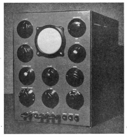
General appearance of the Oscilloscope described in the article. It is designed as a general-purpose bench testing instrument. For the model, overall dimensions are 11½ ins. high by 8½ ins. wide by 12 ins. deep, but any suitable cabinet size could be used.
