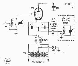
Fig. 1. The cathode follower Linear RF Amplifier used by DL4WM, and discussed in the text. It will work with any tetrode or pentode.
