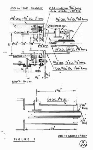
Fig. 5. Mounting (sectional view) for the 446A doubler and tripler valves. The circuitry was given at Fig. 4 on p. 662 of the February issue.
