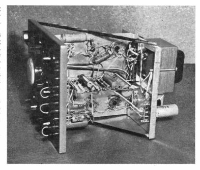
The construction underside of the Oscilloscope. The transformer is a home-made item, for which the necessary details are given in the text. It can, of course, be substituted by any commercial product providing the required outputs.
