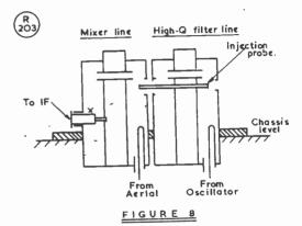
Fig. 8. The shunt-injection mixer arrangement, with the crystal tapped in about half-way down the signal frequency line—see Fig. 9 for further details.
