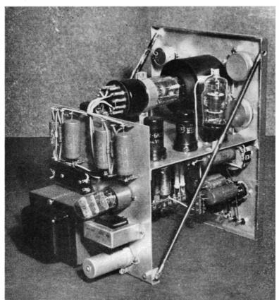
Half-rear view of the Oscilloscope, showing construction round the tube, a VCR139A.
