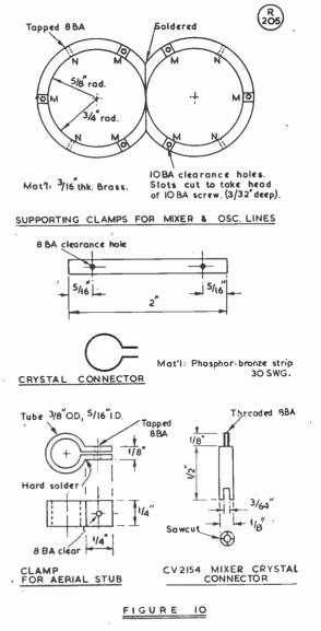
Fig. 10. Connectors and clamp for the mixer and oscillator lines, and the CV-2154 crystal mounting.
