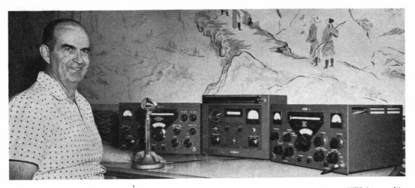
When W6ITH signs FS7RT and PJ2MC on his visits to the Island of Saint Marten (French and Dutch) he has a KWS-1 transmitter, SC-101 station control unit and 75A-4 receiver, all of Collins manufacture. The SC-101, centred in this photograph, contains speaker, aerial matching and switching controls, beam direction indicator — and a clock. Murais by the XYL.
