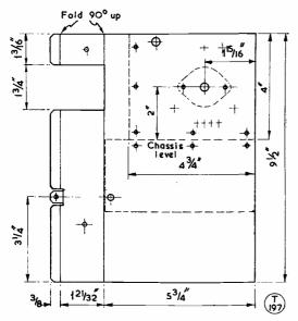
Fig. 3. The large dividing screen, as viewed from the VFO side with the transmitter inverted.
