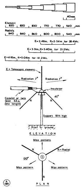
General arrangement of the ground plane transmitting aerial system described by HB9OP. Dimensions are given in metres and millimetres (one metre = 39.4 inches) and from the data, either a multi-band or a single-band ground plane can be designed. As explained in the text, it is essential to make the radial angle with the horizontal  $45^\circ$ . With a 120° plan angle between them, some control over directivity is possible, as shown by the "max. pattern" indication — and see text.
