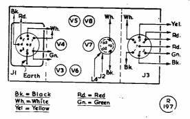
Fig. 2. Guide sketch to the general component layout, under chassis. This will enable the various items involved in the modification to be located.
