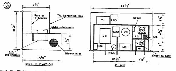
Fig. 2. Simplified drawings showing general arrangement of the chassis and screening compartments, with dimensions, and the placing of main parts. The upper screening box is from a TU unit and the chassis is made from heavy-gauge aluminium. The VI compartment also serves as a screening box for meter M1.
