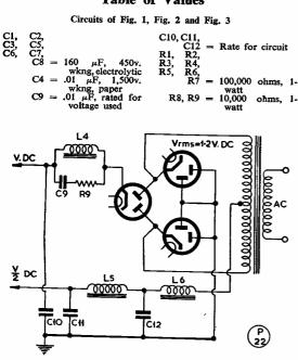
Fig. 3. With this arrangement three full-wave rectifier valves will give two voltage outputs at different current loadings from the one transformer.
