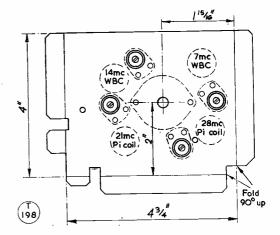
Fig. 4. Under chassis screen seen from the VFO with the transmitter inverted. The components are mounted on the reverse side.
