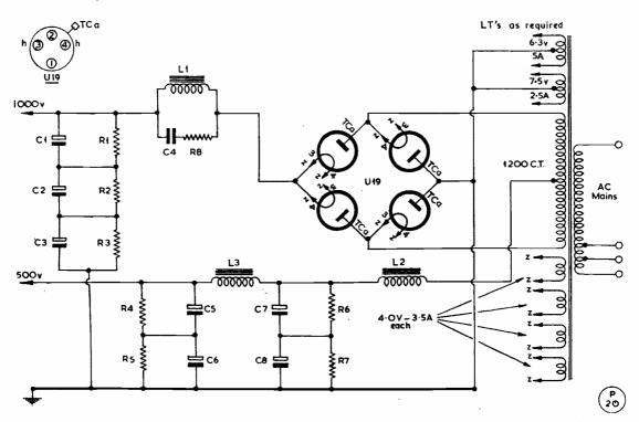
Fig. 1. The two-voltage HT supply circuit designed by The General Electric Co., Ltd., and described in the article. The system permits the use of one HV transformer to obtain two voltage outputs.
