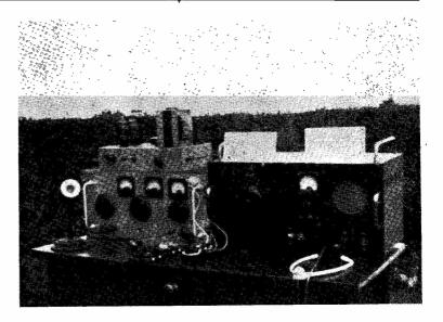
Top Band gear used by G3IDF/G3IDG on their GW/A foray into Anglesey during August 4-20 last. The CO-PA transmitter ran an EF91 into a QVO4-7, the speech side consisting of EF37A-EF37A-EL33 with a moving coil microphone; the receiver was a modified R.103 and two end-fed aerials were used, one 400ft. long and the other 175ft.
