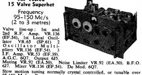
Slow motion tuning normally crystal controlled, or tunable over 95-150 Mc/s. Power supply required : 240-250 volts at 80 mA. 6.3 volts at 4 amps. Size  $19^{\prime\prime}$  x  $10^{\prime\prime}$  x  $10^{\prime\prime}$ . Standard Rack Mounting.
