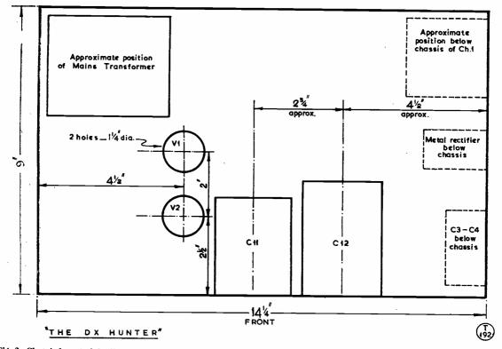
Fig. 2. Chassis layout of the "DX-Hunter." The metal-work can be supplied to this design by Philpotts, Loughborough, to match the "DX-Pilot" Exciter.
