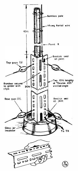
Fig. 1. General arrangement of the vertical Top Band aerial as evolved by the writer. It is not actually necessary to use "Dexion 225," nor a bamboo end-section to support the last ten feet. Any 25-40 ft. vertical tube, copperised metal mast, or just a wire hung from the highest available support, will do. In any event, the same principles apply.
