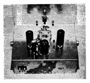
Top chassis view of the 10-metre converter, as constructed by G3WS. It is capable of giving very good results with any receiver tuning around 3 mc, which is the IF used. One of the valves shown is a stabiliser, V3 in the circuit.
