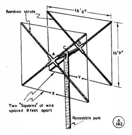
Fig. 1. Layout of the two-band Cubical Quad used by G3FXB. A boom A-B is secured to a pole at balance-point C, the pole being rotatable, through 180°, for directivity. The feed points for the two sections, which are both driven, are at X and Y. The arrangement of the feed line and matching stub is shown in Fig. 2.
