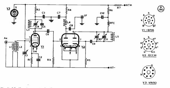
Circuit of the 10-metre converter described by G3WS. It is a tuned oscillator arrangement (C11), with L4 adjusted to a quiet spot near 3 mc. A unit of this sort will bring the 28 mc band on to any receiver which either does not tune Ten, or has an inferior performance on that band.
