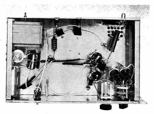
Nothing terrifying in the under-chassis construction of the "DX-Hunter." The three-band switched grid assembly is lower right and the small screen AF choke Ch.1 upper left; beneath the latter, up against the left-hand chassis drop, is mounted the Brimar DRM1B metal rectifier for bias supply. The phone/CW switch S3 is at left on the front chassis drop.
