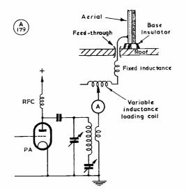
Fig. 2. Electrical layout of the 160-metre radiating system described by G5RZ. The effectiveness of the whole arrangement depends upon the correct adjustment of the loading coll, the object being to obtain maximum indication in the RF ammeter. Any similar electrical arrangement will work just as well, and the two inductances can be combined as one.
