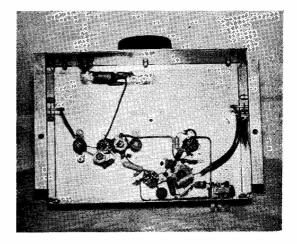
Under-chassis layout of the 10-metre converter. Wiring is quite straightforward.
