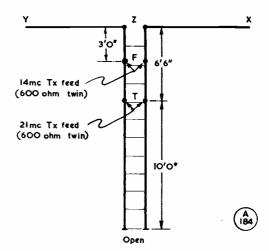
Fig. 3. Dimensions of the matching stub and position of the feed point for the 15- and 20-metre bands; the lettering corresponds to the layout shown in Fig. 2.
