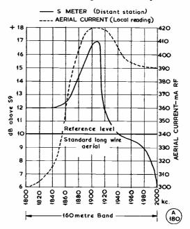
Fig. 3. Curves plotted under practical test conditions, in cooperation with a distant station at 15 miles. This curve was taken without any top loading capacity ("capacity hat"). The bandwidth for VFO operation would be good enough for all practical purposes over the range 1880-1920 kc, with th system resonated at 1900 kc. (In this presentation, the vertic scale above the reference level has been exaggerated for clarity.)
