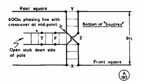
Fig. 2. The inter-connection arrangement between the two loops of the Cubical Quad; a feed line of 14 SWG spaced 2 inches is used. This sketch should be studied with Fig. 3.
