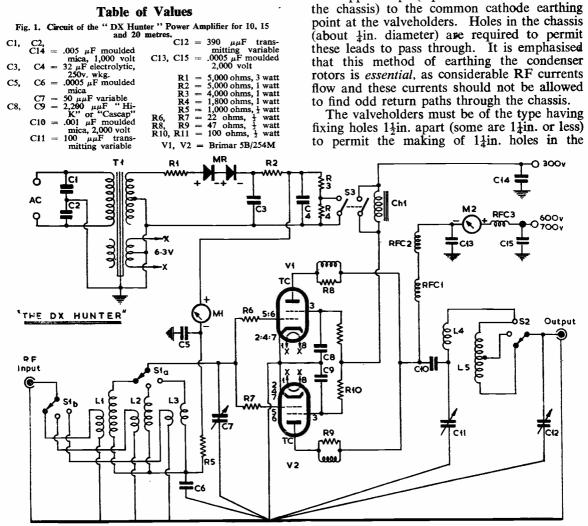
Fig. 1. Circuit of the "DX-Hunter," which is the PA unit for operation with our "DX-Pilot," as described in detail in the May issue of "Short Wave Magazine." This PA uses modern valve types (the Brimar 5B/254M, which is a miniature 807), and is band-switched to correspond with the three HF DX bands covered by the "DX-Pilot." Full constructional details are given in the article. (Note: The resistor above RIO should be marked RII in the circuit)
