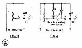
Fig. 3. Receiver muting circuit, explained in the text. Fig. 4. Circuit for BK operation, incorporating receiver muting .... see text for discussion.
