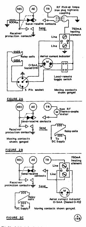
Fig. 2A : Original circuit of the American "Antenna Tuning Unit" Type CCT 29125. Fig. 2B : Modified circuit of the Type CCT, with new thermo-couple type RF meter. Fig. 2C : A suggested circuit for the Type CCT if the RF meter and thermo-couple as originally fitted are undamaged.
