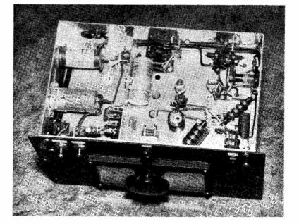
Under view of the VFO described by G3CNM, showing general layout. The small condenser in the centre foreground is C4, the control for close frequency shift. The power supply section is at the left, separated from the rest of the assembly by a screen.
