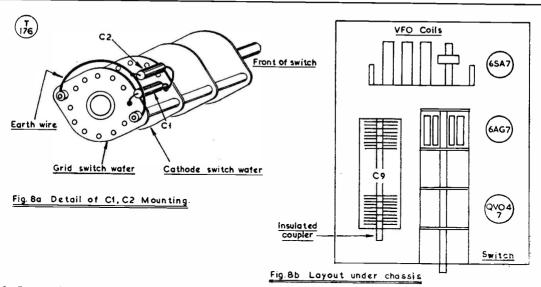
Fig. 8. Some main constructional details as discussed in the text, which will be helpful for planning layout. There is no need to follow this exactly — though it will probably be found convenient to do so — for, as the author himself points out, the idea is to suggest a line of approach, rather than a cast-iron mechanical design.
