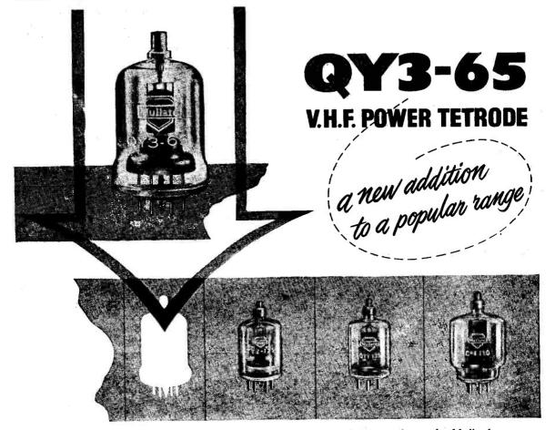
This new tetrode, the QY3-65, embodies a similar technique and construction to the Mullard range of all-glass transmitting valves which are already well established in communications and industry. It has an anode dissipation of 65 watts and a maximum frequency of 250 Mc/s and is directly interchangeable with the American 4-65A.
