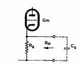
Fig. 2. The pass-band of the cathode follower is determined by the cathode load Rk - see text for discussion.
