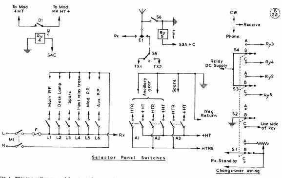
Fig. 6. This is a rather more elaborate station control system than that suggested in Fig. 2, and should be read in conjunction with Fig. 5. The switching sequences are explained in the article. As readers will appreciate, many variations of these layouts are possible to meet individual requirements. At many stations, the switching is built up piecemeal, as dictated by circumstances. Our contributor explains why it is better to work to a planned layout from the outset.
