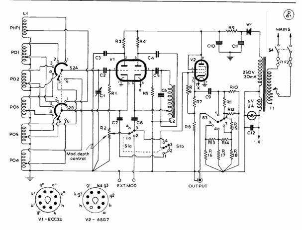
Circuit of the simplified signal generator described in the accompanying article. As our contributor explains, as a test instrument it can be rated as coming mid-way between the laboratory type of signal generator and a well-built and carefully calibrated GDO. Most receiver adjustments can be carried out with the instrument as described here, and it would be an extremely useful adjunct to the test gear at any station.
