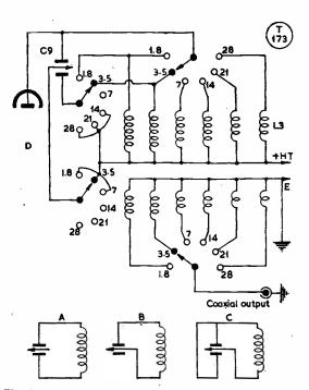
Fig. 5. Amplifier tank switching system, showing (below) how the double section condenser is used on various bands; in A, it is as a split stator on 14, 21, and 28 mc, 37.5  $\mu\mu$ F; on 7 mc, B, one stator/rotor section only is used, glving 75  $\mu\mu$ F maximum capacity; on 3.5 and 1.8 mc, C, the stators are in parallel, equal to 150  $\mu\mu$ F. Three wafers are used for L2/C8 (not shown), and 4 wafers for C9/L3, with L4.
