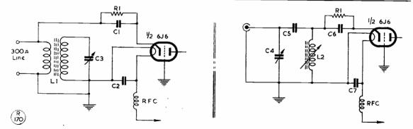
Fig. 2. Alternative input circuits for the grounded-grid 6J6, depending upon the aerial feeder to be used. Values are given in the table.
