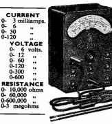
A conveniently compact 21-inch moving coil precision meter for making D.C. measurements of milliamps, volts and ohms. The total resistance of the meter is 100,000 ohms, and full scale deflection of 300 v. or 600 v. is obtained for a current consumption of 3mA. or 6mA. respectively
