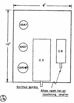
Fig. 7. Upper chassis layout for main items. As suggested by the author, if a sequence is followed in construction, it will make things easier.
