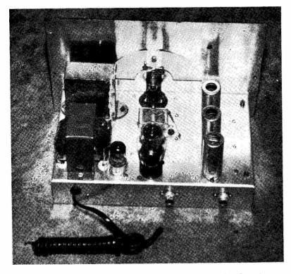
The power supply components are at the left, the valves in cans being, from the pane towards the near edge of the chassis : V1, the oscillator stage; V2, the buffer; and V3, the cathode follower output stage.
