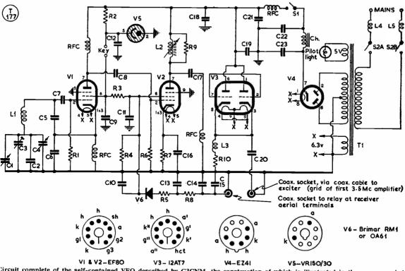
Circuit complete of the self-contained VFO described by G3CNM, the construction of which is illustrated in the accompanying photographs. That part of the circuit identified by V6, R5, R8, Cl3, Cl4, Cl5 is to control a relay to follow the keying ; this could be arranged to perform all change-over functions, while permitting BK operation. In the author's case, the relay mutes the receiver. All values are given in the table.
