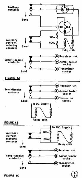
Fig. 1A: Original circuit of the Switch Unit Type G. Fig. 1B: Modified send-receive wiring, Type G. Fig. iC: Wiring for send-receive and current reducing contacts, with all remaining sockets and contacts removed. The action of the Type 78A relay is very similar to the above, and it also has provision for manual control. (This is the knob protruding from the case, seen in the photograph.)
