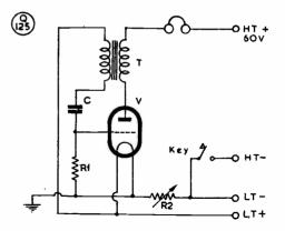
Fig. 7. A simple audio oscillator for Morse sending practice. The key is in the —HT lead and the pitch of the note can be adjusted by variation of the RI and C values. This oscillator will go off on HT as low as 9v. from a bias battery. Any diffi-culty in getting it to work is usually because the connections to the transformer are in the wrong sense. If audio oscillation cannot be obtained when the circuit is first set up, the leads on one side of T should be reversed.
