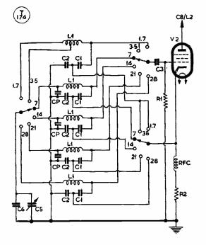
Fig. 6. Oscillator switching layout, with coil values in the table—and see text for discussion.
