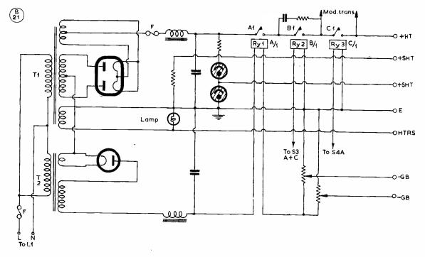
Fig. 5. Typical power-supply unit, incorporating a bias pack and relay control from the main switching layout shown in Fig. 6. The salient features of this arrangement are discussed in the text. For the relays Ry1, Ry2, Ry3, the P.O. 600 or 3000 types would be suitable.
