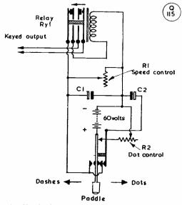
Fig. 1. Circuit of the auto-key described by G3IIH. Using no valves, it is easily put together; the secret of success lies in the adjustment — see text.
