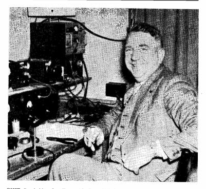
G3IIT, Cambridge, first licensed in June, 1952, has been operating exclusively on two metres ever since. All his gear is home-built except the BC-454 used as IF/AF strip. The converter is RF 6AK5 into 6AK5 mixer, CO 6C4-12AT7 multiplier, and the IF range tuned is 3.4-5.4 mc. The transmitter consists of CO EL91-QVO4/7 doubler-QVO4/7 doubler-832 PA and the modulator is 6SJ7-6SL7 into p/p 6V6's. The beam is four stacked Skeleton Slots.
