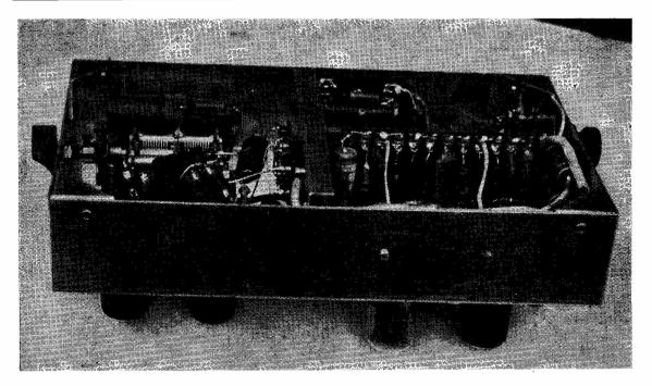
Under-chassis view of the G3GEN SSB modulator. On the left of the central screen are the balanced modulators, V3 and V4 in Fig. 2, with the tuned circuit of L1 at the rear. In the centre of the right-hand section can be seen the group board carrying the twelve audio phase-shift networks.
