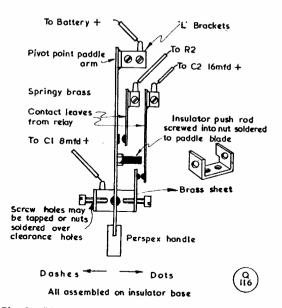
Fig. 2. Electro-mechanical assembly of the auto-key. It should be mounted on a firm, insulating base; if this base is heavy enough and is fitted with rubber feet, the key can be made non-slip in operation.
