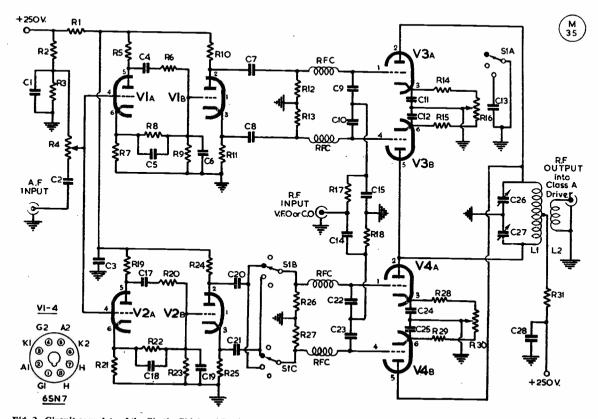
Fig. 2. Circuit complete of the Single-Sideband Exciter described by G3GEN and based upon a standard design. It is of the phasing type, with low-level balanced modulators. The switching provides for A3 (AM phone) carrier when required. Note that the top end of C13 should go to the junction of R14, R16, and that the switching is shown in Posn. 3 of the 4-way switch S1A-S1C.
