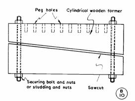
Sectional view of the wooden mandrel which can be made, as described in the text, for the winding of self-supporting transmitter coils. The mandrel collapses by taking out the securing bolts and can then be withdrawn easily after the coil has been formed. Other methods of coil construction are suggested in the text.
