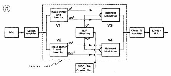
Fig. 1. Block schematic, showing the SSB Exciter in a typical transmitter chain.
