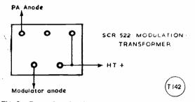
Fig. 3. Connections for the modulation transformer in the G3FRV transmitter with an SCR-522 mod. xformer. When a Woden UM1 is used details are: Strap 3/4, 9/10; take HT + to 5/11 strapped; 6V6 anode to 2; QVO4-7 anode to 8.
