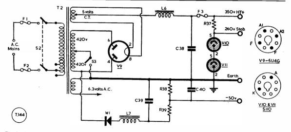
Fig. 5. A suitable power pack, as a separate unit, for the Top Bander designed by G3FRV. All values are given in the table.
