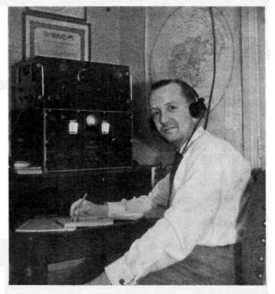
PAOVD, Rotterdam, is ex-PK4VD (1947-'48) and now has a neat living-room layout running, as he says, "moderate power." The transmitter is EF50-EF50-6V6-807, covering 3.5, 7 and 14 mc, but operated mainly on 40-metre CW; the power supply is on the same chassis as the transmitter, the whole of this part of the assembly being in a BC-348 cabinet. Receiver is an HQ-120 and the aerial a 7 mc doublet. Some 55C have been worked post-war on Forty.
