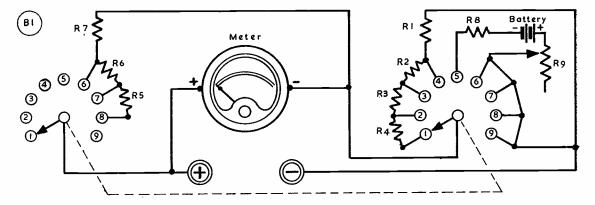
Circuit of the DC Test Meter constructed for the essential measurements. It is easy to put together, cheap to build and will be found indispensable once you have it! The photograph shows the way in which this particular model was actually built; other forms could be adopted, provided the general principles are followed—remember, too, that the 0-1 mA meter must be a good one if the readings are to be reliable and consistent. F1, F2 in the Table of Values is the ganged switch.
