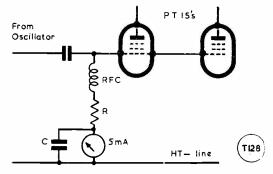
Fig. 1. The grid side of the parallel-PT15's PA, as modified by G3EGC; C is .01  $\mu F$ , and R 20,000 ohms. The RF choke and grid meter are additional items and the modification as a whole results in a worth-while improvement on the RF side.
