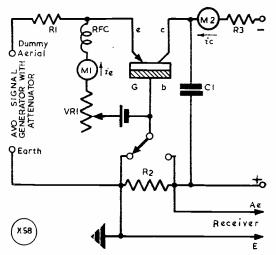
Fig. 3. A complete circuit as in Fig. 2, with the addition of bias. As explained in the text, with this set-up the variation of "alpha" against frequency can be determined to a degree of accuracy sufficient for most practical purposes.
