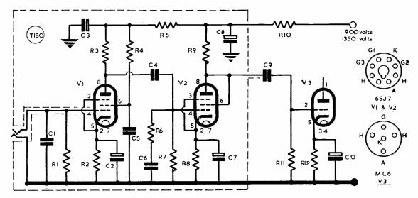
Fig. 3. Circuit of the two-valve speech amplifier incorporated in his T.1154 modulator circuit by G3EGC. V1, V2, are the new stages, for which values are given in the table, and V3 is the ML6 modulator as fitted in the original. The results on phone are greatly improved by this modification.
