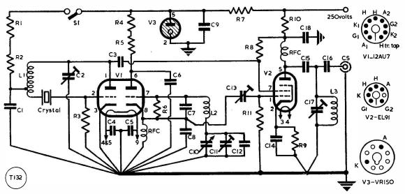
Fig. 2. Circuit of the VHF VFO designed and described by G3FYY in his article. The degree of stability attained, and the freedom from drift after warm-up, makes it entirely acceptable as a driver unit on two metres. The variable oscillator is around 4 mc and the crystal output frequency about 20 mc; the mixed (24 mc) output is multiplied up in the usual way and, with a good dial on C10, accurate frequency setting in the 144 mc band can easily be obtained.
