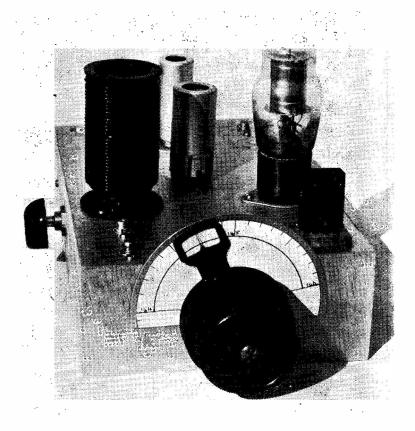
The VHF-VFO complete, as described by G3FYY. Full coverage of the two-metre band is obtained, with ample drive output into the existing 24 mc stage in the transmitter. The large valve on the right is a voltage stabiliser for the Clapp variable oscillator. Mixed frequencies are: Crystal, 20 mc; variable oscillator, 4 mc.
