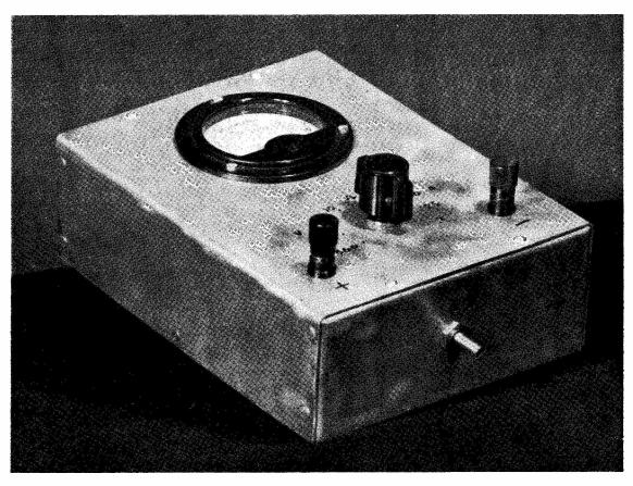
General appearance of the DC Test Meter described in the article. It covers the voltage-current ranges met with under practical conditions and will also measure resistance. The heart of the instrument is the 0-1 mA moving coil milliammeter. The text gives you full details for construction and calibration. The slotted spindle on the front drop is for screw-driver adjustment of resistor R9.
