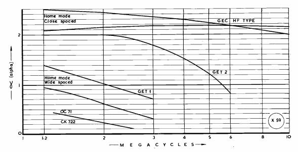
Fig. 4. These curves show typical results obtained with the apparatus shown in Fig. 3. It will be seen that a very clear indication is given by the method described, and that as "alpha" begins to drop with frequency, it falls off fairly rapidly.
