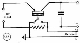
Fig. 2. Outline of a practical circuit based on the principle of Fig. 1 showing how one resistor, of about 100 ohms, can be used both on input and output sides by switching in the base.
