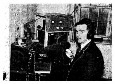
GI3HJA, Omagh, Co. Tyrone, is mainly on 80-metre phone with paralleled 1625's in the PA, modulated by a pair of 807's. The transmitter is band-switched for 80 to 10 metres, and it is hoped to get on 160 metres when a suitable receiver is obtained—at present it is an unmodified R.1155. The aerial is a 132-foot end-fed wire.
