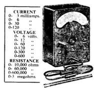
A conveniently compact  $2\frac{1}{2}$ -inch moving coil precision meter for making D.C. measurements of milliamps, volts and ohms. The total resistance of the meter is 100,000 ohms, and full scale deflection of 300 v. or 600 v. is obtained for a current consumption of 3mA. or 6mA. respectively
