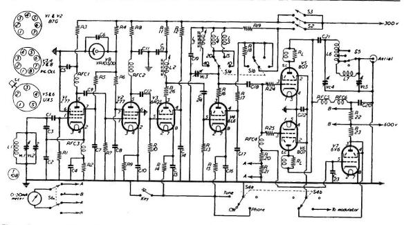
Fig. 1. Circuit of the RF section of the VQ2AH transmitter as described. The driver section V1, V2, V3 can be built and tested as a separate unit before fitting to the main chassis. The switched coils in the plate of V4 give output on three HF bands, operation of the PA on 10 metres being obtained by doubling from the 20-metre drive at L4. The 807's in the PA are in parallel and modulation is by screen control.
