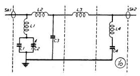
Fig. 1. Circuit of the filter suggested by G8PG. Values are: C1, 100  $\mu\mu$ F silver mica; C2, 50  $\mu\mu$ F air trimmer; C3, 440  $\mu\mu$ F, silver mica; C4, 120  $\mu\mu$ F, silver mica; L1, L4, 13 turns spaced 1-3 ins.; L1, L3, 20 turns spaced 2 ins.; all colls are  $\frac{1}{2}$ -in. diameter. Sk1, Sk2, are coax sockets.
