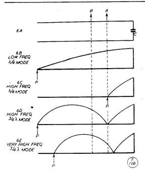
Fig. 6. Showing how quarter-wave and three-quarter wave modes of oscillation can be obtained over the same pair of lines. As explained in the text, this is one of the most important attributes of the concentric line principle.
