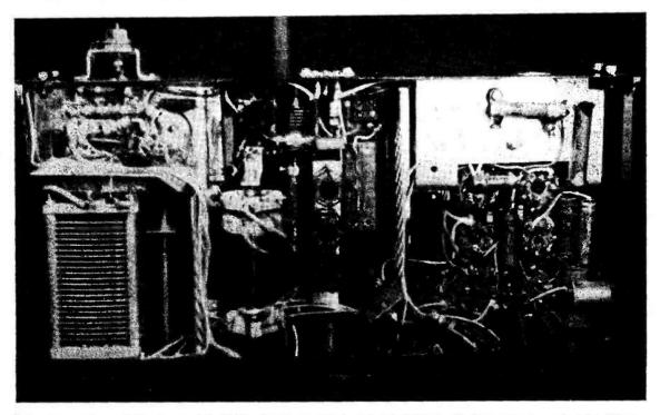
General view underneath the chassis of the HF Band Table-Topper described by VQ2AH. The big condenser on the left is VC5 (see Fig. 1), with coax RF output connection above, on the rear apron. The grid side of the PA section is immediately below this and the coil assembly L3, L4, L5 can be seen at centre, with the switching S1a-S1b alongside at left. The wiring associated with the modulator is over to the right.
