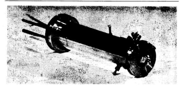
The 1215 mc oscillator complete, seven inches in length, as designed and constructed by G5RZ and described in the article. The coaxial line tuning technique is what makes the dimensions manageable at this (relatively) very high frequency. The unit can be operated either as oscillator or amplifier and will give about two watts of measurable and controllable RF output, with reasonable stability.
