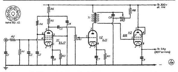
Fig. 2. Screen-control modulator unit for the VQ2AH transmitter. This arrangement will give full modulation of a 70-watt carrier, with good quality speech and easy adjustment, provided the screen voltage of the 807 PA, controlled by VR2, is correctly set.
