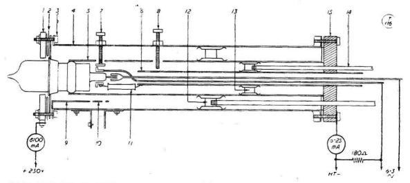
Fig. 5A. Detail of the 25-centimetre oscillator designed by G5RZ and illustrated in the photographs. This is a section ("cut in half down the centre") showing both the mechanical arrangement and the electrical layout and connections for details, and refer exploded view photograph.
