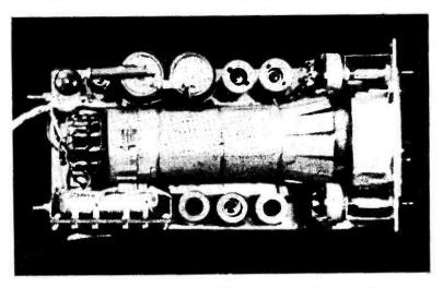
Plan view of the Oscilloscope, showing that space is not wasted. The drawings to follow should be consulted for the mechanical details.
