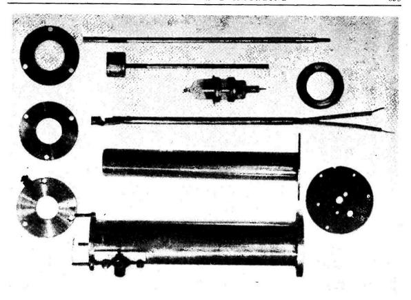
All the parts for the 25-centimetre oscillator, which make up to the assembly shown in the accompanying photograph. It is a Mullard TD03-10 (ME-1000) and a detail drawing of the oscillator appears in Fig. 5A.
