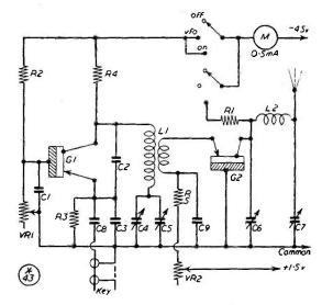
Fig. 3. VFO-PA transistor transmitter now in use at G3CSZ, of which details are given in the text. He uses the VFO circuit suggested by G3CGA, while the PA arrangement is that devised by G3HMO. The result is a handy, stable TTX for 160-metre working; in G3CSZ's case, the transistors are home-made but GET-2's could very well be used.
