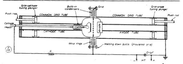
Fig. 5. The basic coaxial or concentric-line oscillator circuit as a logical development of Fig. 3. This is a sketch of the electromechanical arrangement, in section, the actual construction being cylindrical.
