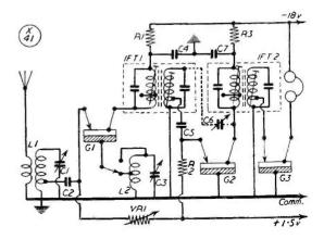
Fig. 1. This simple superhet circuit employs only three transistors. The signal is injected into the emitter of a base-tuned oscillator and the resulting IF taken from the collector. Feedback in the IF stage increases sensitivity and makes CW reception possible. The last transistor detects and amplifies, the output being taken on phones. This is an experimental circuit, which has been tried on the 160-metre band with very encouraging results.
