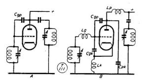
Fig. 1. (A) shows the basic circuit of the conventional TPTG oscillator. At (B) is the TPTG as it appears at VHF, showing the effect of lead inductance, inter-electrode and stray capacities.
