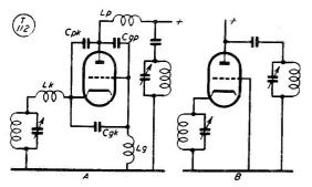
Fig. 2. (A) The common-grid circuit drawn to conform with Fig. 1 (B). (B above) The common-grid with the unwanted L and C components absorbed into their respective circuits. This is now the familiar grounded-grid arrangement.
