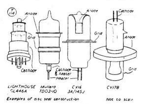
Fig. 4. Outline drawings (not to scale) of valve types designed for concentric line circuits at UHF.
