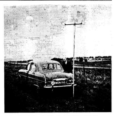
G2ATK (Shirley, Birmingham) is a well-known /PM operator on the two-metre band. For static working, the beam is a 3-ete knock-down Yagi; for operation on the move, a quarter-wave vertical, seen on the near side of the car, is used. G2ATK at the microphone, photograph taken by G3ABA. Nice site, too, by the look of it!
