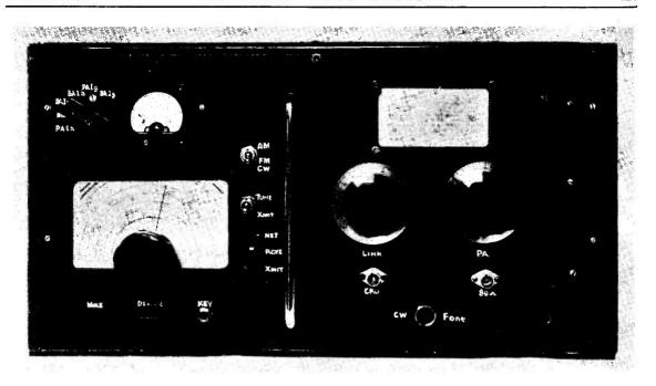
Panel appearance of the 160-metre CW/Phone transmitter described by G2NS. The VFO is on the left, and the dials on the right are for C14, C15 in the circuit, Fig. 1. Phone working can be either by plate-screen modulating the 807 PA, or by NBFM on the grid of the VFO.
