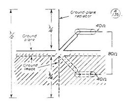
Fig. 1. The equivalent radiating system for the usual type of ground-plane aerial, which demands a low-impedance feed, sometimes awkward to achieve.
