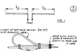
FIG 2 Balun impedance transformer for 145 mc
