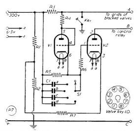
Fig. 1. Circuit of the control section in the change-over system discussed by G3EFI. VI, V2, can be a single 6SN7, one half V1 connected as a diode, or a separate triode and diode can be used. The unit requires a negative supply of about 300 volts.
