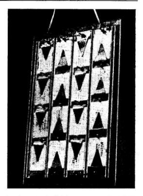
Rear view of the photo-cell battery constructed by G3HMO, shown as P in the circuit at Fig. 1. The triangular pieces are cut from springy brass sheet, set to give good contact with the back of each cell. The perspex sheet is about 8 ins. wide by 10 ins. deep, approximately the size of an ordinary window name.
