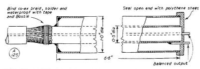
Fig. 7. Balun for 430 mc. The inner tube should be chosen to give a wall thickness making a tight fit over the polythene insulation of the cable used.
