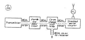
Fig. 4. Block schematic of the layout complete on the output side of the 160-metre transmitter—an arrangement contributing very largely to the elimination of BCI and TVI.
