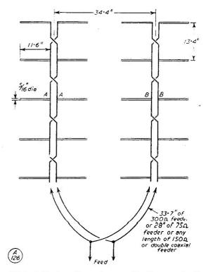
Fig. 8. A 20-element beam layout for the 430 mc band. It should be particularly noted that the correct feed points are at "A-A" and "B-B" and not at the bottom of the stacks.
