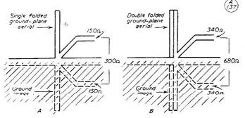
Fig. 2. Showing the equivalent radiating system for single and double-folded ground plane systems, with feed impedances.
