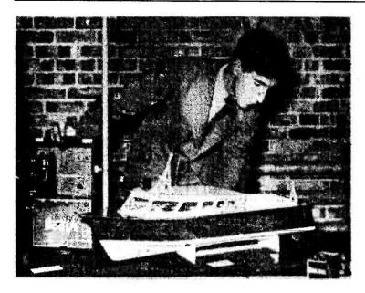
Displayed at the Hastings Hobbies Week exhibition was this radio-controlled launch, built by T. A. Curtis; the boat is powered by a 20-volt motor, and the control transmitter is a self-excited push-pull oscillator, with a quench receiver. The control motions give five steering settings, half-speed and stop.
