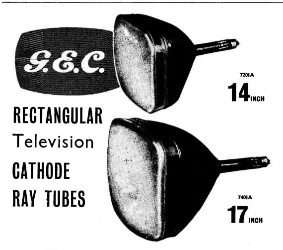
These G.E.C. television tubes combine all the requirements for perfect viewing. ALUMINISED SCREENS for brighter and more contrasty pictures with long life and freedom from screen burn. GREY FILTER GLASS faceplates with high light transmission efficiency permitting viewing under normal lighting conditions without loss of contrast and without need of separate viewing filters.
