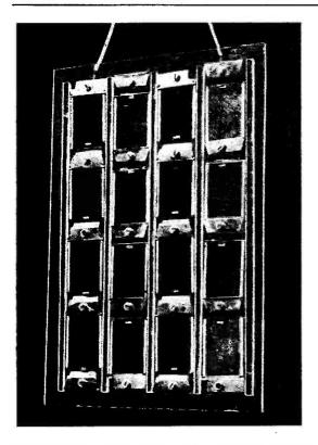
Front view of the selenium photo-cell assembly actually used for the sun-power transistor transmitter tests on Sunday, September 5. The cells are each about 1}-in. wide by 2-in. long and are individually mounted on a sheet of perspex, and series connected. The DC output in bright sunlight is 4-5 volts at about 3 mA, sufficient to run a good point-contact transistor at 12 mW input.
