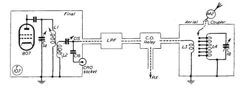
Fig. 4A. RF output feeder and aerial coupler, the latter enabling any normal length of end-on aerial to be energised. The adjustment is to get maximum reading in M2 at the correct PA input; this will involve finding the correct tap on L4 and resonating C18 at each adjustment. The coupling L1, L2, and the setting of C15 may also be affected as these changes are made. The general tune-up procedure is all-through adjustment from C14 to C18 for the best reading on M2.
