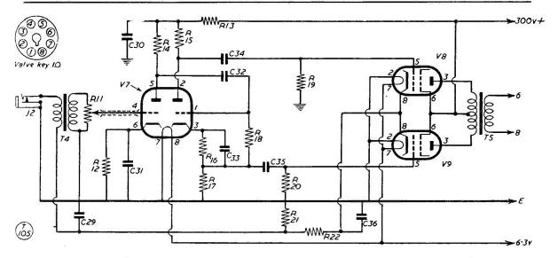
Fig. 3. A simple amplitude modulator for the 160-metre transmitter described in the article. This gives plate-and-screen control of the 807 PA. V7 is a 6SN7 and V8, V9, are 6V6; note how the energising current for the carbon microphone at J2, T4, is supplied by tapping off the cathodes of the 6V6's.
