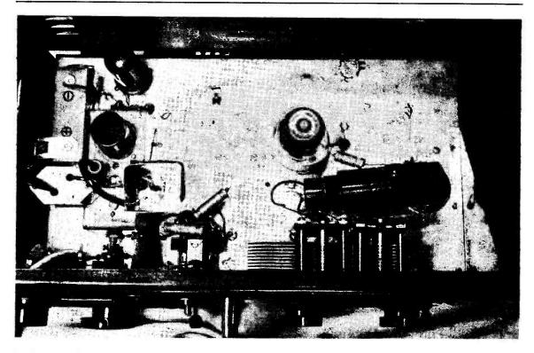
Interior view of the Safe Top Bander, with the PA section on the right. The coils L, L2, can be seen below the main tuning condensers C14, C15; this part of the circuit is normally enclosed in a shielding box. The VFO is on the left, with the buffer-stage valve immediately behind it. The frequency modulator section is mounted on the VFO, and connected to it by coax—see Fig. 1.
