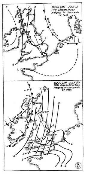
Fig. 1. On the two occasions shown here, reflection from layers at unusually high levels is thought to have occurred. On July 12 (above), the phenomenon coincided with an abnormally low value of surface pressure; on July 20, a double structure is shown over southern England.
