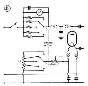
Fig. 2. In this circuit, rheostat No. 1 of Fig. 1. can be eliminated, and R3 is a calibrated 4-ohm resistor tapped at 1, 2, 3 and 4 ohms exactly. The circuit to the right of the valve is as fig. 1.
