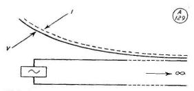
Fig. 2. Current and voltage distribution on an infinite line — see text for discussion.
