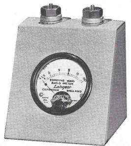
The "Labmatch" Standing Wave Ratio Meter provides instant indication of feeder matching.
