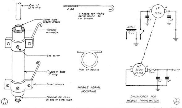
Details (left) of the whip aerial mounting; the centre tube is a piece off the butt end, forced into the length of rubber hose, which is then rasped down till it in turn is a tight fit in the 1-in. copper tube bolted to the humper. On the right is the electrical layout of the dynamotor power supply unit; condenser values are C1, C2, 0.1  $\mu$ F; C3, 0.1  $\mu$ F, 600v. working; C4, 30  $\mu$ F, 500v. working. No other smoothing is necessary. Note the HT fuse.
