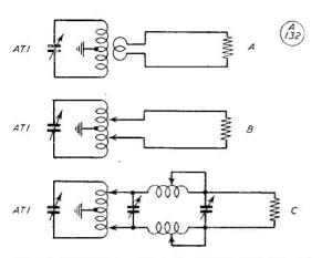
Fig. 5. Matching the tuned tank circuit into the transmission line, which is the immediate load on the tank.
