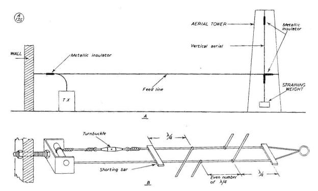
Fig. 8. (A) Single-line diagram to illustrate layout of strained feeder system. The quarter-wave metallic insulators, marked heavily in this sketch, are described in the text (B) is the detail of tensioning arrangements in a feeder system of this kind, using non-stretch wire such as cadmium-loaded copper.
