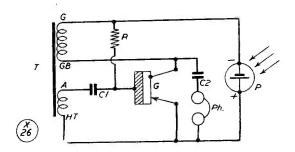
Fig. 1. An LF oscillator which works with ordinary daylight as the sole source of power! A strong audio note is heard when the photo-cell is exposed; if the p-e cell is shown to an electric lamp, the note can be heard with 50-cycle AC modulation superimposed. The "easy-oscillation" characteristic of the Mullard OC70 junction transistor is such that it will also go off on a cell consisting of wet blotting paper between a piece of aluminium foll and a penny.
