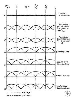
Fig. 3. This interesting diagram shows the relationship between voltage-current standing wave patterns and a variety of the terminations likely to be encountered.
