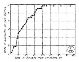
Fig. 2. This curve shows the drift against the warm-up time for the G6XH VHF-VFO as described. After 20 minutes, the frequency remains perfectly steady.
