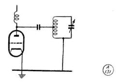
Fig. 4. Matching the PA valve into its own load, the tank circuit. A correct match can be obtained by tapping the anode connection down the tuned circuit.
