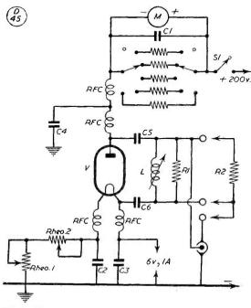
Fig. 1. The circuit suggested by DL2MW, of which Fig. 2. is a rather more elaborate version with a double-bank switch (see text). A noise generator is an extremely valuable piece of equipment for receiver comparison.
