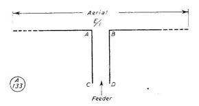
Fig. 6. The impedance at the feed point of a centre-fed aerial — see text.
