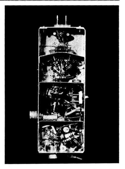
Layout and construction underneath the G5RZ converter, with the RF stage at the top. The various stages are in screened compartments, and the chassis overall is 9ins. long by 3\{\}ins. wide by I\{\}ins. deep.
