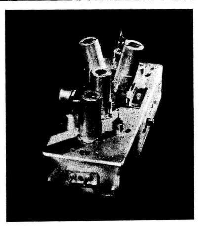
Top view of the G5RZ two-metre converter, from the aerial end. A neat and symmetrical layout, with the preamp-cathode follower stage in the turret mounting, and the oscillator—multiplier immediately behind.
