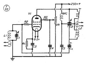
Fig. 1. Neutralised harmonic-free driver stage for the Class-AB1 RF amplifier.
