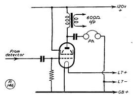
Fig. 1. The original circuit, on the LF side, of the R.1224A.
