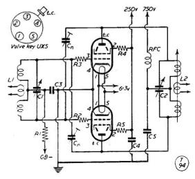
Fig. 2. Push-pull RF amplifier in Class-AB1, using 807's, which must be neutralised to ensure a clean signal. When adjusted in the manner explained in the article, there should be very little harmonic energy in the output, and even though RF power will be less than with more bias and harder drive, this will not noticeably affect results if the radiating system is efficient.
