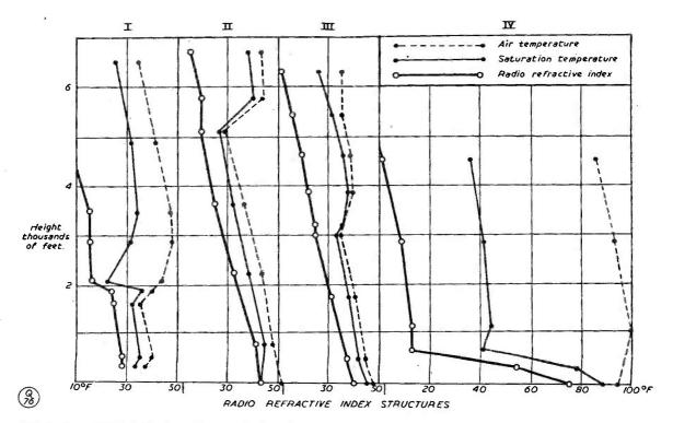
Fig. 3. As explained in the text, these graphs show how varied, from the radio view-point as well as for their effects upon our weather, warm fronts can be. Section IV shows intense duct conditions as experienced in the Middle East.
