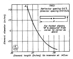
Fig. 2. Curve for the design of Yagi flat-tops, showing how the length for resonance at 145 mc decreases with the larger diameters for the element material.
