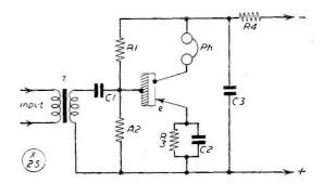
Fig. 3. Transistor audio amplifier, used as the LF stage with the 1-V-O TRX shown on p.283 of the July issue. The input is taken from where the phones are connected in that circuit, and the result is a "1-V-1" type of receiver which gives excellent results on the 160-metre band.
