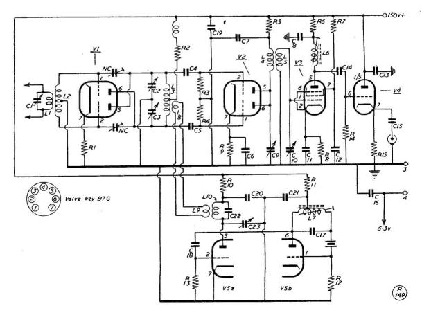
Circuit complete of the converter designed and described by G5RZ. It is quiet and sensitive, and being crystal controlled on the oscillator side, gives a T9 beat and is accurate for calibration over the IF tuning range. (Note: The winding above R2 is a VHF RF choke).
