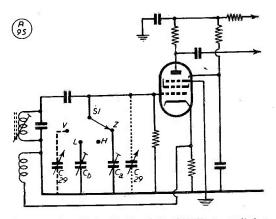
The BFO modification suggested by G3DXI as applied to an AR77; it is equally suitable for communication receivers of other types. In this arrangement, the cathode resistor does not act as a bias source, but determines the output of the oscillator. Ca, Cb are 3-2  $\mu\mu$ F trimmers, C29 dotted is the original BFO beat adjusting condenser, and C29 dashed, connected to S1, is of sufficient capacity to swing from 455 to 1000 kc.
