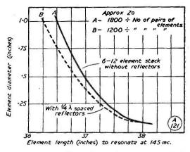
Fig. 1. Element length in inches against diameter of the element material for resonance at 145mc under (A) and (B) conditions as discussed in the text.
