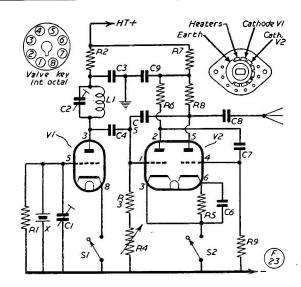
Circuit of the 1-megacycle CC marker oscillator, with the multiplier-amplifier stage V2 to give 100 kc beats all the way up into the HF bands. With such an arrangement it should be possible to find, for example, a well-defined heterodyne note at 14000, 14100, 14200 kc and so on, thus enabling VFO or receiver to be accurately calibrated.
