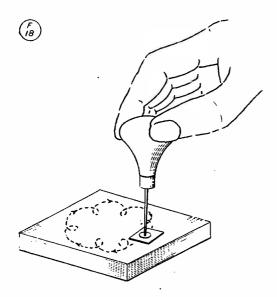
Fig. 2. Motion for crystal grinding. The crystal to be treated is under the brass pad.
