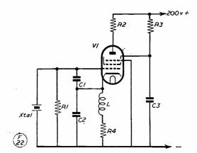
Fig. 6. This is the Pierce, a very useful general-purpose test oscillator which will go off with any active crystal.
