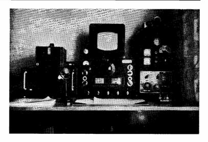
Station of GI3GTR, Whitehouse, Co. Antrim, first licensed in July 1950. The transmitter, says he, "is a much-modified G09 with straightforward circuitry and runs an unpretentious 25w. to an 807." Phone is by crystal microphone into a 65J7-6J5-p/p 6L6 modulator, the receiver is an HRO, and the aerial a 132-ft. long wire. Control is by relays throughout, operation is exclusively on 80 metres, CW and phone, and DX is never chased — though it is worked when it presents itself.
