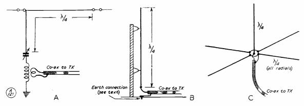
Fig. 1. Showing forms of what is known as the "Marconi Aerial." In (a) the total length of a quarter-wave is obtained by bringing the lower end in to the operating position and resonating by means of a series-tuned circuit; (b) A vertical quarter-wave, with a direct earth connection immediately under it, and coax feed from the transmitter (not using 72-ohm line, however); (c) The ground-plane is an elevated Marconi with horizontal radials taking the place of a direct earth connection.
