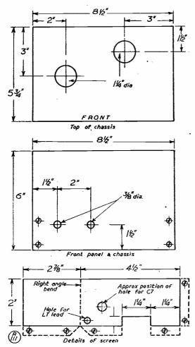
Fig. 2. Chassis drilling detail and sub-chassis screen for the two-stage preselector. The screen is fitted across V1, as indicated by Fig. 3.
