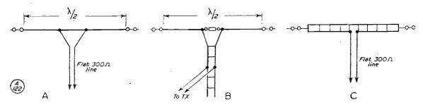
Fig. 2. Dipoles not fed with 72-ohm coaxial line. In (a) is shown the delta-match system, whereby a feeder of almost any impedance can be matched to the dipole; (b) Matching by means of an open stub suspended at the centre of a dipole; (c) The folded dipole, which gives an almost perfect match to 300-ohm feeders.
