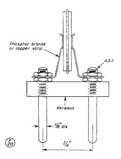
Fig. 4. A home-made experimental mount for the quick checking of processed crystals. For final calibration accuracy, the crystal must be checked in the holder and circuit in which it is to be finally used.
