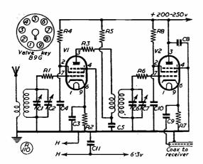
Fig. 1. Circuit of the two-stage preselector, for which full details are given in the text. It will considerably improve the performance of most receivers over the 14-28 mc bands.
