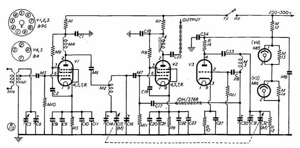
Circuit of the RF-27 Unit as modified for Two Metres. In this and the table of values circuit elements marked "M" are the modification items. Stabilisation of the oscillator V3 is very important for the best results. The existing IF section tuning can be adjusted on the slug for any frequency between 7 and 8 mc.
