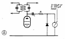
As explained in the text, with this S-meter circuit C should be made as low and R as high as possible consistent with the desired range of readings.
