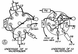
Fig. 3. Showing wiring around the valveholders (underchassis view) for best screening effect. The circuitry on the grid side of VI (Fig. 1) is fitted inside the screened compartment.
