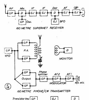
Block schematic of the transmitter and receiver arrangement at G3CCA, Leicester — using transistors and crystal diodes throughout, and possibly the first all-transistor station in the world. On the night of May 4-5, on the 160-metre band, G3CCA worked G6FO, nr. Buckingham, on the transistor transmitter and was able to receive phone from G6FO at R5 on the transistor superhet receiver; the distance is 45 miles.
