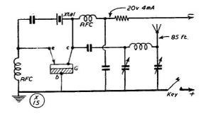
Fig. 1. Transistor circuit in use by G3IYX on 1822 kc, with an 85-foot aerial and Collins coupler; his input is 85 milliwatts and he radiates a very good local signal up to 10 miles or so, with a 28-mile reception report as best DX so far. G3IYX is regularly active from Bradwell in North Bucks and can be found on the air most evenings.
