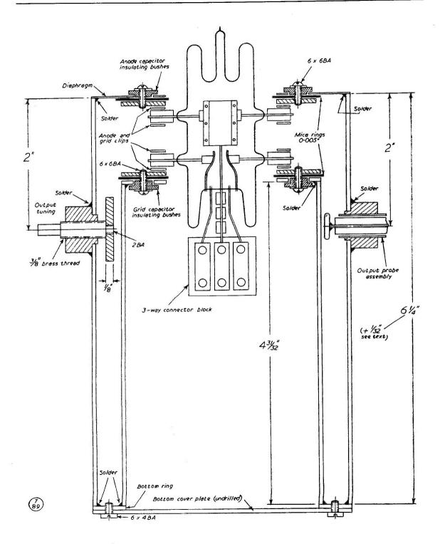
Fig. 2. Dimensioned cross-section through the 430 mc circuits in the G3HAZ 8012 tripler.
