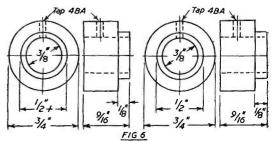
Output probe and output tuning capacitor bushes
