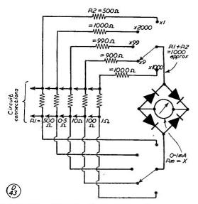
Fig. 4. With this arrangement AC current can be measured at five separate points in a circuit. As in Fig. 3, a 2-pole 5-way rotary switch can be used.
