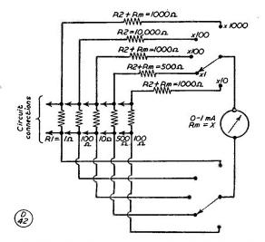
Fig. 3. Wiring layout for current measurement at five separate points in a circuit, the principle being the same as in Fig. 1. except that parallel resistors are involved. The switching motions can be carried out by a 2-pole 5-way rotary selector.
