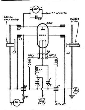
Fig. 1. Electrical cross-section through the 70-centimetre tripler, showing also the circuit arrangement. L1, C1, C2, comprise the 2-metre tuning assembly.
