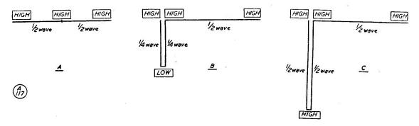
Fig. 1. Illustrating the well-known Zepp aerial system, familiar in amateur working. As shown at (b) and (c), the length of feeder affects the impedance to be matched, and hence the method of feeding, at the transmitter end. It will also be seen that (a) is an "opened-out" version of (b), and is the best way to think of the Zepp.
