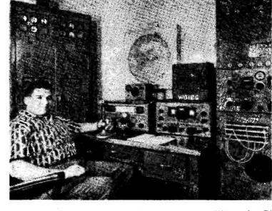
A Californian Kilowatter is W6IEG, Arcadia, Calif., who runs 1000 watts in a PA consisting of a pair of 304TL's in push-pull, with push-pull 810's modulating. Receivers are an HQ129X and a Super-Pro, and the aerial for 20 metres is a three-element wide-spaced beam.
