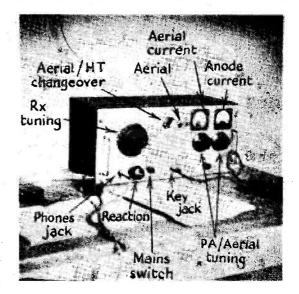
The transmitter/receiver complete, as designed and constructed by G3AHO. It is a single-valve CC oscillator, with a straight two-valve receiver, and would be particularly effective for local working on the LF bands.
