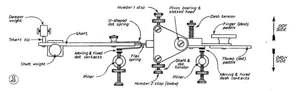
Detail sketch of a well known commercial type of semi-automatic ('' bug '') key, showing adjustments. The correct way of setting up this, and any other similar type of key, is discussed in the article.
