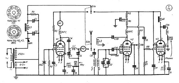
Circuit of the transmitter/receiver as used by G3AHO for CW operation on the 40-metre band. It is essentially a low-power CC transmitter (V1), with an O-V-1 receiver (V2, V3). Particularly interesting results should be possible on the LF bands, where the receiver would be more effective.
