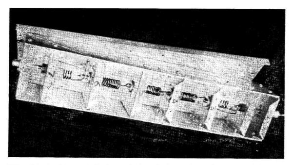
Method of construction of the complete filter shown at Fig. 15. Details of the coupling capacity used are given in the text, and constructional data for the screening box in Fig. 18.
