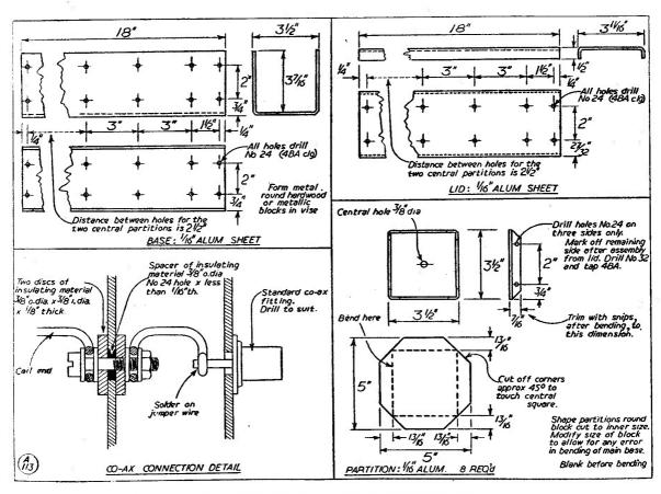
Fig. 18. Construction of the screening box for the filter shown at Fig. 15, with inter-connection details.
