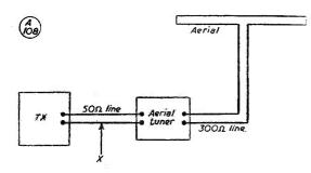
Fig. 13. Practical case in which a filter is required at point "X"
