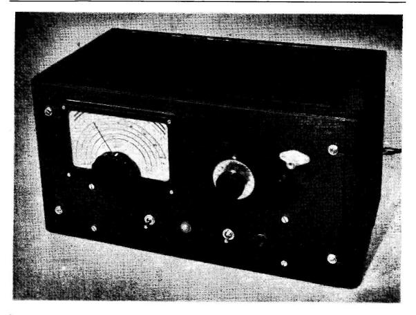
General appearance of the Crystal-Mixer VFO Unit, as designed and constructed by G5JU. Full details are given in the article, with constructional views in other photographs. An exceptionally high degree of stability is attainable with this instrument.
