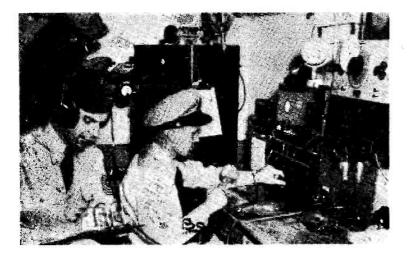
The boys at KA7RC, Iwakumi, Japan, run the full kilowatt on 14 mc, into stacked rhombics 700 feet long; the receiver is a modified AR88. The U.S. Army, Navy and Air Force are represented in the operation of this station.
