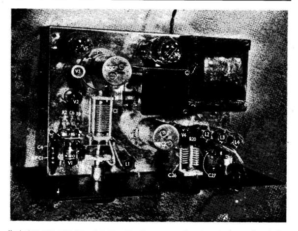
Showing layout above chassis for the Crystal-Mixer VFO, with main parts identified. The wideband couplers WBC1, WBC2 are IF transformers from the R.1124A\_SBA receiver, and involve only a very slight modification (see text) to make them suitable for this equipment.
