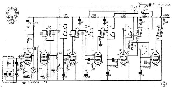
Fig. 3. The Clapp VFO, buffer amplifier and four frequency multipliers in the circuit as discussed by G3JAM in his article. By using miniature valves, a very compact band-switched assembly is possible.
