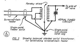
We can see, therefore, that in order to give complete protection from both electric and magnetic induction fields a combination of the coaxial and twin feeder is required. For this reason a screened twin feeder must be employed, and fortunately feeder line of this type is freely available.
