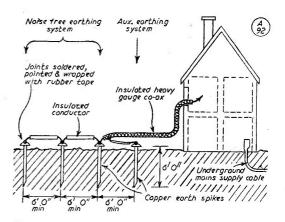
FIG to Typical installation of an ideal earthing system
