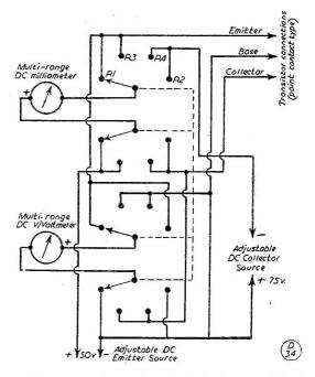
Fig. 3. A circuit derived from Fig. 2, enabling all checks to be made by switch selection. This could be built up as a standard test instrument.
