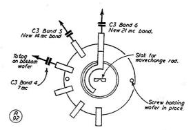
Fig. 1. The wave-change wafer switch connections, tagged to show the modifications required.
