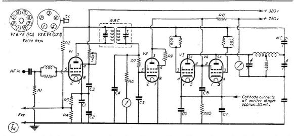
Fig. 3. Circuit of the 130-watt transmitter at VK2AWU, embodying the principles discussed in his article. The PA output can be so closely adjusted for a good keying characteristic that no thumps are audible at a nearby station tuned only a few kc off the transmission.
