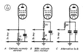
Fig. 1. Cathode keying of an early stage. Values would be R, 100-500 ohms,  $\frac{1}{2}$ w.; R1, usual cathode bias resistor; C, "break" delay condenser, .05-0.5  $\mu$ F; C1, usual RF by-pass condenser.
