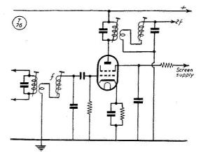
Fig. 1. Doubler stage as normally connected.
