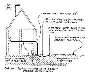
any underground electricity supply cable in relation to the main earth. The earthing system should be as far removed from this as possible, for the following reasons:
