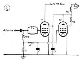
Fig. 2. Typical PA stage with screen-control valve. R is the "make" delay resistor; R1, PA grid resistor; R2, PA screen dropper; R3, 100 ohms, \( \frac{1}{2} \), "make" delay condenser; C1, PA screen by-pass condenser; V1, PA valve(s); V2, the control valve, which can be a 6L6, 6Y6G or similar
