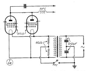
Modifications to the PT15 PA stage of the T.1154, as suggested by G2ASY. By these and the minor alterations to the driver stage as detailed in the text, he has been able to obtain a good T9 note.
