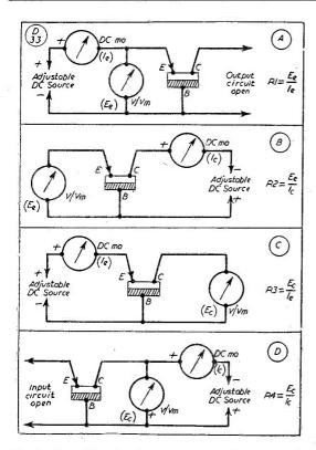
Fig. 2. Connections for the measurements discussed in the text. They enable individual transistors to be properly checked.
