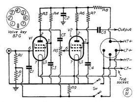
Circuit of the audio pre-amplifier, a simple enough arrangement giving reasonable gain and an absolutely hum-free output.
