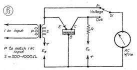
Fig. 4. The voltage amplification of a transistor can be directly checked by using the circuit shown here in the manner explained in the text.
