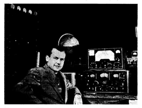
All those who heard or worked WØNWX, Newton, Iowa, during our Trans-Atlantic Tests on 160 metres earlier in the year will be particularly interested in this photograph. The gear includes a Lysco VFO driving a pair of 805's to 200 watts, and the receiver is an SX28A, modified as described in ''Short Wave Magazine '' for October, 1952. Outside, WØNWX has a 75 ft. mast supporting one end of an aerial 1,160 ft. long running across a valley.
