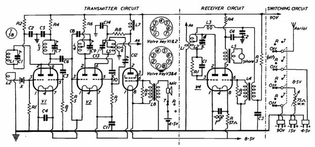
Fig. 1. Circuit complete of the short-range Handie-Talkie designed and constructed by GM6LS. The transmitter section is crystal controlled to ensure stability, but the receiver is a simple super-regenerator, since it is intended to work only with stabilised signals of high field strength. For this particular application (see photograph) it is an acceptable combination.
