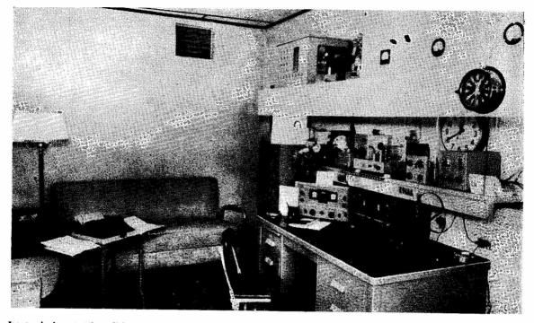
Impressive layout at the well-known DX station KV4AA, Virgin Islands. To the left on the top shelf is the 750-watt PA, using 4-125A's. Other items visible in the photograph are the beam direction indicator, VFO (centre, middle shelf), and the electronic key, to the right of the VFO. Aerials at KV4AA include a 136-ft. Zepp for 1.7, 3.5 and 7 mc and three-element beams for 14, 21 and 28 mc.
