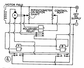
Fig. 5. Circuit arrangement for full automatic operation. In this system, the beam head cannot be turned more than 360°, since the motor is automatically reversed. The desired heading is simply set up on the direction-calibrated potentiometer, and the beam takes up its position accordingly.
