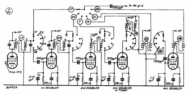
Fig. 1. Suggested circuitry, with optimum values, for the use of the wide-band couplers described in the article. Stray capacities can be equalized by the small condensers across the grid resistors.
