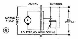
Fig. 1. Control switching, as first used at G3ION.
