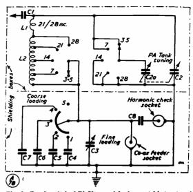
Fig. 2. Band-switched Pi-filter and feeder matching network used by G2NS during tests with the T2FD. His PA is a pair of 807's.
