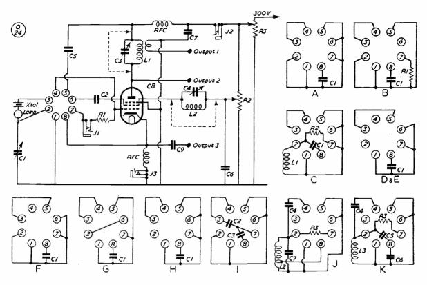
Fig. 1. Basic oscillator circuit and plug-in unit connections for selecting various oscillator arrangements. The plug reference letters identify the complete circuits they form, as shown in Fig. 2.
