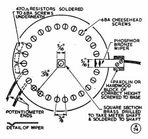
Fig. 3. Construction of the control potentiometers. It was found necessary to make these up, manufactured types not being suitable for reasons explained in the text.
