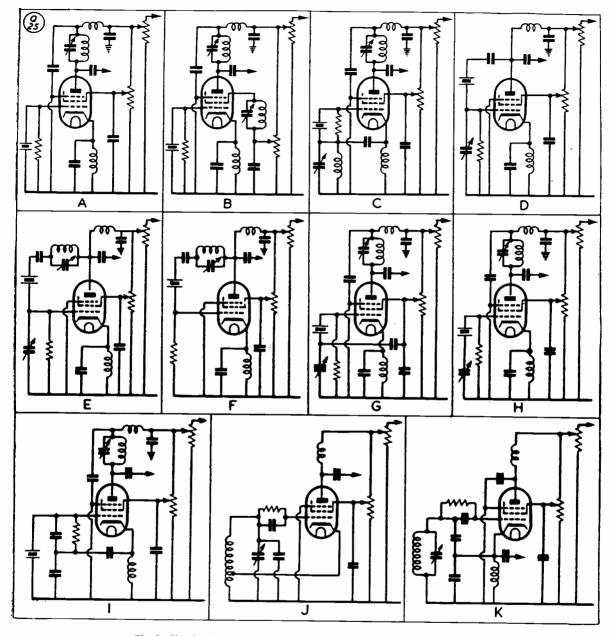
Fig. 2. Circuits derived by plugging in the adaptors wired as shown in Fig. 1.
