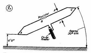
Fig. 1. The five-band T2FD aerial system, as modified by G2NS for coax feed. The dimensions and values are: AB = BC = 23 ft. 3 in. for all bands 3.5 to 28 mc; Spacing XY = 17 ins. for all bands; Tilt, 30° with low end 6 ft. above ground; Resistor, as discussed in text.
