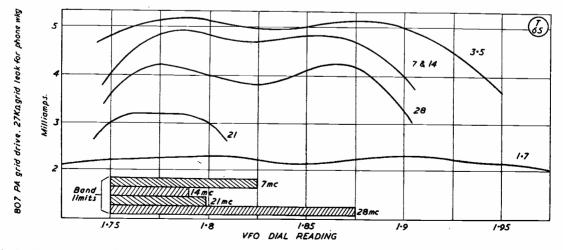
Fig. 3. These curves show frequency coverage against drive into an 807 PA for a set of wide-band couplers as designed by G3JAM and described in his article.
