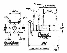
Fig. 2. This sketch shows the constructional details for the miniature wide-band couplers. Winding data are given in the Table on page 203.
