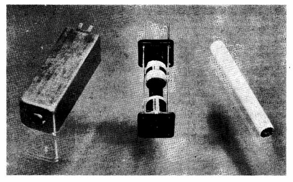
Sample of a miniature wide-band coupler designed and constructed by G3JAM, with a size comparison. The excellent flat-band characteristic of these couplers is shown in the curves at Fig. 3.
