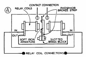
Fig. 4. Construction of a suitable polarised relay to obtain "right" and "left" rotation—see text for details.
