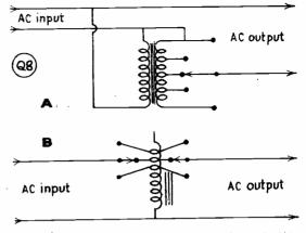
Fig. 5. Two methods of adjusting supply voltage; in (A) a small transformer would be quite adequate.
