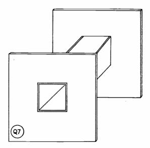
Fig. 2. Winding former for home-built power transformers. The material can be thin paxolin sheet and the laminations of Fig. 1 are built up on this core after it has been wound see text.
