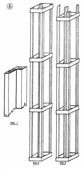
Sketches showing the construction of the tower sectionssee photographs and text for details of finalised layout.
