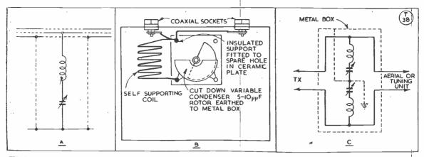
Fig. 4. Theoretical circuit (A), and practical construction (B), of a TVI filter designed to attenuate one particular harmonic with negligible effect on the fundamental output. The unit is contained in a fully-screened diecast box and the condenser is a cut-down miniature variable. A second tuned circuit (C) has to be added if the output line is of the balanced type.
