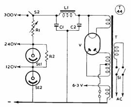
Fig. 5. Circuit diagram of a power pack suitable for the Multi-Band Exciter Unit.
