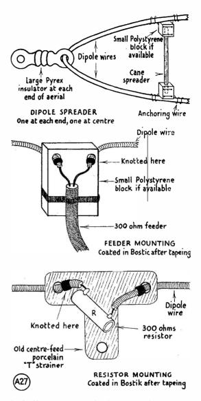
Fig. 2. Necessary constructional details for the Terminated Tilted Folded Dipole system described by G2NS.
