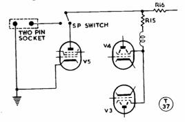
Fig. 3. When a separate Clamp modulator is used, a changeover switch and two-pin socket, wired as shown here, should be fitted to the chassis wall near V5. Only two connections are then required between modulator and transmitter, and a length of coax is ideal.
