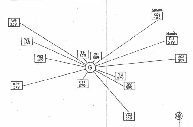
Fig. 3. Results obtained by G2NS under actual test conditions using the "T2FD" aerial described in this article. Transmission was on the 20-metre band for ten operating sessions and the directions shown here are roughly great circle paths in each case.
