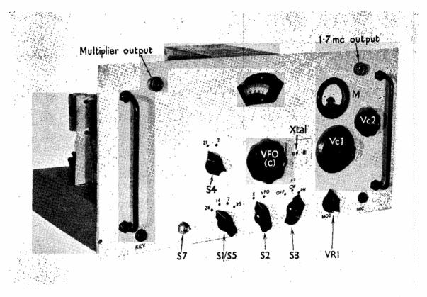
Front panel view of the Multi-Band Exciter described in the accompanying article. It gives RF drive output on all bands 1.7 to 28 mc.
