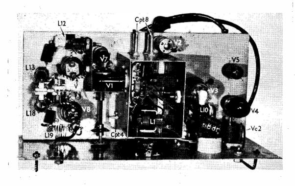
Behind-panel construction of the Exciter, showing main parts. In this view, "Cpt8" refers to padder condensers Cp5-8 (see text) and "VB" is V8 in the circuit of Fig. 4.
