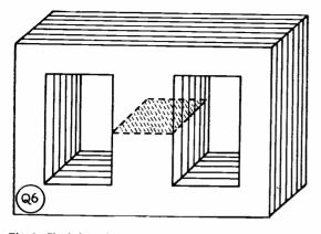
Fig. 1. Shaded portion shows cross-sectional area referred to in text. The width of the centre arm is exactly double the width of the sides, and there is no air gap.
