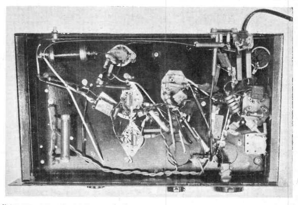
Underneath the chassis of the All-807 HF transmitter. Resistors R4 and R16, which develop some heat, are mounted well away from the oscillator stage.
