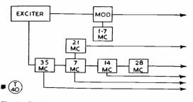
Fig. 1. Block schematic of the VFO Exciter Unit, showing electrical layout for all-band output.
