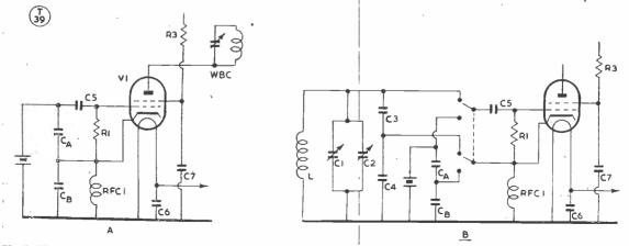
Fig. 5. The transmitter can easily be converted to crystal by changing the "front end" to correspond to (A) above. Ca is  $20 \mu\mu F a$  Cb  $40 \mu\mu F$ , other values being as in Fig. 1. Crystal or VFO control is possible by the throw of a switch if the circuit at (B) is adopted.
