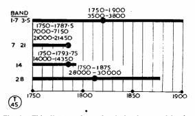
Fig. 6. This diagram shows the six bands covered by the Exciter, giving the frequency relationship, band-to-band, based on the fundamental tuning range.
