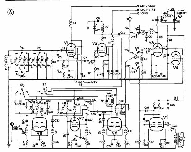
Fig. 4. Circuit of the Exciter Unit, as described and illustrated in the accompanying article.
