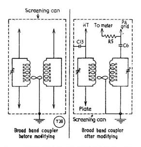
Fig. 4. Modification to the commercial broad band coupler, as mentioned in the article by VQ2AH. C6 is  $100~\mu\mu F$ ; C13, .005  $\mu F$ ; and R5 20,000 ohms.
