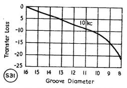
Fig. 4. Representation of losses due to what is known as Tracing Distortion, an important factor in high quality work.
