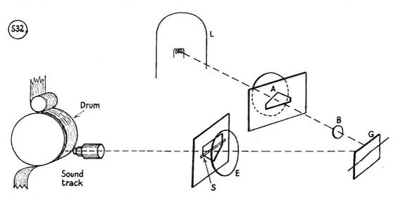
Fig. 5. Diagrammatic representation of the optical system involved in photographic sound recording. This is as for the sound-on-film technique now generally used in recording for the cinema.
