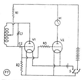
Fig. 1. Circuit of the GDO as constructed by G6FW. It is based on the original G5JU design, but is made self-contained and therefore fully portable by the use of miniature valves and battery power.
