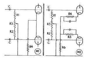
Fig. 1. No signal voltage should be present across R4 if the valves are properly balanced. R3 can be made variable to obtain balance. Fig. 2. Tests for balance are made with a headset across R6 — see text.
