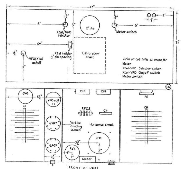
Fig. 3. Further constructional details and placing of components. This is a front-panel and top-chassis view and is not to scale.
