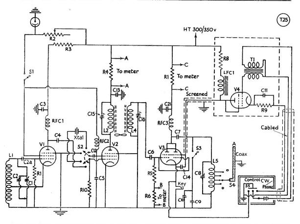
Fig. 1. Circuit complete of the 20/40 QRP Transmitter designed by VQ2AH to utilise a TU6 unit. The PA is an 832 twin tetrode operated with grid and plate sides paralleled, modulation being by screen control using a 6V6.
