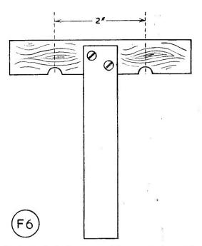
Fig. 3. The Lecher-line runner. There are, of course, other ways of making up this simple tool, depending rather upon how the wires for the Lecher are strung up.
