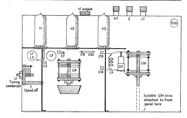
Fig. 4. Disposition of parts in G5RZ's version of the G2IQ 144 mc converter. References are to circuit elements as given in the original article—see August, 1949, issue.
