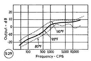
Fig. 2. Change in frequency respon se with temperature,
