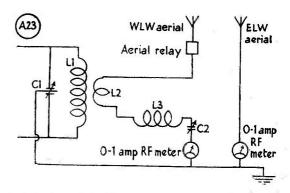
Fig. 1. Current-feed system used with 135ft. end-on wire operated as a Marconi aerial on 160 metres. Cl/Ll, balanced tank circuit; L2, coupling link; L3, loading coil, 24t. of 18g. enam. on 2 in. former; C2, .0005 µF receiving type condenser.
