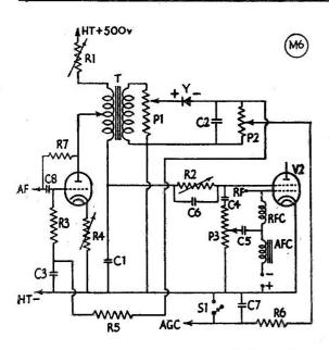
Fig. 4. The Controlled Carrier circuit as finally evolved by G3ENI and described in his article.
