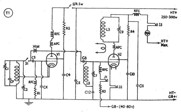
Fig. 1. Circuit of the 807 two-stage four-band transmitter suggested by G4AY. APC are aperiodic RF chokes, and the condenser from the bottom of L2 to the base line is C12, of .001 μF.
