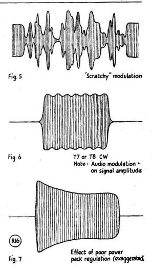
'scope at the IF output to audio detector, the point at which the BFO is also usually connected. With receiver RF gain in a normal position and BFO off, tune through the band and note the average amplitude of signals heard. Now tune to a dead spot, or disconnect aerial, and switch on BFO. Amplitude of the signal from the BFO should be approximately the same as the average of signals heard. If not adjust BFO injection until it is.
