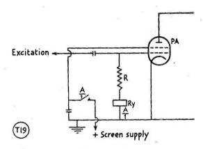
The circuit used by G5WB. The relay Ry cannot operate until drive is applied; it then switches HT to the screen of the valve. If drive fails or the grid resistor breaks down, screen HT is removed. The resistor R, with the relay resistance itself, should equal the total resistance required to give the necessary bias.
