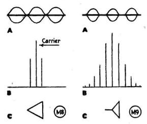
Fig. 1. Sine-wave modulation, 100%. (A) Modulation envelope; (B) Carrier and two sidebands; (C) Modulation pattern as seen on CRT. Ideally, with pure-tone modulation only two sidebands of haif carrier peak amplitude are produced.
