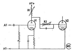
Fig. 1. Heising Constant Current Modulațion on the screengrid of a PA stage.
