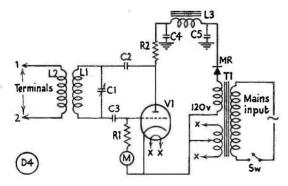
Circuit of the Test Unit described by G2YI, and incorporating its own power supply. Test capacities are connected across terminals 1, 2, and resonance readings taken off the scale of C1, which is an SLC condenser of known characteristics.
