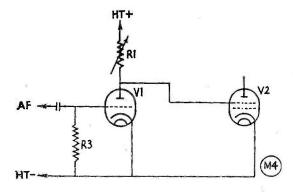
Fig. 2. Clamp Tube Modulation—which has been discussed in recent articles.
