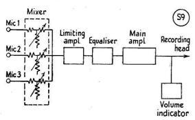
Block diagram of a typical recording system.
