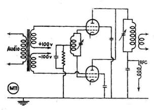
Fig. 4. Super Modulation with negative carrier, applied to the screen of the PA stage.
