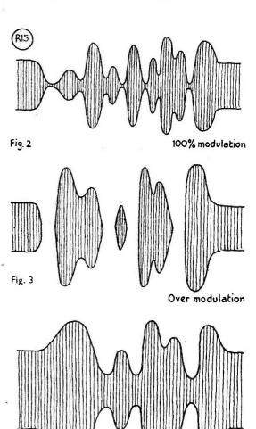
modulated signal and adjust Y-plate gain so that modulation peaks do not saturate the tube. Now increase X-plate amplifier gain until the pattern on the tube opens out to show the waveform of the modulated signal. If no X-plate amplifier is used it becomes necessary to run the time base very slowly in order to obtain the audio modulation envelope. A very slow running time base means an unsteady trace, so use of the amplifier is a distinct advantage.
