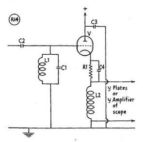
Fig. 1. Cathode follower connection for the 'scope. C2,  $20\mu\mu$ F, silver mica; C3, C4 .005  $\mu$ F; R1, as required; L1/C1, to resonate at IF, or replaceable by 100,000 ohm resistor; L2, RF choke; V, 6J5 or similar.
