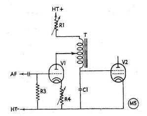
Fig. 3. An improved Clamp Tube Modulator circuit, discussed by G3ENI.
