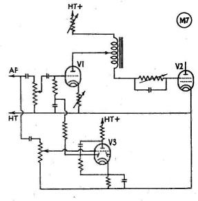
Fig. 5. Skeleton circuit of an alternative Controlled Carrier Modulator—see text.
