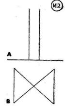
and it will be seen that the cathode ray tube modulation pattern is a symmetrical double triangle corresponding to a modulation index of infinity.
