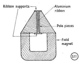
Diagrammatic representation of a ribbon microphone.
