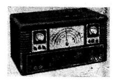
Panel appearance of the S.640 as modified by G2AIQ to incorporate the QRP Tx unit described in his article.
