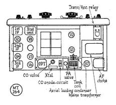
Fig. 5. General layout plan showing the positioning of the transmitter unit on the S.640 chassis. The Tx controls are brought out by flexible drive to a separate small panel mounted on the louvre on the front of the main panel of the receiver—see front view.
