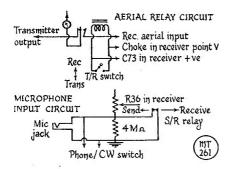
Fig. 2. Wiring detail for the Aerial Relay and Microphone Input circuits when modifying the S.640 for transmitter working.
