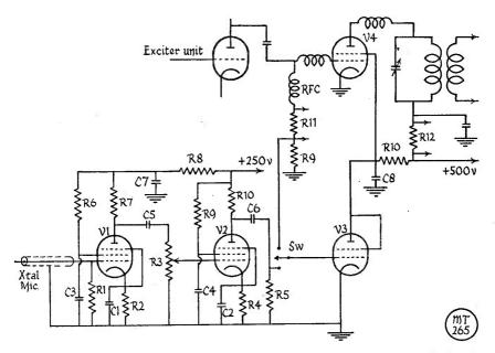
In this circuit, the Clamp valve V3 is used to modulate the screen of the PA V4 and also functions as a protective device—preventing the screen current of the PA running high when on CW. The speech circuit V1, V2 will itself provide good Clamp control of V4 under the conditions discussed in the text.
