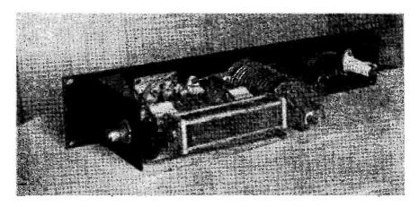
Back-panel arrangement of G2AJ's aerial coupler, the circuit of which is given in Fig. 3.
