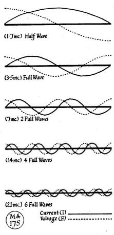
Fig. 2. Using a 270-foot aerial, this is the current-voltage distribution to be expected on five bands, neglecting end-effect. The tuning of the aerial to resonance would be effected by the coupler.
