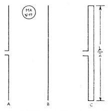
Fig. 1. Electrical layout of the folded dipole; A, the fed element and B, the driven element, are combined as C, the result being that the feedpoint impedance is stepped up, as explained in the text.
