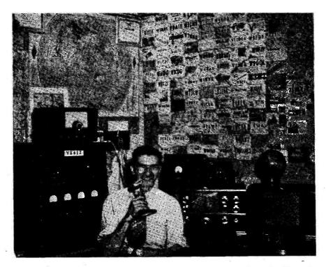
Station, operator and cards at VE6IZ, Vegreville, Alberta. The transmitter is 6C5-6L6-813 running 160 watts, modulated with a pair of 811's; the VFO is 6SK7-6AB7-6L6 with oscillator keyed for BK working; and the receiver is an NC-240D with R9'er. The whole station is relay-controlled and a fair amount of DX has been worked.
