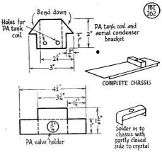
Fig. 3. The metal work and necessary mechanical details for making up the additional small fitments for the S.640 Tx unit.
