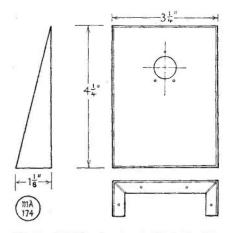
Fig. 1. Mounting bracket, in 16-gauge steel, for the aerial coupler described by G2AJ.
