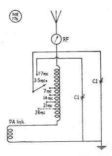
Fig. 3. Electrical arrangement of the aerial coupling unit. By using a tapped coil, all-band coverage is obtained, Cl (200 µµF) being the padder for the 1.7 mc band; C2, 150 µµF, tunes all other bands, the whole coil being in circuit for 3.5 mc operation. Unless C2 has a very low minimum capacity, it will probably not be possible to get as high as the 28 mc band. The method of linking into the PA is discussed in the text.
