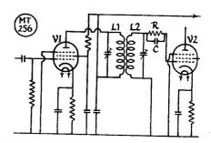
Fig. 3. An alternative circuit to that of Fig. 1, suitable for broad-band couplers used in intermediate stages. R can be 22,000 ohms and C 100  $\mu\mu$ F.
