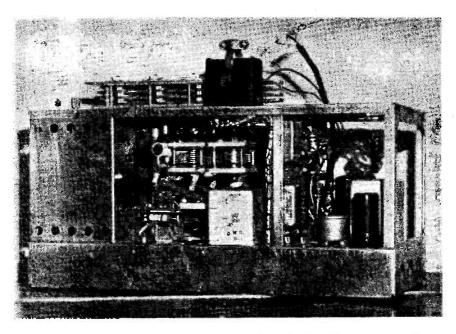
Rear view of the BC-625A, which is the transmitter section of the SCR-522, showing the additional audio stage as suggested by G2AO (see Fig. 2).
