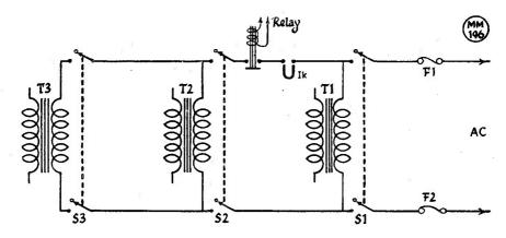
A simple switch-for-safety wiring diagram for the power supply units. Each transformer—filament, exciter HT and PA HT—is controlled through DPDT switches S1, S2 and S3, which can only be made in that order. Additional safety is ensured by the mechanical interlock Ik, while the relay can be wired for remote switching of the HT supplies from the operating position.
