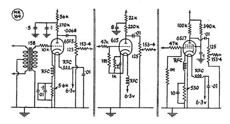
Fig. 2. Three possible methods of wiring in the additional speech amplifier, depending upon what type of microphone and 1st audio stage valve are to be used. In each case, RFC is 20 turns of No. 28 SWG enamelled wire on a 1-watt resistor as former.
