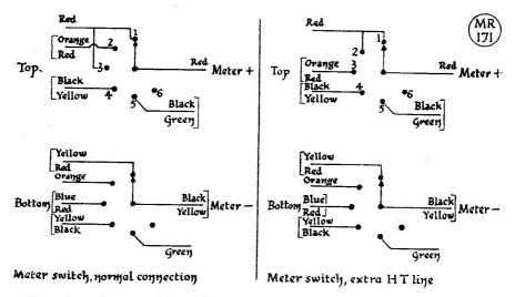
Fig. 4. The switching detail referred to in the text. The colour codings will identify the leads.
