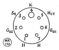
Fig. 3. Base connections of the 832 used in the BC625A.
