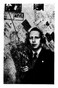
When G2BCX of South Woodford, London, goes /P on Ten, this is the outfit. It is completely self-contained and input is about ½-watt. Ranges up to a mile or so have been possible with the 1/8th wave vertical rod.
