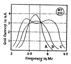
Fig. 2. These curves are of grid current against frequency in terms of band-width and show how changing the degree of coupling between L1, L2 in Fig. 1 affects the response. Taking 3.65 mc as the reference frequency, curve B indicates the correct degree of coupling for level drive conditions over the 80-metre band; in curve A the circuits are under-coupled (too "sharp") and in curve C they are too tightly coupled, giving the double-hump tuning effect.
