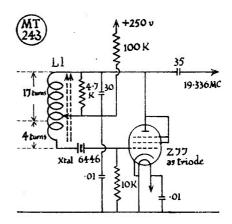
Fig. 3. It is just as necessary to choose the right frequency for the CO stage of the 2-metre converter. With an oscillator frequency of 19.336 mc, multiplied to approximately 116 mc, a tunable IF of 28-30 mc would be produced in the 2-metre receiver. In this case LI is a 3/8-in. former wound with 21 turns of 26 SWG over 1-in., tapped at the 4th turn. The coil is fitted with an adjustable dust-iron core.
